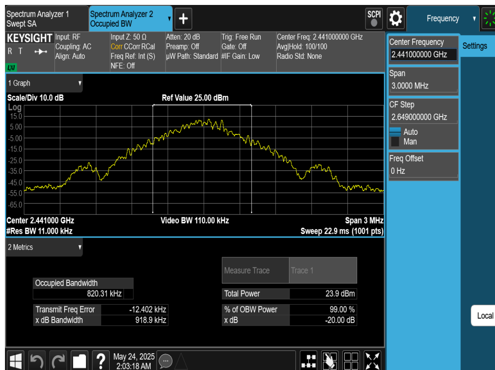
Plot 7-8. 20dB BW and 99% OBW Plot Antenna WF7 (Bluetooth, GFSK, ePA – Ch. 39)
