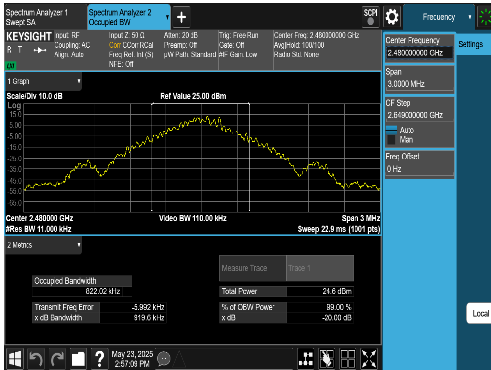
Plot 7-15. 20dB BW and 99% OBW Plot Antenna WF9 (Bluetooth, GFSK, ePA – Ch. 78)
