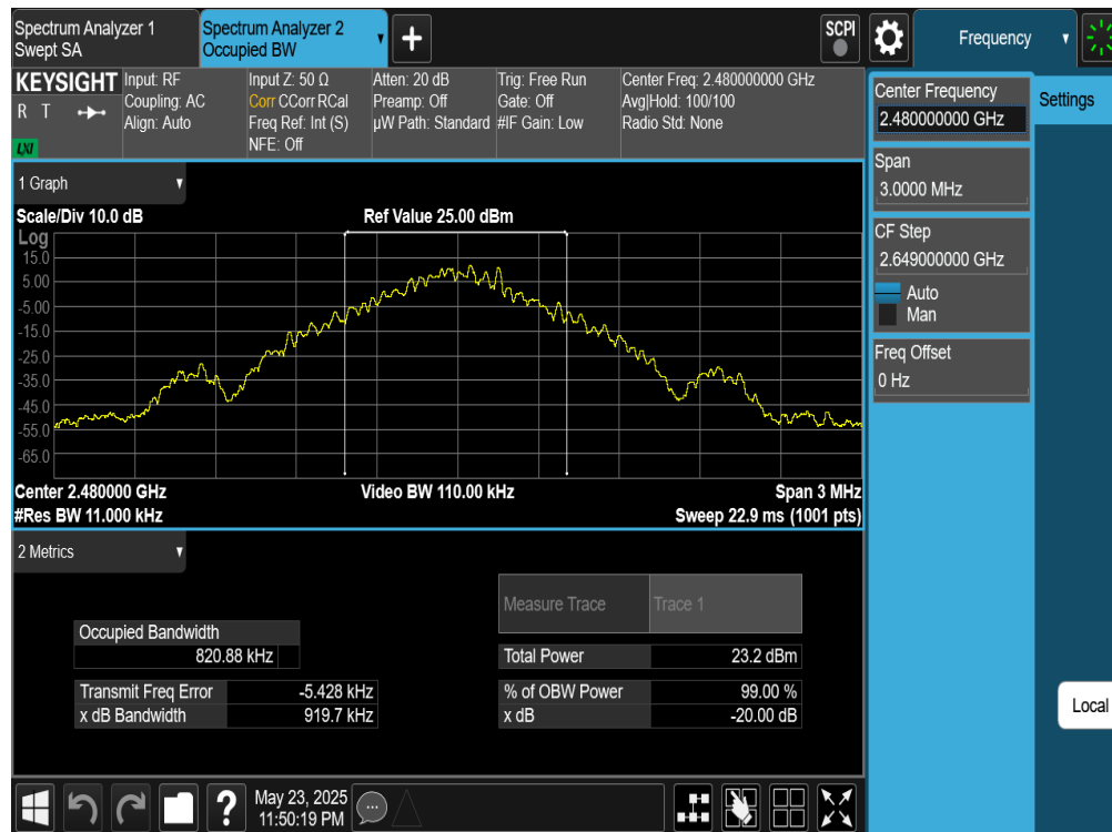
Plot 7-3. 20dB BW and 99% OBW Plot Antenna WF8 (Bluetooth, GFSK, ePA – Ch. 78)
