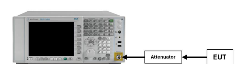
Figure 7-1. Test Instrument & Measurement Setup
