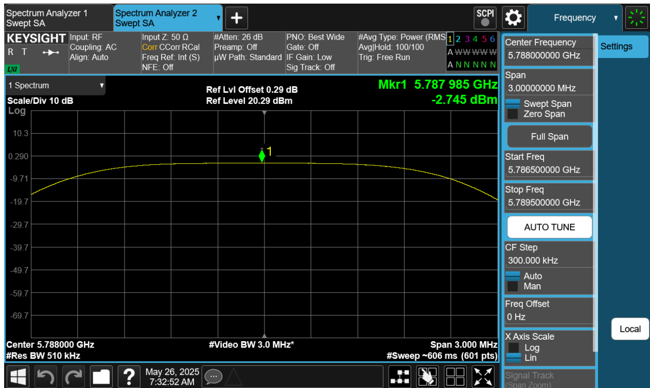
Plot 7-128. PSD Antenna WF5B (NB UNII HDT4, iPA - 5788MHz)
