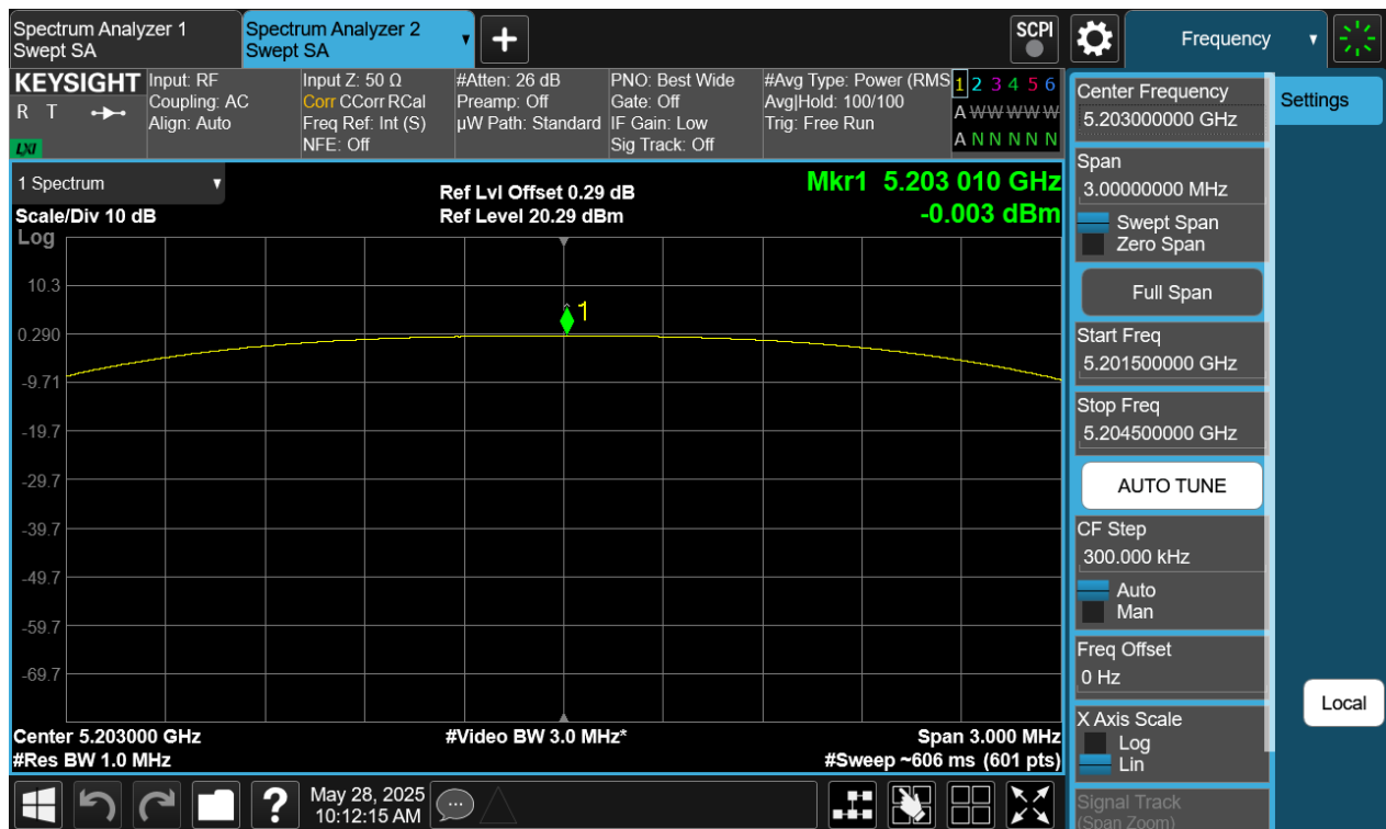
Plot 7-154. PSD Antenna WF8 (NB UNII HDT4, iPA - 5203MHz)
