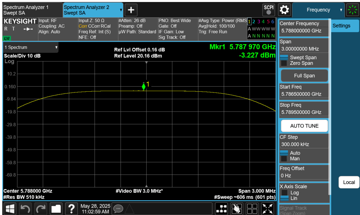
Plot 7-178. PSD Antenna WF8 (NB UNII HDT2, iPA – 5788MHz)
