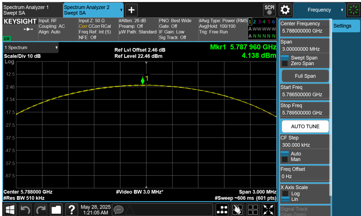
Plot 7-162. PSD Antenna WF8 (NB UNII LE2M, iPA – 5788MHz)
