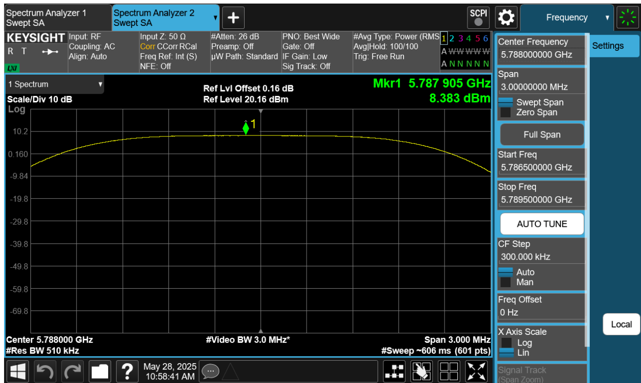
Plot 7-177. PSD Antenna WF8 (NB UNII HDT2, ePA – 5788MHz)
