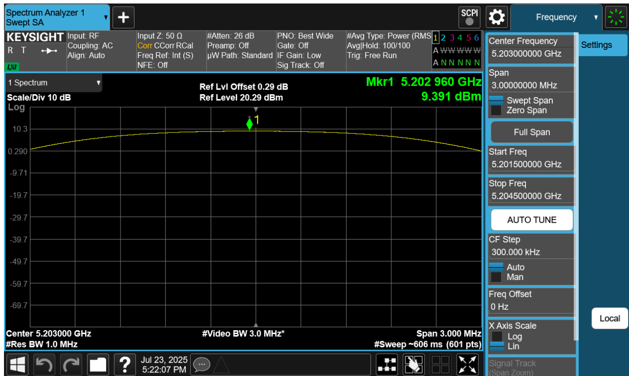
Plot 7-153. PSD Antenna WF8 (NB UNII HDT4, ePA - 5203MHz)
