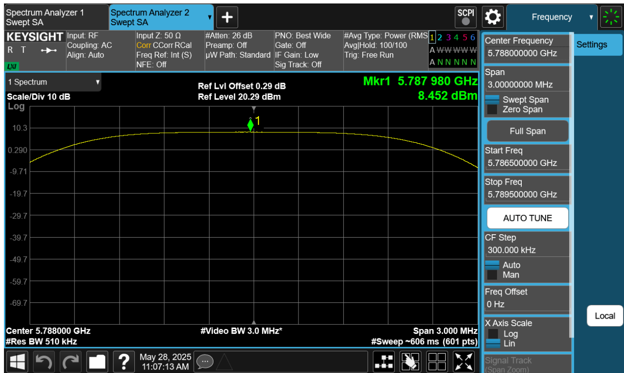
Plot 7-179. PSD Antenna WF8 (NB UNII HDT4, ePA – 5788MHz)
