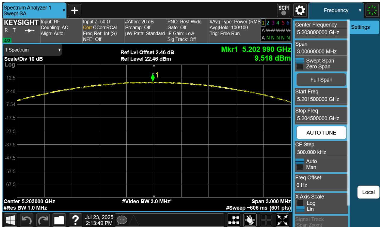
Plot 7-135. PSD Antenna WF8 (NB UNII LE2M, ePA – 5203MHz)
