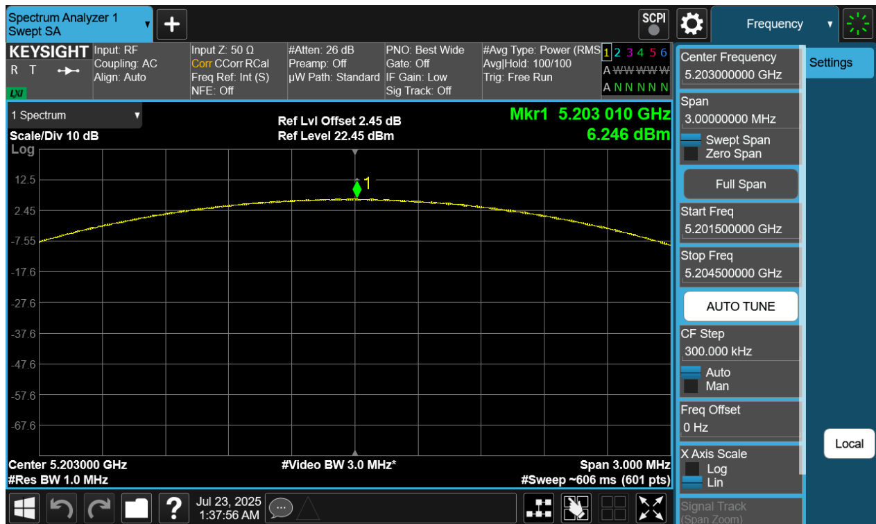
Plot 7-243. PSD Tx BF Primary Antenna WF5B (NB UNII LE2M, ePA – 5203MHz)
