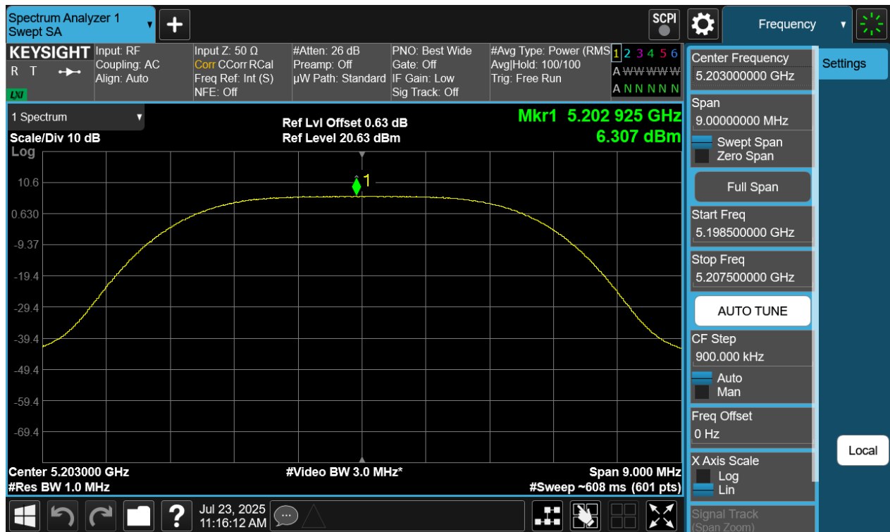
Plot 7-259. PSD Tx BF Primary Antenna WF5B (NB UNII XHDRPM6, ePA – 5203MHz)
