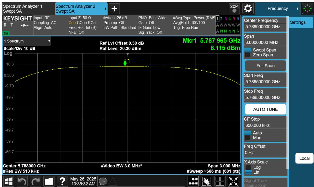
Plot 7-331. PSD Tx BF Primary Antenna WF5B (NB UNII HDT4, ePA - 5788MHz)
