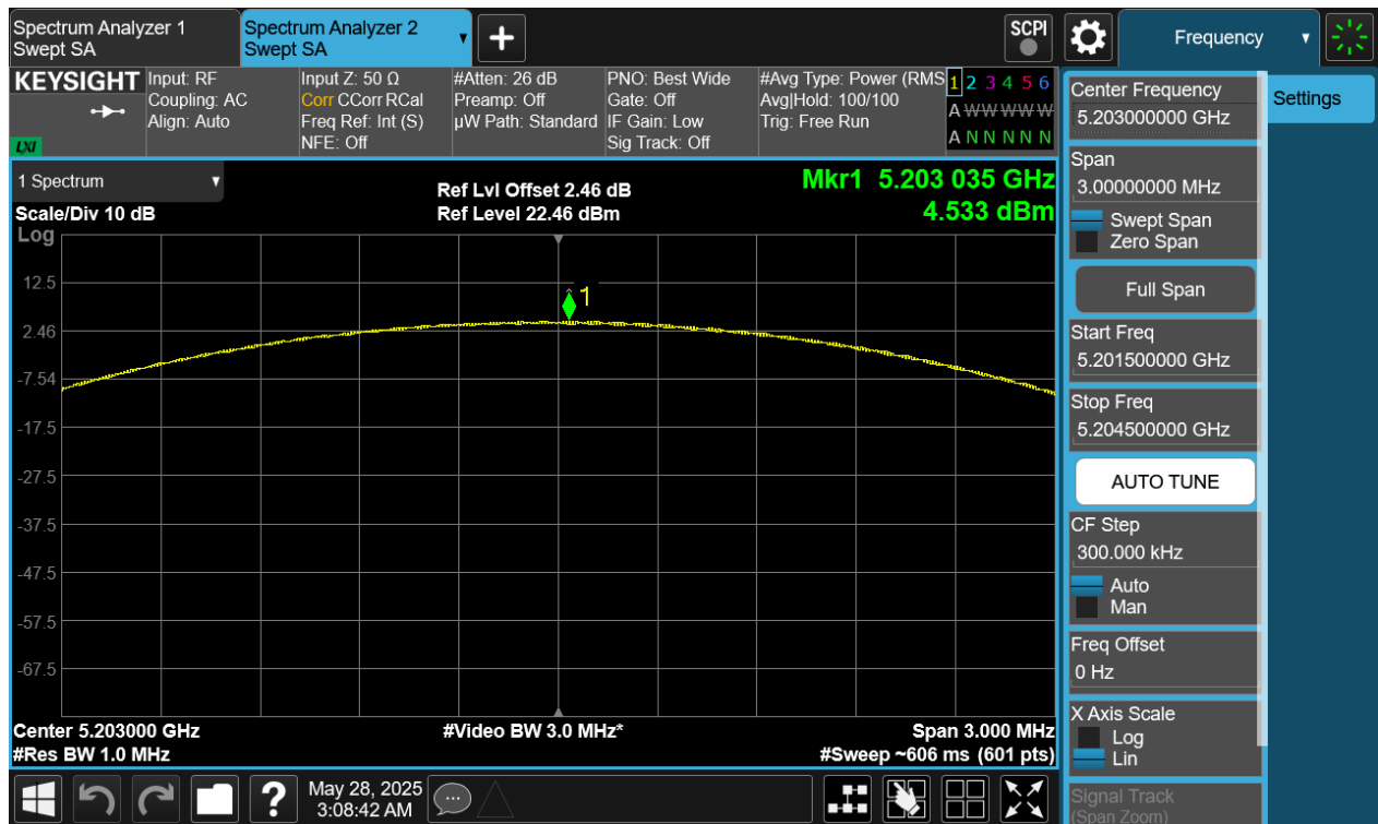
Plot 7-349. PSD TxBF Primary Antenna WF8 (NB UNII LE2M, iPA - 5203MHz)
