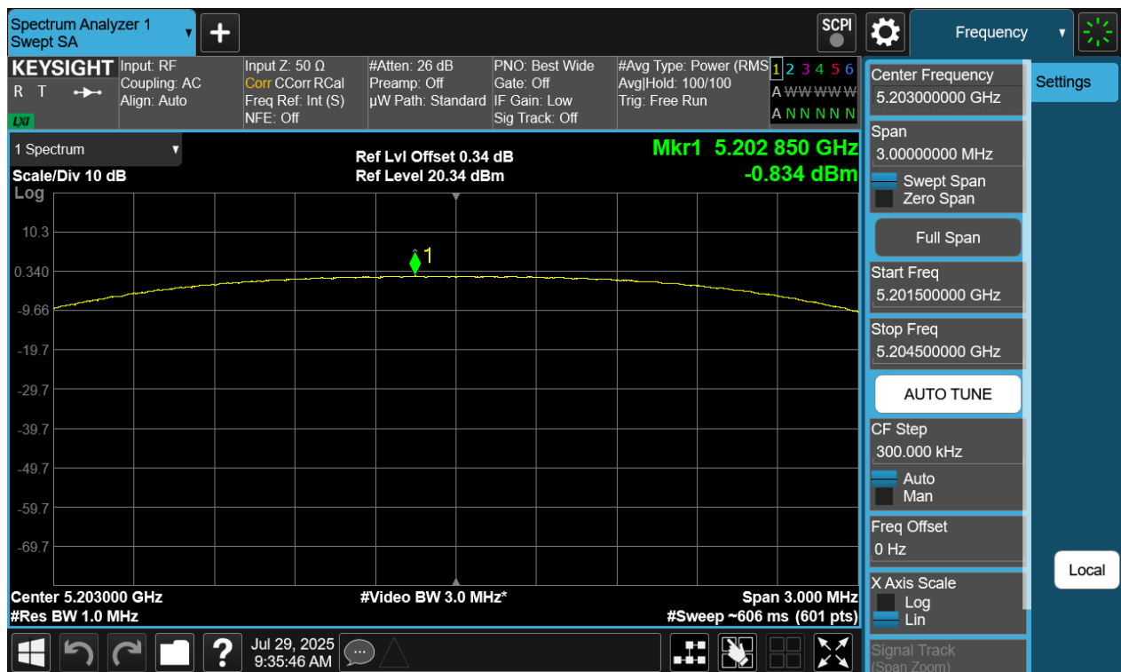
Plot 7-362. PSD TxBF Diversity Antenna WF7 (NB UNII HDRPS2, iPA – 5203MHz)
