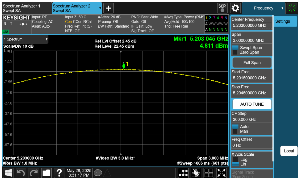
Plot 7-350. PSD TxBF Primary Antenna WF7 (NB UNII LE2M, iPA - 5203MHz)
