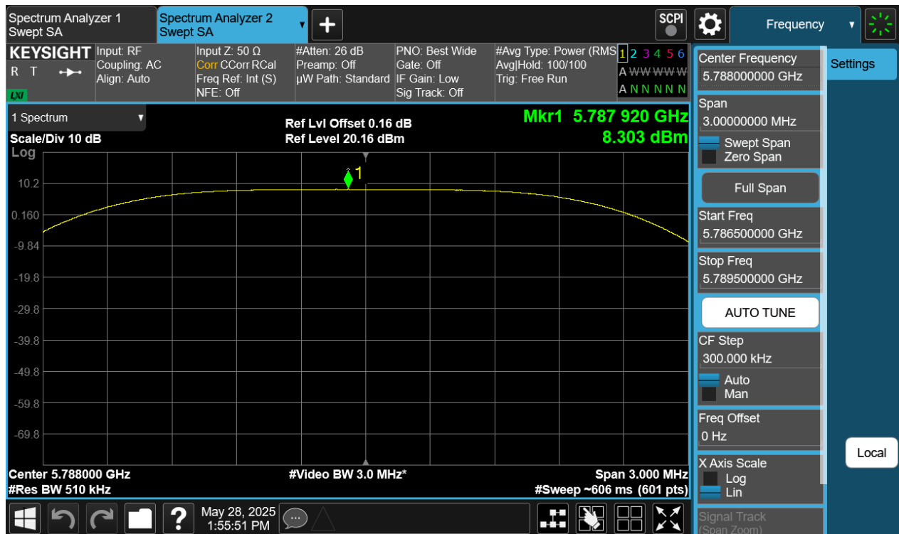
Plot 7-431. PSD Tx BF Diversity Antenna WF8 (NB UNII HDT2, ePA – 5788MHz)
