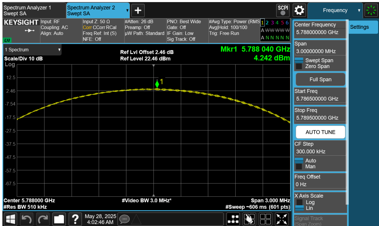
Plot 7-401. PSD TxBF Primary Antenna WF8 (NB UNII LE2M, iPA - 5788MHz)
