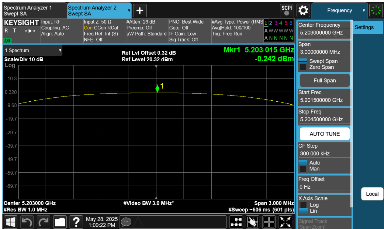
Plot 7-385. PSD Tx BF Diversity Antenna WF8 (NB UNII HDT4, iPA - 5203MHz)
