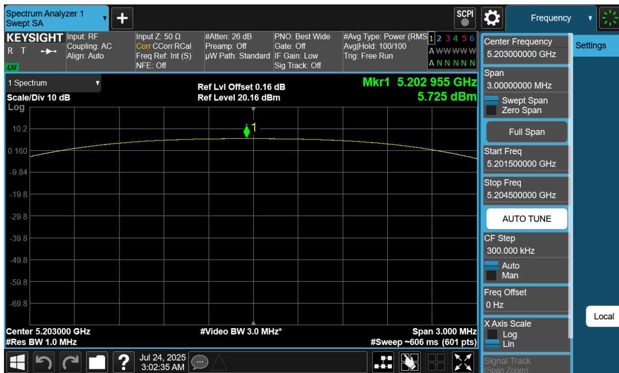
Plot 7-380. PSD Tx BF Diversity Antenna WF7 (NB UNII HDT2, ePA – 5203MHz)
