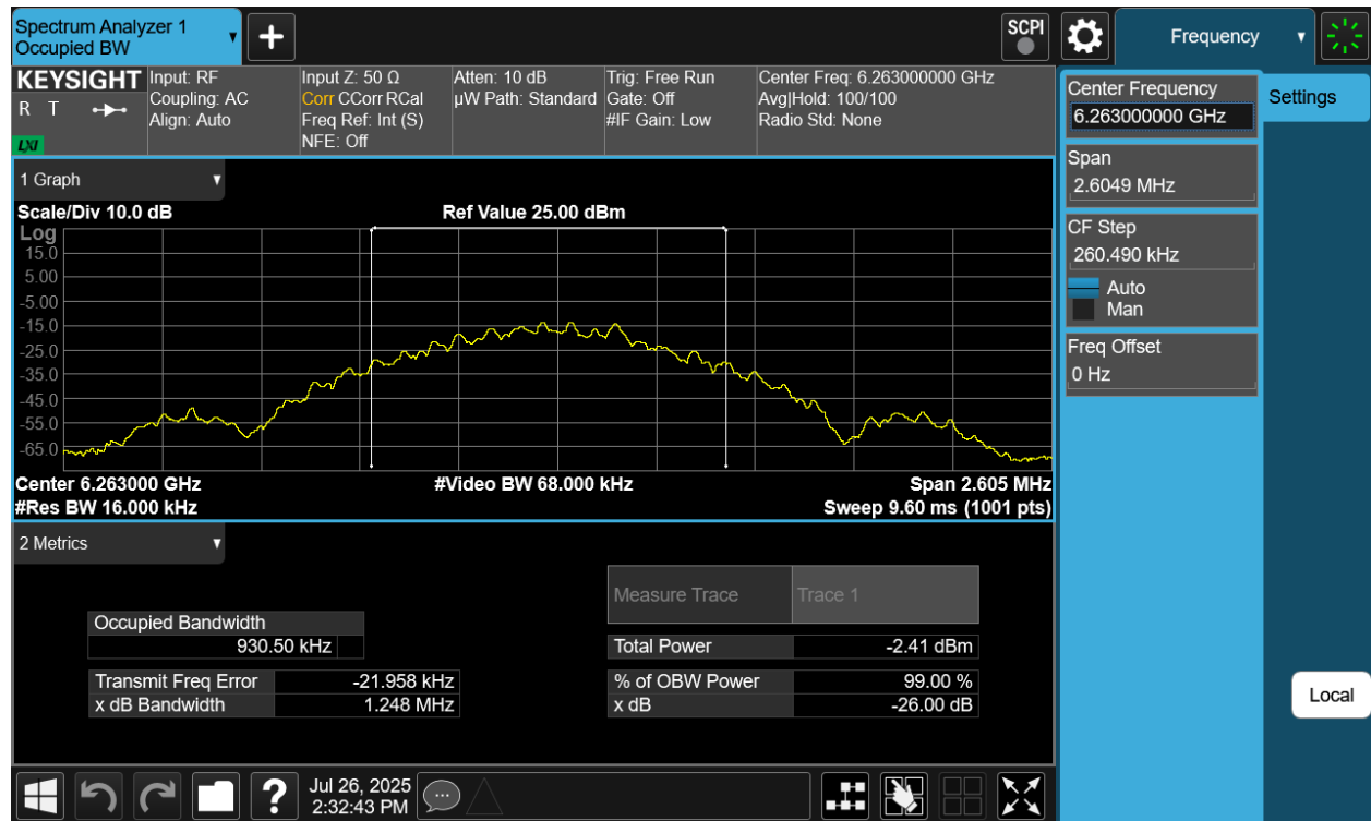
Plot 7-14. 26dB BW & 99% OBW Antenna WF8 (NB UNII BDR, ePA- 6263MHz)
