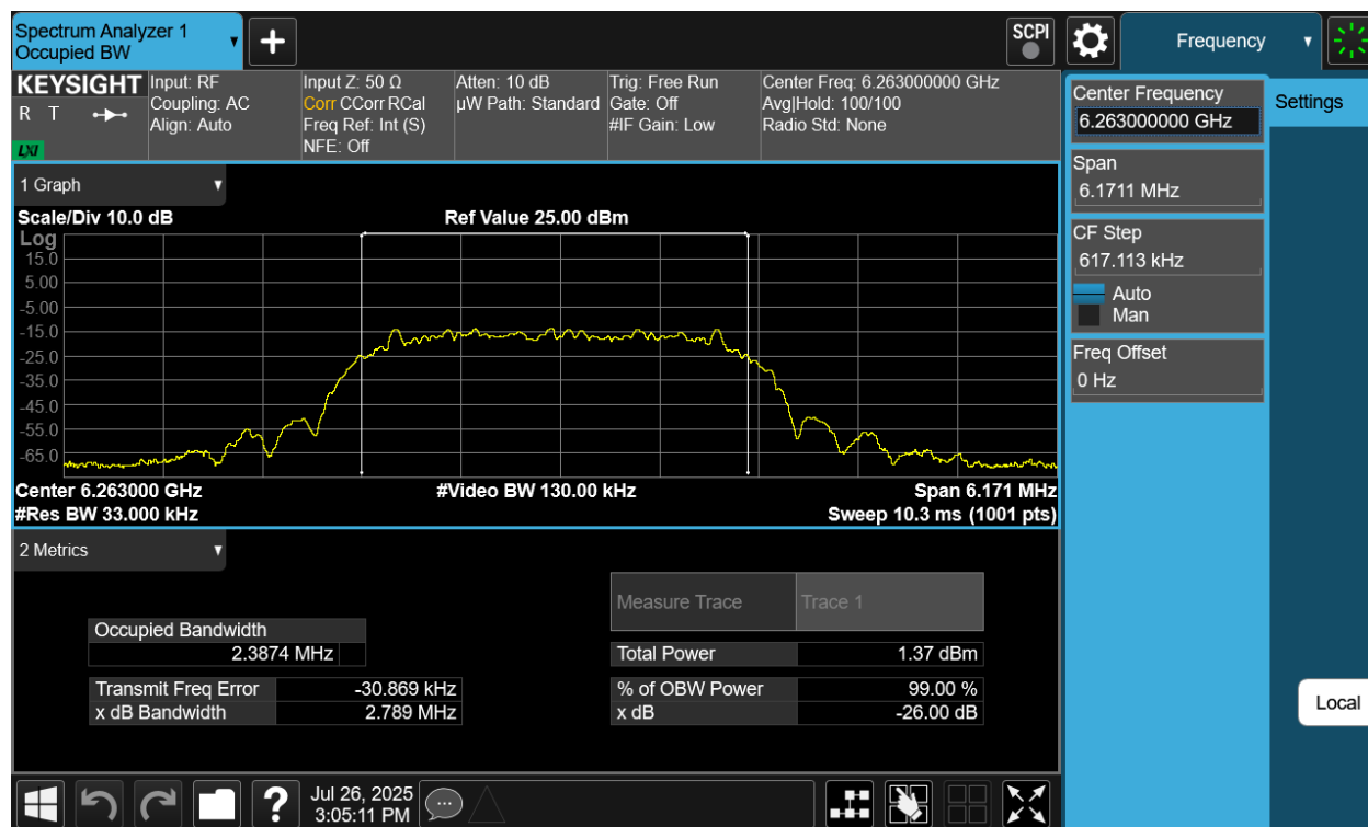
Plot 7-26. 26dB BW & 99% OBW Antenna WF8 (NB UNII HDT6, ePA– 6263MHz)
