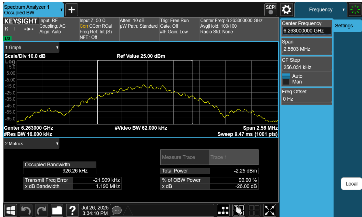
Plot 7-27. 26dB BW & 99% OBW Antenna WF7 (NB UNII BDR, ePA- 6263MHz)
