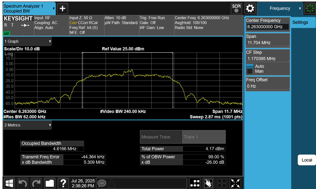
Plot 7-18. 26dB BW & 99% OBW Antenna WF8 (NB UNII HDR8, ePA- 6263MHz)
