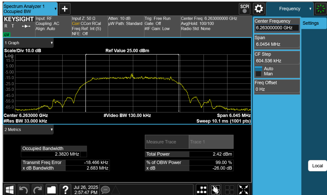
Plot 7-19. 26dB BW & 99% OBW Antenna WF8 (NB UNII HDRPS2, ePA- 6263MHz)
