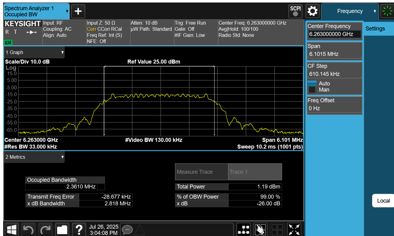
Plot 7-25. 26dB BW & 99% OBW Antenna WF8 (NB UNII HDT4, ePA- 6263MHz)
