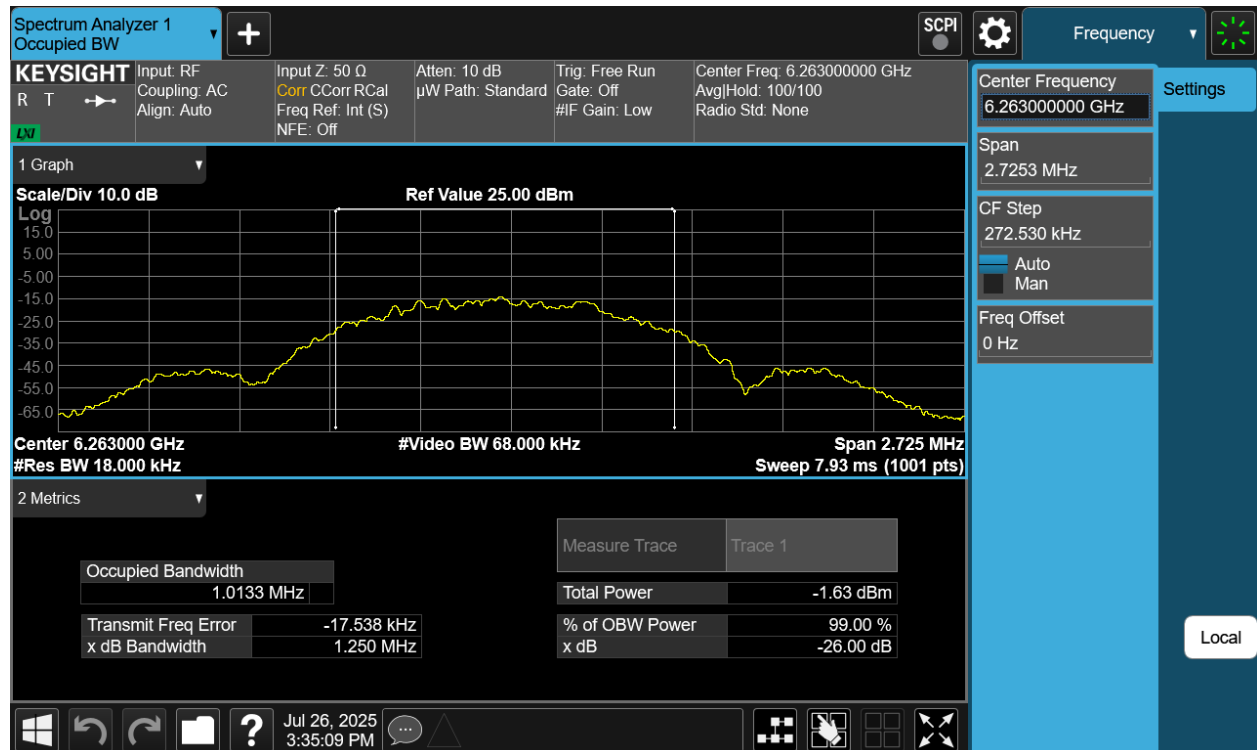
Plot 7-28. 26dB BW & 99% OBW Antenna WF7 (NB UNII LE1M, ePA- 6263MHz)
