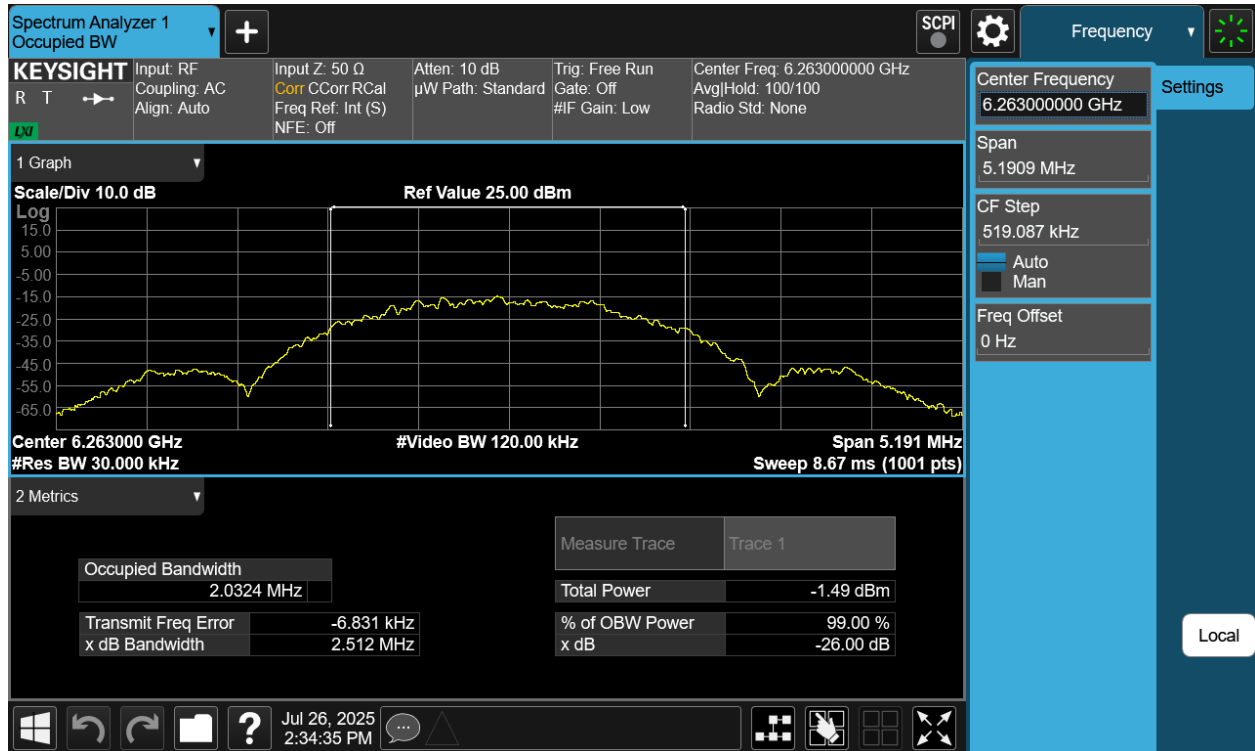
Plot 7-16. 26dB BW & 99% OBW Antenna WF8 (NB UNII LE2M, ePA- 6263MHz)
