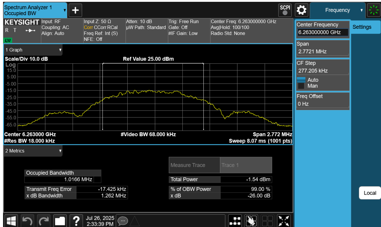
Plot 7-15. 26dB BW & 99% OBW Antenna WF8 (NB UNII LE1M, ePA- 6263MHz)
