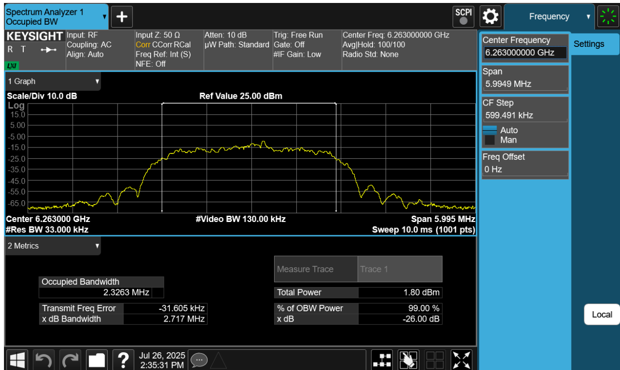
Plot 7-17. 26dB BW & 99% OBW Antenna WF8 (NB UNII HDR4, ePA- 6263MHz)
