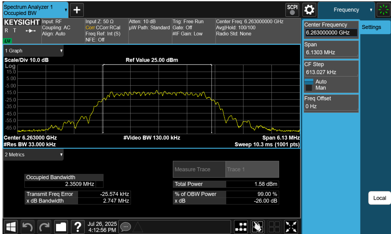
Plot 7-37. 26dB BW & 99% OBW Antenna WF7 (NB UNII HDT2, ePA- 6263MHz)
