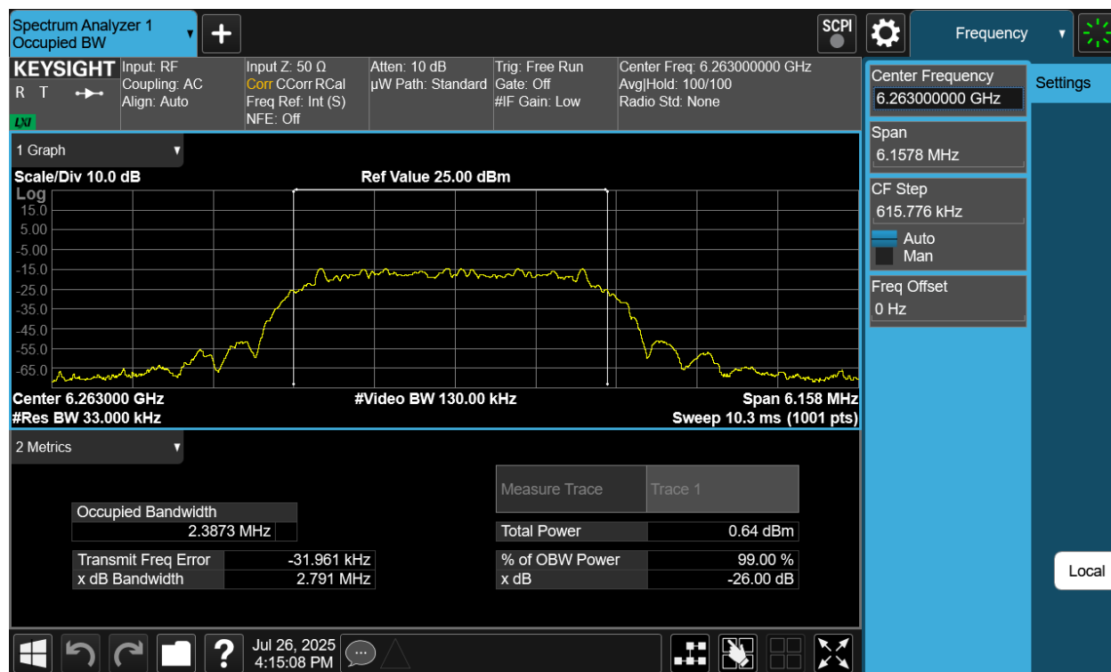
Plot 7-39. 26dB BW & 99% OBW Antenna WF7 (NB UNII HDT6, ePA– 6263MHz)
