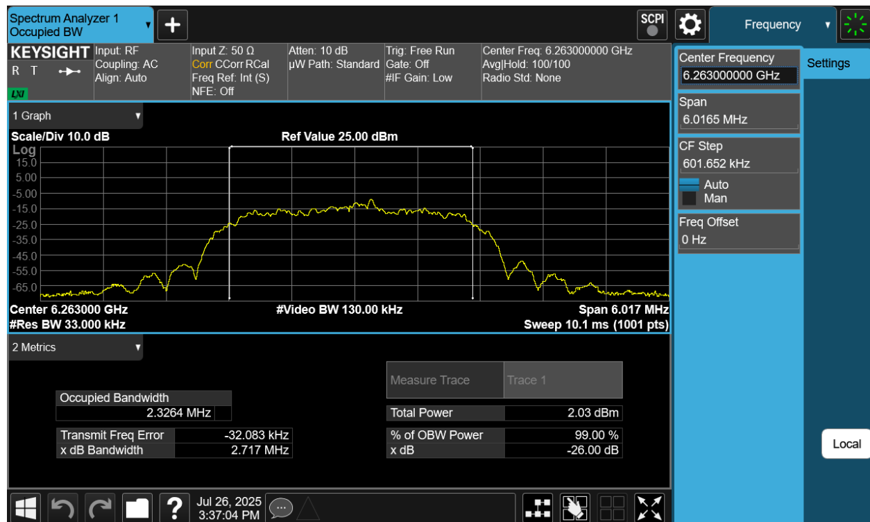
Plot 7-30. 26dB BW & 99% OBW Antenna WF7 (NB UNII HDR4, ePA- 6263MHz)
