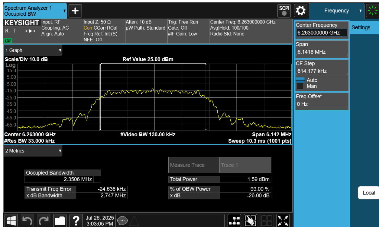
Plot 7-24. 26dB BW & 99% OBW Antenna WF8 (NB UNII HDT2, ePA- 6263MHz)
