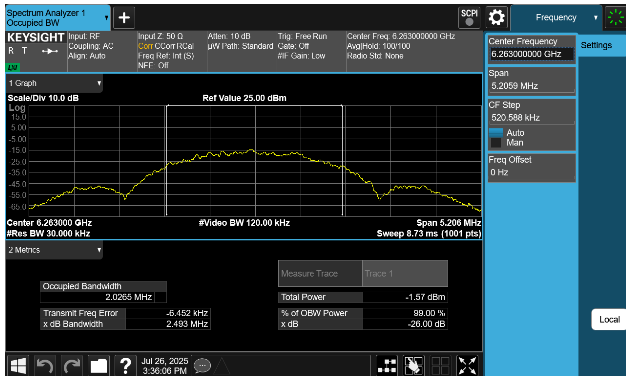
Plot 7-29. 26dB BW & 99% OBW Antenna WF7 (NB UNII LE2M, ePA- 6263MHz)
