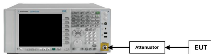
Figure 7-3. Test Instrument & Measurement Setup
