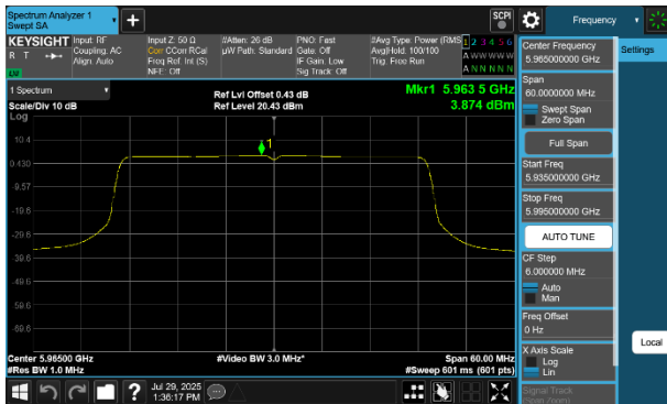
Plot 7-170 PSD CDD Primary Antenna WF5B (40MHz BW 802.11be(SU) - Ch.3)
