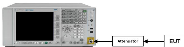
Figure 7-4. Test Instrument & Measurement Setup
