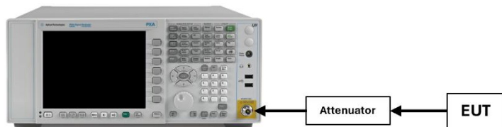
Figure 7-4. Test Instrument & Measurement Setup
