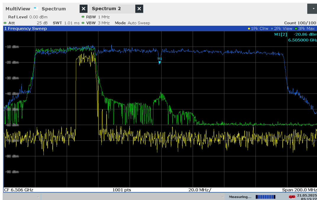
Plot 7-306. 160MHz Bandwidth, AWGN Signal Injected – 6505MHz
