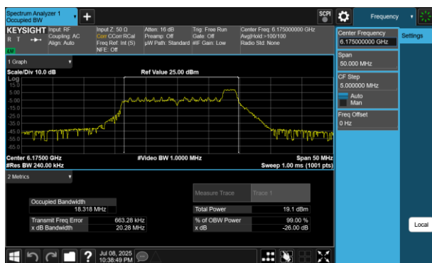
Plot 7-1 26dB BW & 99% OBW Antenna WF5B (20MHz BW 802.11be(RU) RU26 Index8 - Ch.45)
