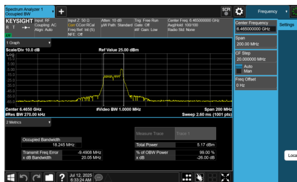
Plot 7-47 26dB BW & 99% OBW Antenna WF5B (80MHz BW 802.11be(RU) RU26 Index17 - Ch.103)
