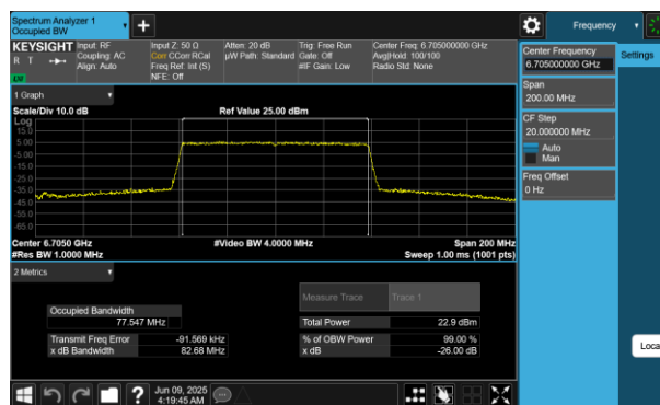
Plot 7-65 26dB BW & 99% OBW Antenna WF5B (80MHz BW 802.11be(RU) RU996 Index67 - Ch.151)
