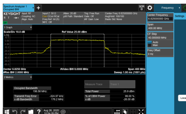
Plot 7-66 26dB BW & 99% OBW Antenna WF5B (160MHz BW 802.11be(RU) RU996X2 Index68 - Ch.175)
