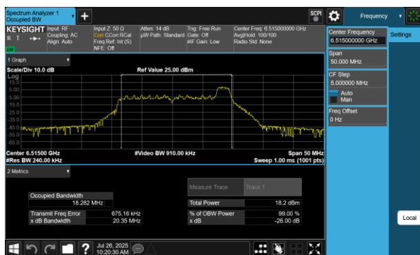
Plot 7-12 26dB BW & 99% OBW Antenna WF5B (20MHz BW 802.11be(RU) RU26 Index8 - Ch.113)
