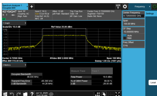
Plot 7-64 26dB BW & 99% OBW Antenna WF5B (40MHz BW 802.11be(RU) RU484 Index65 - Ch.155)
