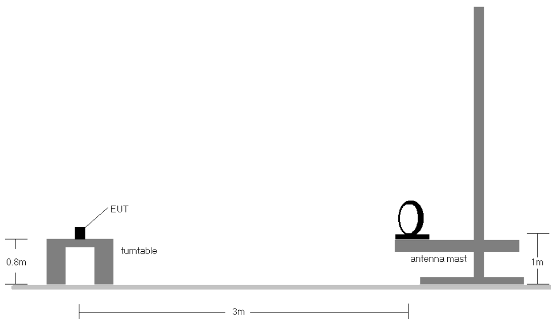
Figure 7-6. Radiated Test Setup < 30MHz
