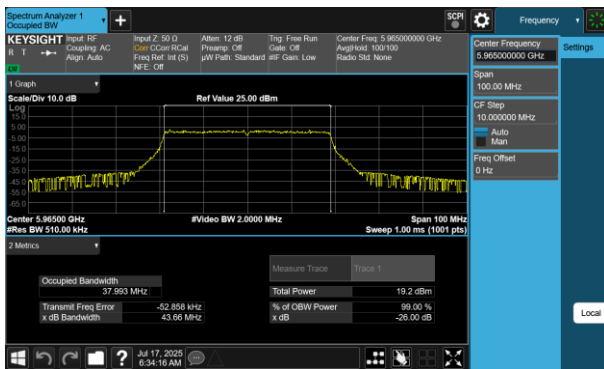
Plot 7-196 26dB BW & 99% OBW Antenna WF7 (40MHz BW 802.11be(RU) RU484 Index65 - Ch.3)
