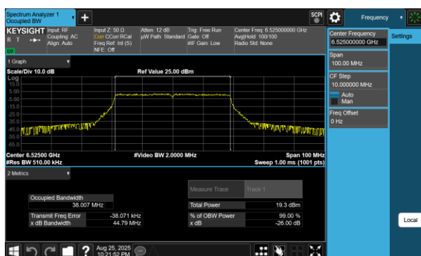
Plot 7-207 26dB BW & 99% OBW Antenna WF7 (40MHz BW 802.11be(RU) RU484 Index65 - Ch.115)
