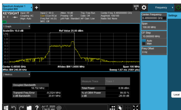
Plot 7-200 26dB BW & 99% OBW Antenna WF7 (40MHz BW 802.11be(RU) RU26 Index8 - Ch.107)
