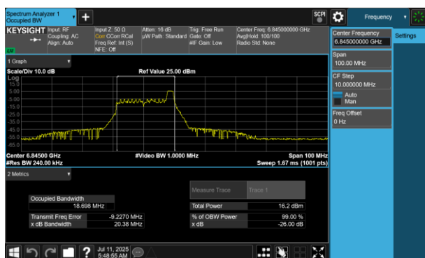
Plot 7-178 26dB BW & 99% OBW Antenna WF7 (40MHz BW 802.11be(RU) RU26 Index8 - Ch.179)
