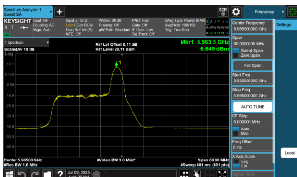
Plot 7-233 PSD Antenna WF5B (40MHz BW 802.11be(RU) RU26 Index8 - Ch.3)
