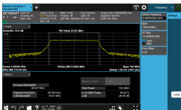
Plot 7-229 26dB BW & 99% OBW Antenna WF7 (40MHz BW 802.11be(RU) RU484 Index65 - Ch.187)
