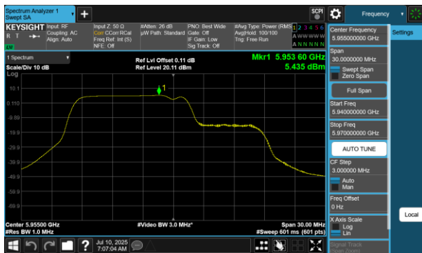
Plot 7-236 PSD Antenna WF5B (20MHz BW 802.11be(RU) RU106+26 Index82 - Ch.1)
