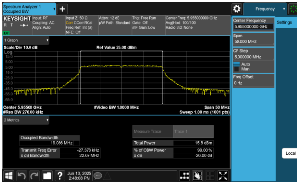
Plot 7-195 26dB BW & 99% OBW Antenna WF7 (20MHz BW 802.11be(RU) RU242 Index61 - Ch.1)
