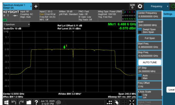
Plot 7-198 PSD Antenna WF8 (160MHz BW 802.11be(RU) RU996X2 Index68 - Ch.111)
