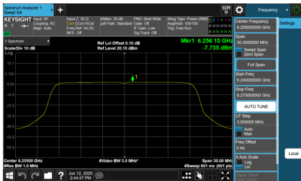
Plot 7-184 PSD Antenna WF8 (20MHz BW 802.11be(RU) RU242 Index61 - Ch.61)
