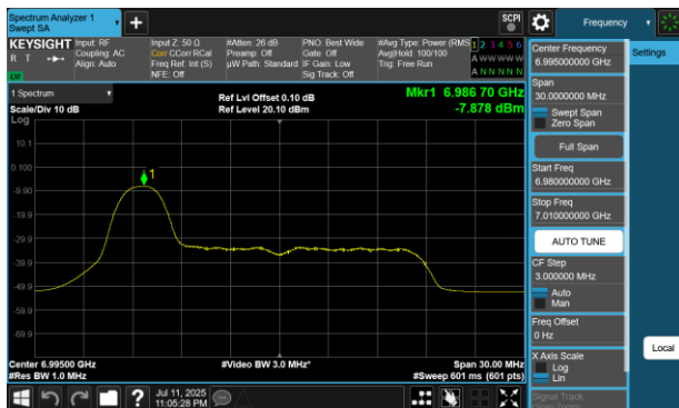
Plot 7-166 PSD Antenna WF5B (20MHz BW 802.11be(RU) RU26 Index0 - Ch.209)
