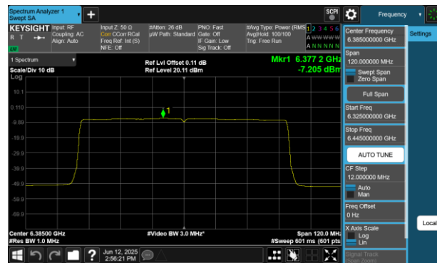
Plot 7-186 PSD Antenna WF8 (80MHz BW 802.11be(RU) RU996 Index67 - Ch.87)
