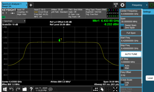
Plot 7-151 PSD Antenna WF5B (20MHz BW 802.11be(RU) RU242 Index61 - Ch.97)
