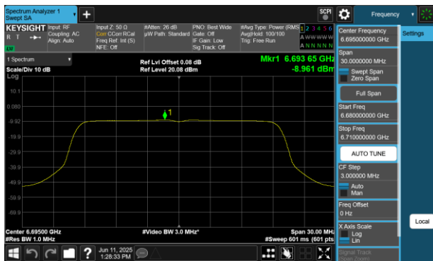
Plot 7-162 PSD Antenna WF5B (20MHz BW 802.11be(RU) RU242 Index61 - Ch.149)
