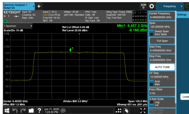
Plot 7-153 PSD Antenna WF5B (80MHz BW 802.11be(RU) RU996 Index67 - Ch.103)
