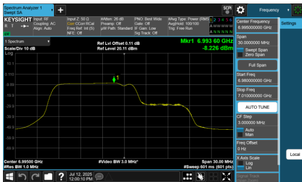
Plot 7-170 PSD Antenna WF5B (20MHz BW 802.11be(RU) RU106+26 Index82 - Ch.209)
