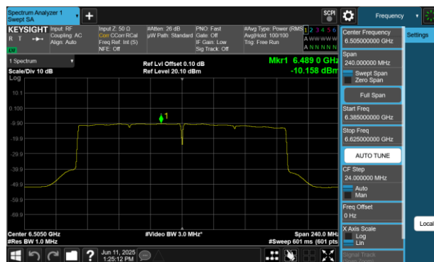
Plot 7-154 PSD Antenna WF5B (160MHz BW 802.11be(RU) RU996X2 Index68 - Ch.111)
