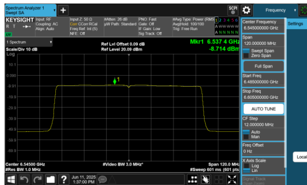
Plot 7-164 PSD Antenna WF5B (80MHz BW 802.11be(RU) RU996 Index67 - Ch.119)
