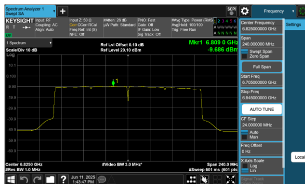
Plot 7-165 PSD Antenna WF5B (160MHz BW 802.11be(RU) RU996X2 Index68 - Ch.175)
