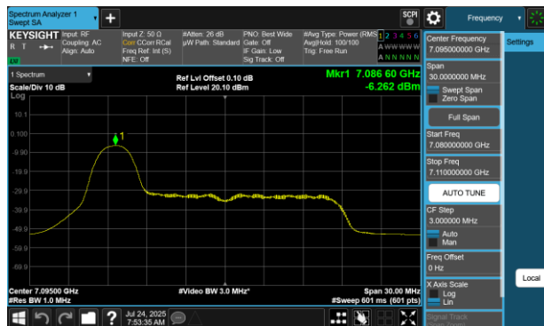
Plot 7-210 PSD Antenna WF8 (20MHz BW 802.11be(RU) RU26 Index0 - Ch.229)
