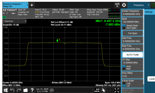
Plot 7-197 PSD Antenna WF8 (80Mhz BW 802.11be(RU) RU996 Index67 - Ch.103)
