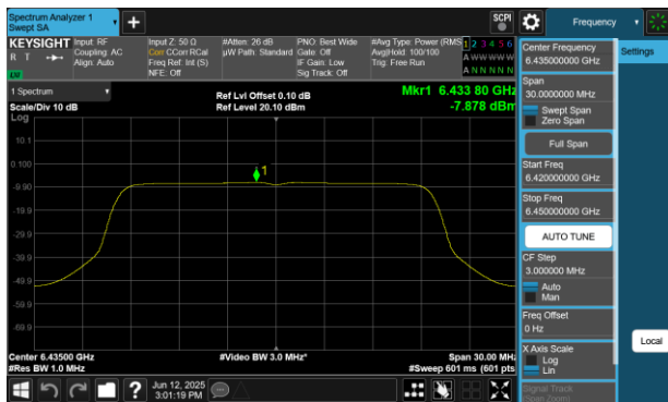
Plot 7-195 PSD Antenna WF8 (20MHz BW 802.11be(RU) RU242 Index61 - Ch.97)
