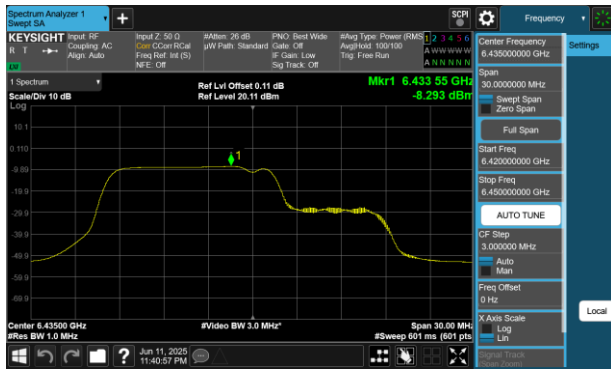
Plot 7-148 PSD Antenna WF5B (20MHz BW 802.11be(RU) RU106+26 Index82 - Ch.97)
