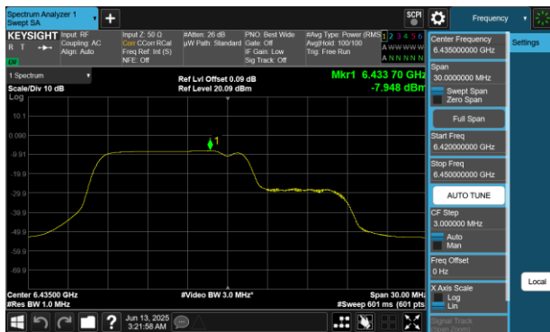
Plot 7-192 PSD Antenna WF8 (20MHz BW 802.11be(RU) RU106+26 Index82 - Ch.97)
