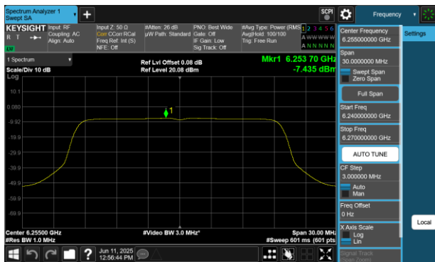
Plot 7-140 PSD Antenna WF5B (20MHz BW 802.11be(RU) RU242 Index61 - Ch.61)
