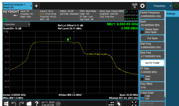
Plot 7-412 PSD Antenna WF7 (20MHz BW 802.11be(RU) RU106+26 Index82 - Ch.149)
