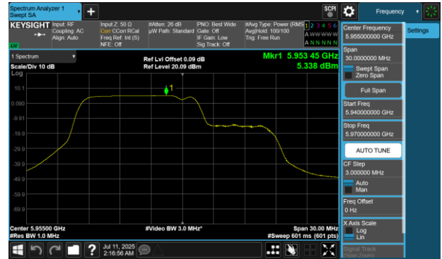
Plot 7-474 PSD CDD Primary Antenna WF8 (20MHz BW 802.11be(RU) RU106+26 Index82 - Ch.1)
