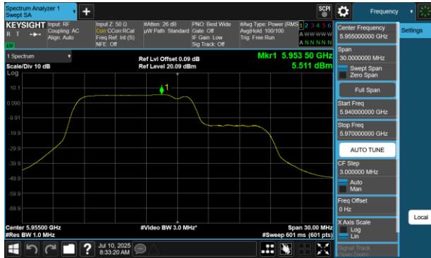
Plot 7-471 PSD CDD Primary Antenna WF5B (20MHz BW 802.11be(RU) RU106+26 Index82 - Ch.1)
