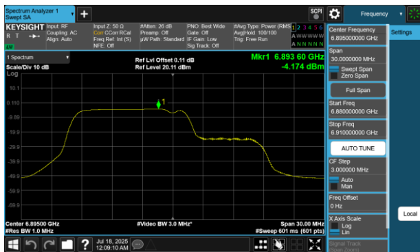
Plot 7-456 PSD Antenna WF7 (20MHz BW 802.11be(RU) RU106+26 Index82 - Ch.189)
