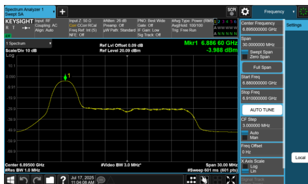
Plot 7-452 PSD Antenna WF7 (20MHz BW 802.11be(RU) RU26 Index0 - Ch.189)
