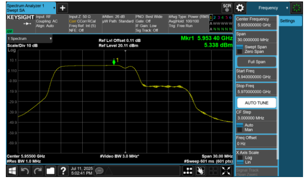
Plot 7-628 PSD CDD Diversity Antenna WF7 (20MHz BW 802.11be(RU) RU106+26 Index82 - Ch.1)
