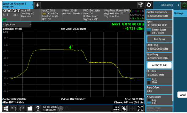
Plot 7-581 PSD SDM Primary Antenna WF5B (20MHz BW 802.11be(RU) RU106+26 Index82 - Ch.185)
