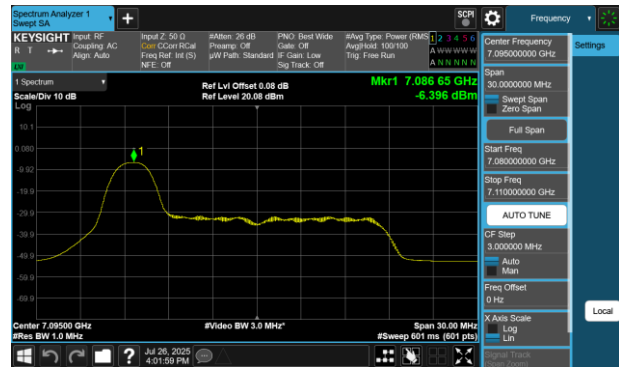
Plot 7-599 PSD SDM Primary Antenna WF8 (20MHz BW 802.11be(RU) RU26 Index0 - Ch.229)
