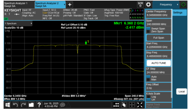
Plot 7-638 PSD CDD Diversity Antenna WF7 (160MHz BW 802.11be(RU) RU996X2 Index68 - Ch.79)
