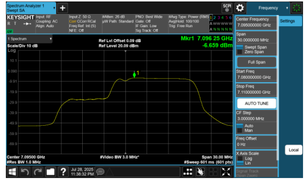
Plot 7-606 PSD SDM Primary Antenna WF8 (20MHz BW 802.11be(RU) RU106+26 Index83 - Ch.229)
