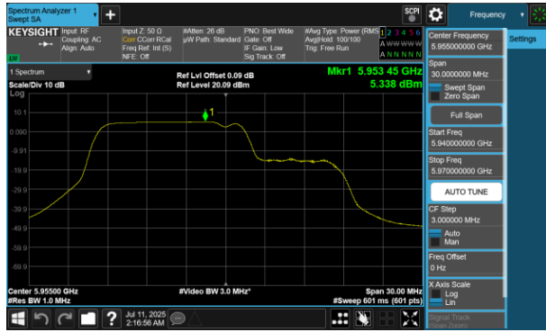
Plot 7-625 PSD CDD Diversity Antenna WF8 (20MHz BW 802.11be(RU) RU106+26 Index82 - Ch.1)
