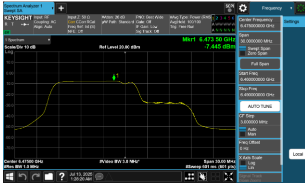
Plot 7-559 PSD SDM Primary Antenna WF5B (20MHz BW 802.11be(RU) RU106+26 Index82 - Ch.105)
