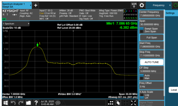
Plot 7-595 PSD SDM Primary Antenna WF5B (20MHz BW 802.11be(RU) RU26 Index0 - Ch.229)
