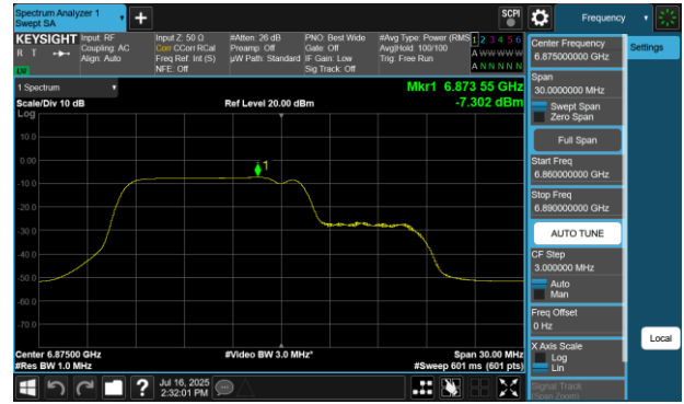
Plot 7-584 PSD SDM Primary Antenna WF8 (20MHz BW 802.11be(RU) RU106+26 Index82 - Ch.185)
