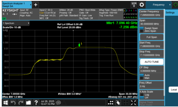
Plot 7-603 PSD SDM Primary Antenna WF5B (20MHz BW 802.11be(RU) RU106+26 Index83 - Ch.229)
