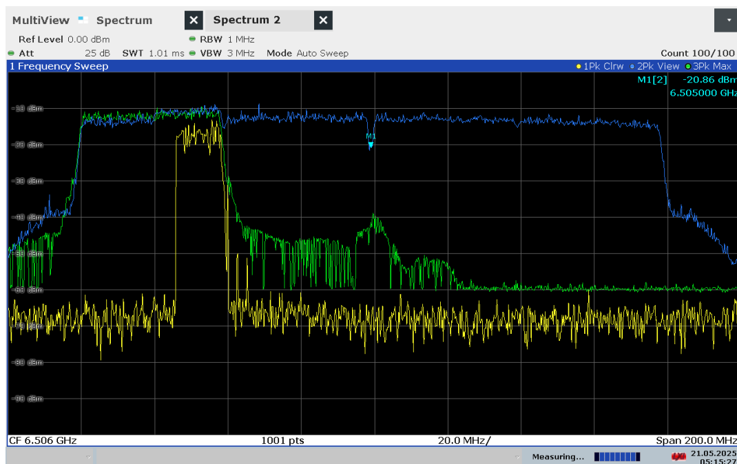
Plot 7-782. 160MHz Bandwidth, AWGN Signal Injected – 6505MHz
