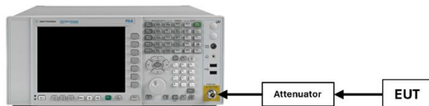
Figure 7-1. Test Instrument & Measurement Setup
