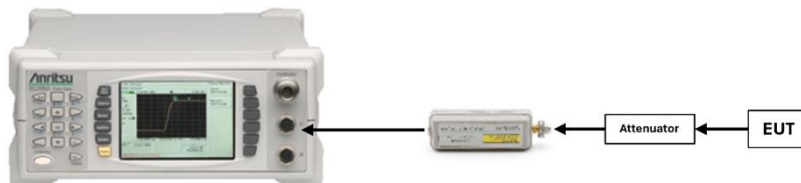
Figure 7-3. Test Instrument & Measurement Setup
