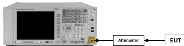
Figure 7-2. Test Instrument & Measurement Setup
