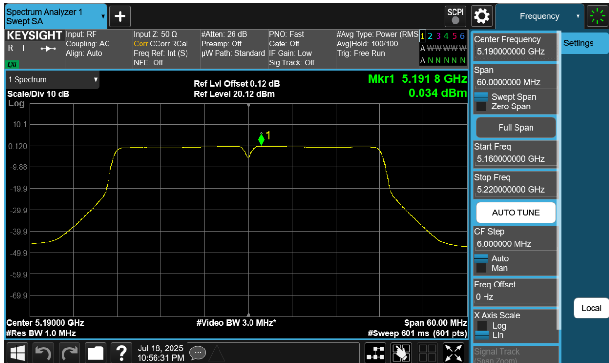
Plot 7-96 PSD CDD Diversity Antenna WF7 (40MHz BW 802.11n - Ch.38)
