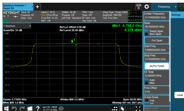
Plot 7-66 PSD Antenna WF5B (40MHz BW 802.11be(RU) RU484 Index65 - Ch.142)
