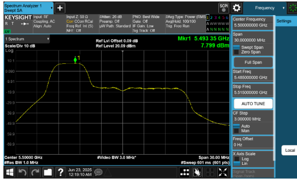
Plot 7-58 PSD Antenna WF5B (20MHz BW 802.11be(RU) RU52 Index37 - Ch.100)
