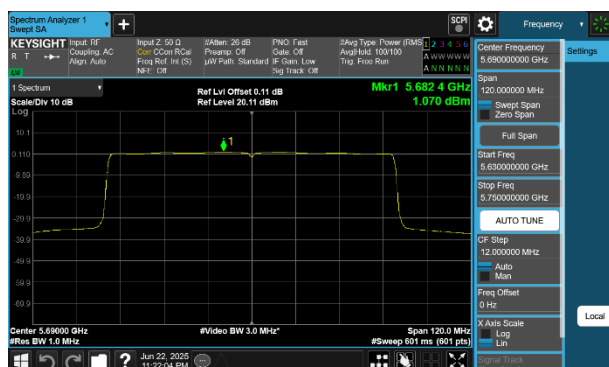
Plot 7-67 PSD Antenna WF5B (80MHz BW 802.11be(RU) RU996 Index67 - Ch.138)
