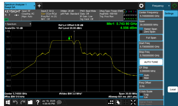
Plot 7-176 PSD CDD Primary Antenna WF8 (20MHz BW 802.11be(RU) RU52+26 Index71 - Ch.149)
