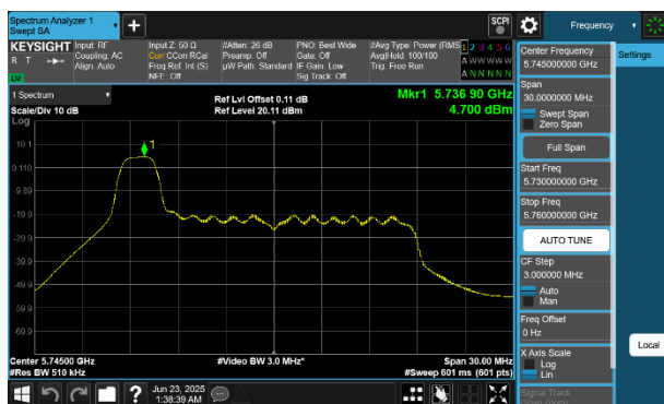
Plot 7-173 PSD CDD Primary Antenna WF5B (20MHz BW 802.11be(RU) RU26 Index0 - Ch.149)
