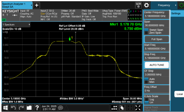
Plot 7-156 PSD CDD Primary Antenna WF8 (20MHz BW 802.11be(RU) RU52+26 Index71 - Ch.36)
