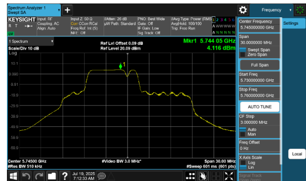
Plot 7-236 PSD CDD Diversity Antenna WF7 (20MHz BW 802.1be(RU) RU52+26 Index71 - Ch.149)
