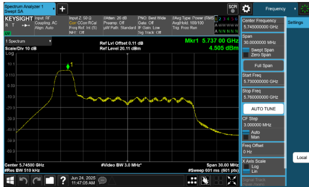
Plot 7-230 PSD CDD Diversity Antenna WF7 (20MHz BW 802.1be(RU) RU26 Index0 - Ch.149)
