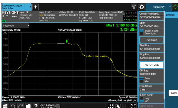
Plot 7-197 PSD SDM Primary Antenna WF5B (20MHz BW 802.11be(RU) RU106+26 Index82 - Ch.40)
