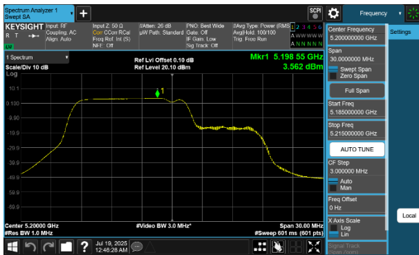
Plot 7-194 PSD SDM Primary Antenna WF8 (20MHz BW 802.11be(RU) RU106+26 Index82 - Ch.40)
