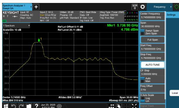
Plot 7-233 PSD CDD Diversity Antenna WF8 (20MHz BW 802.1be(RU) RU26 Index0 - Ch.149)
