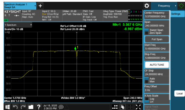
Plot 7-229 PSD CDD Diversity Antenna WF8 (160MHz BW 802.11be(RU) RU996X2 Index68 - Ch.114)
