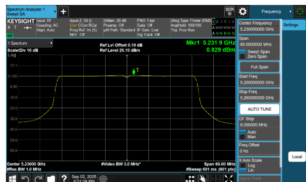
Plot 7-201 PSD SDM Primary Antenna WF8 (40MHz BW 802.11be(RU) RU484 Index65 - Ch.46)
