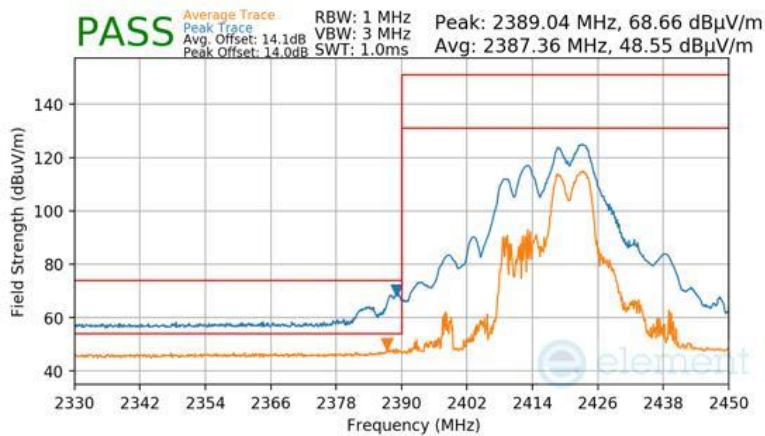
Plot 7-324 Radiated Restricted Lower Band Edge Measurement CDD Diversity (Peak & Average – RU52+26)
