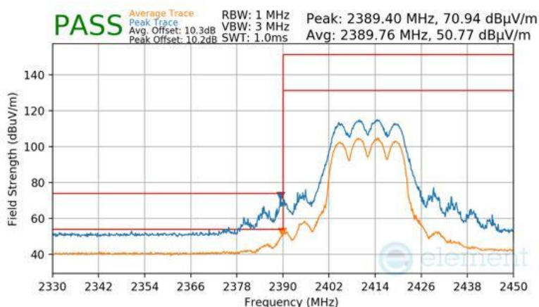
Plot 7-343 Radiated Restricted Lower Band Edge Measurement CDD Diversity (Peak & Average – RU242)
