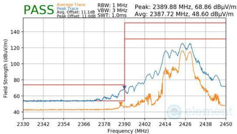
Plot 7-285 Radiated Restricted Lower Band Edge Measurement CDD Primary (Peak & Average – RU52+26)
