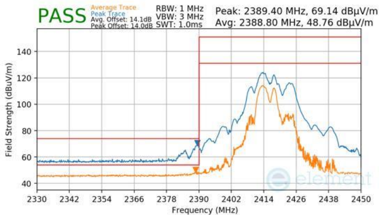
Plot 7-323 Radiated Restricted Lower Band Edge Measurement CDD Diversity (Peak & Average – RU52+26)
