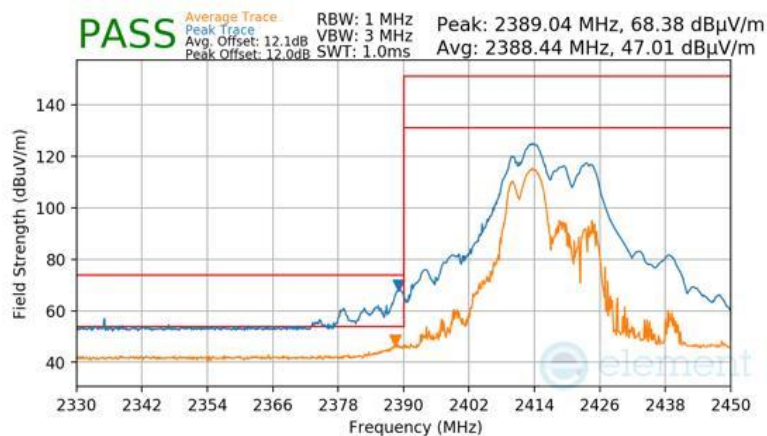
Plot 7-280 Radiated Restricted Lower Band Edge Measurement CDD Primary (Peak & Average – RU52+26)
