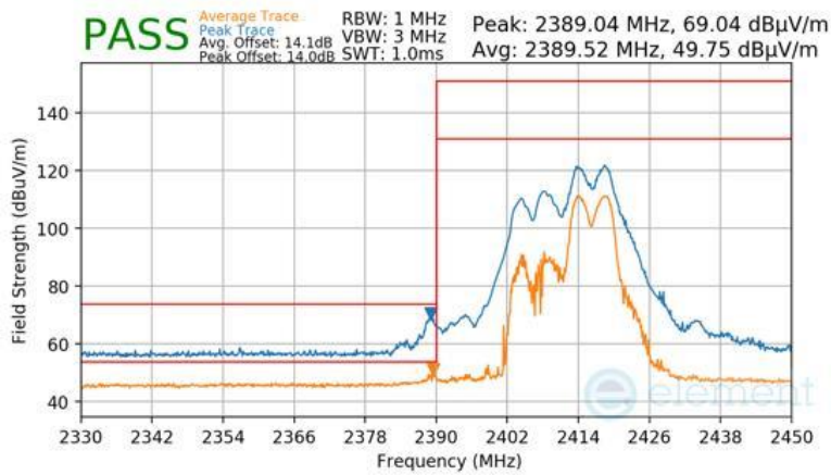
Plot 7-321 Radiated Restricted Lower Band Edge Measurement CDD Diversity (Peak & Average – RU52+26)
