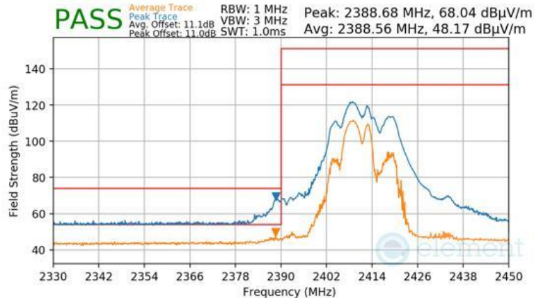
Plot 7-278 Radiated Restricted Lower Band Edge Measurement CDD Primary (Peak & Average – RU52+26)
