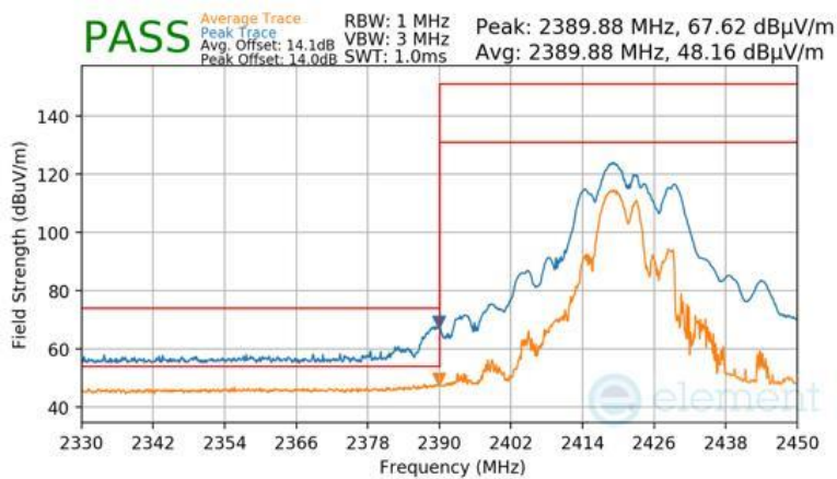
Plot 7-326 Radiated Restricted Lower Band Edge Measurement CDD Diversity (Peak & Average – RU52+26)
