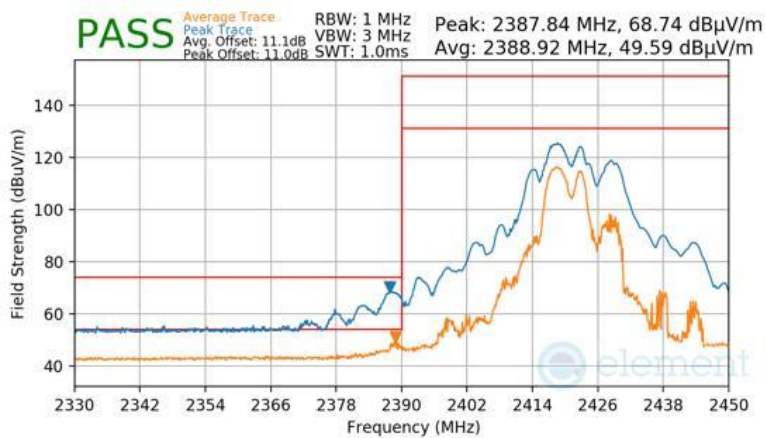
Plot 7-284 Radiated Restricted Lower Band Edge Measurement CDD Primary (Peak & Average – RU52+26)
