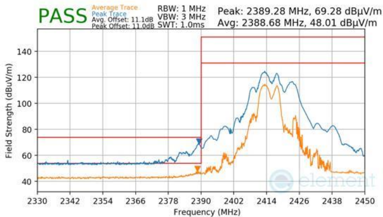
Plot 7-281 Radiated Restricted Lower Band Edge Measurement CDD Primary (Peak & Average – RU52+26)
