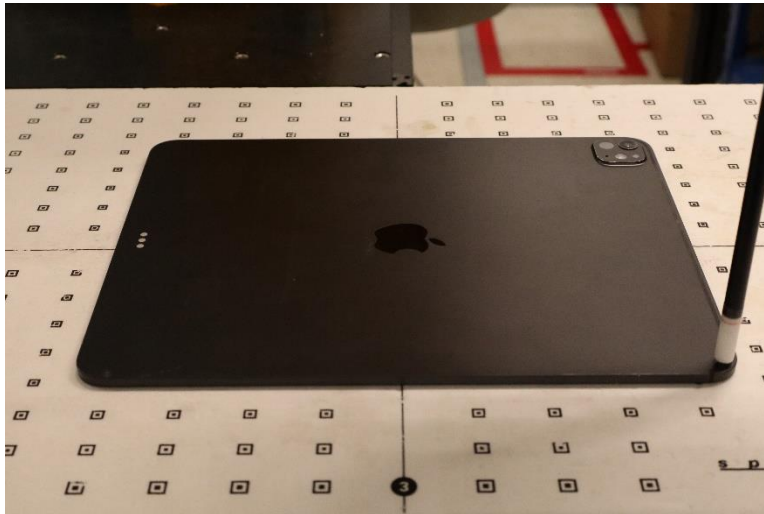
Near Field Power Density Test Setup Photo 19: Body, Back Side at 2mm – WF7
