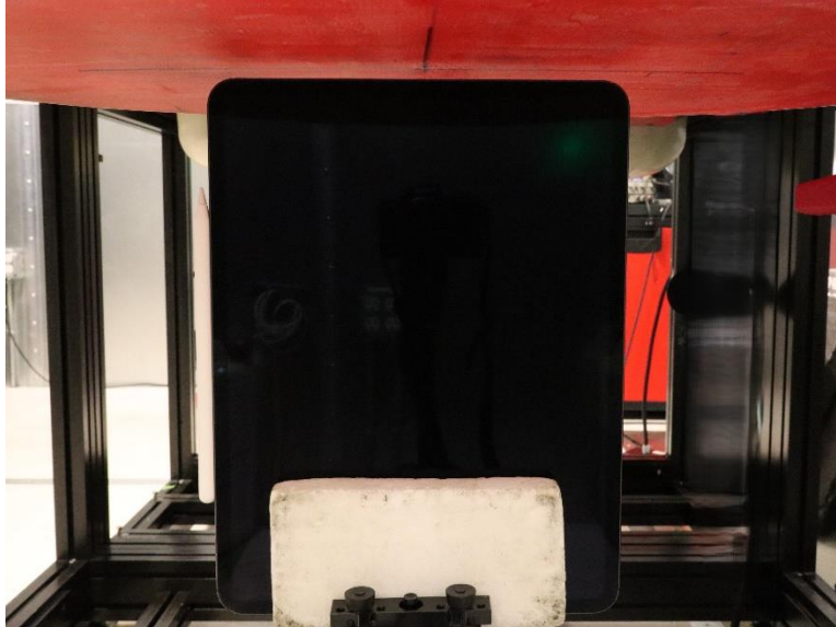
Wireless Power Transfer (wPT) Test Setup Photo 12: Body, Bottom Edge at 5mm
