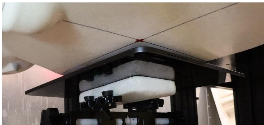
SAR Test Setup Photo 3: Body, Back Side at 5mm – Antenna WF7
