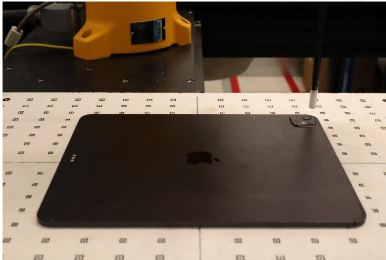
Near Field Power Density Test Setup Photo 23: Body, Back side at 9.22mm – WF8
