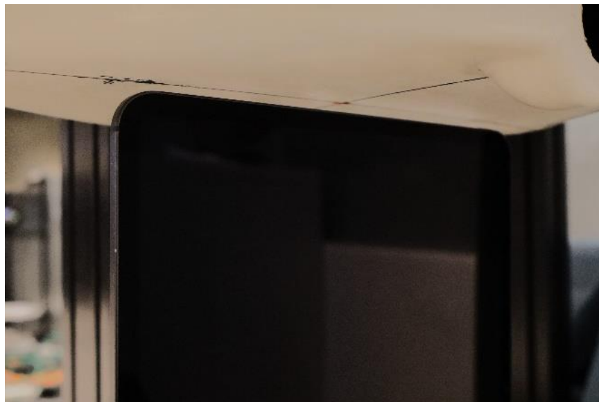
SAR Test Setup Photo 9: Body, Top Edge at 5mm – Antenna WF7/WF8/WF9/WF5B
