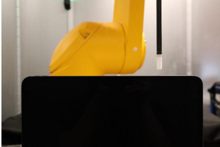
Near Field Power Density Test Setup Photo 18: Body, Right Edge at 9.57mm – WF5B
