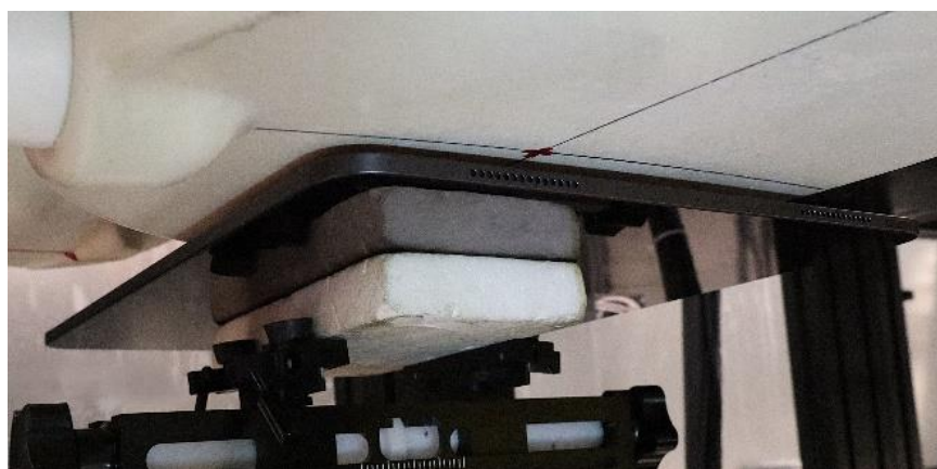
SAR Test Setup Photo 4: Body, Back Side at 5mm – Antenna WF9
