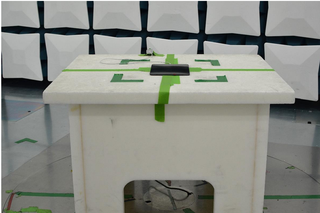
Figure 11: 30MHz-1GHz Test Setup (Front View)
