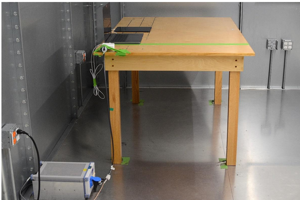
Figure 4: AC Line Conducted Emissions (Side View)
