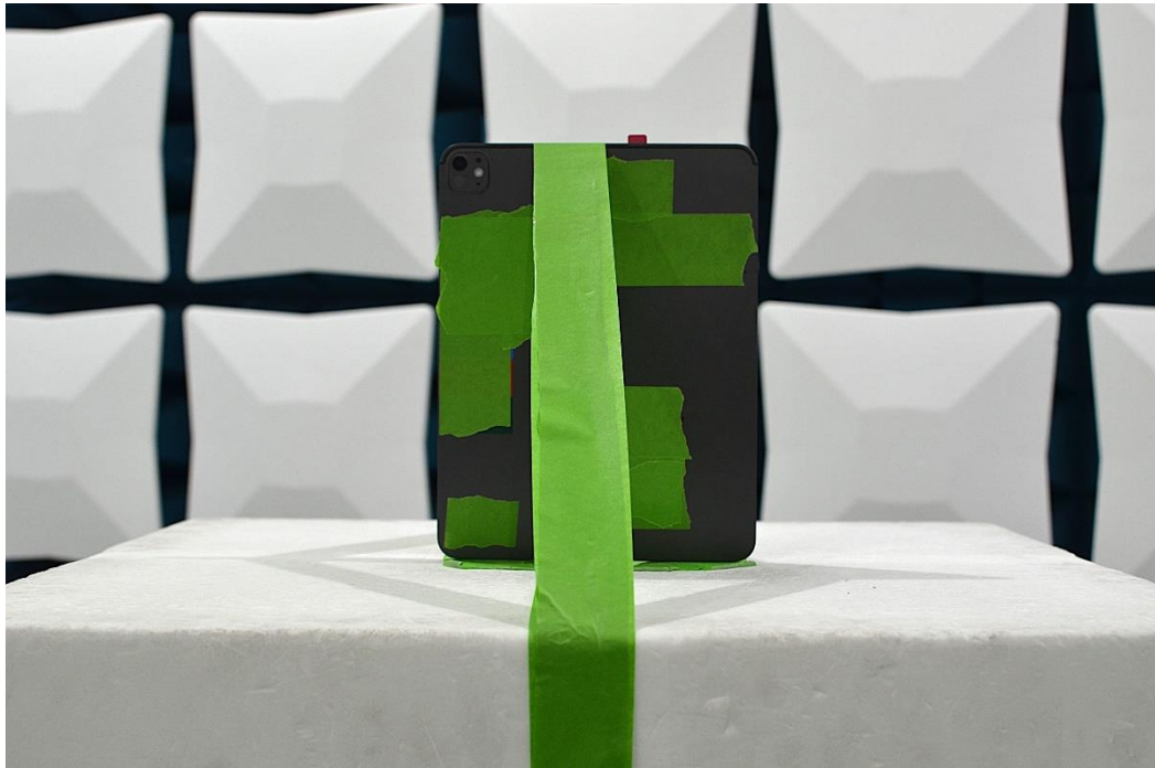
Figure 9: 1-18GHz Test Setup (Front View)
