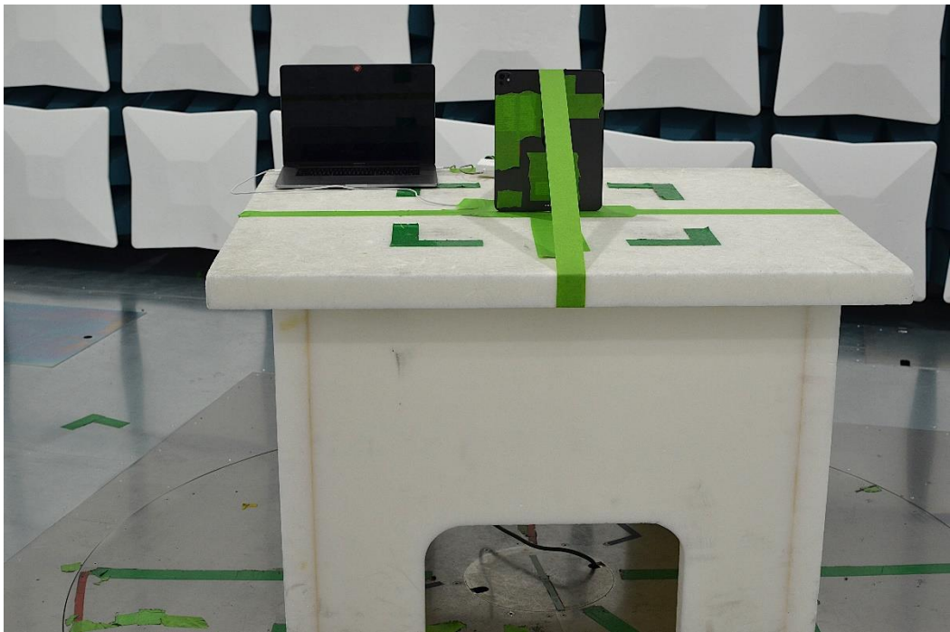
Figure 21: 30MHz-1GHz Test Setup (Front View)
