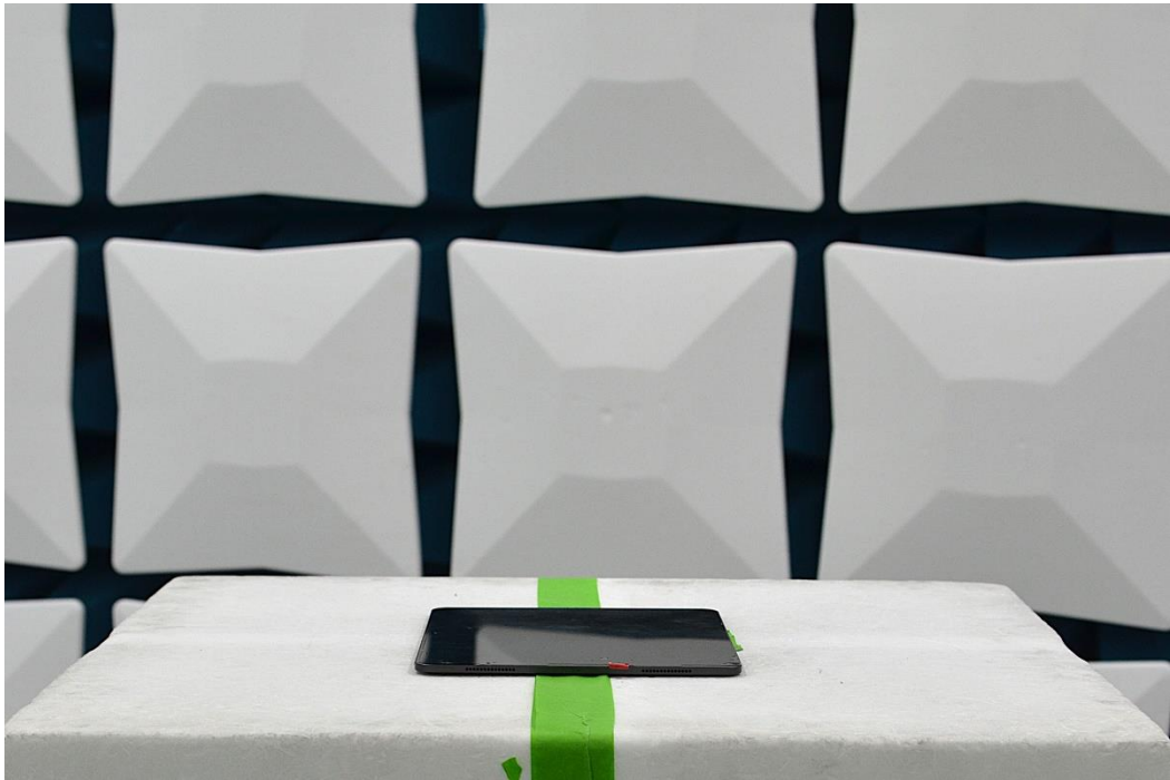
Figure 5: 1-18GHz Test Setup (Front View)
