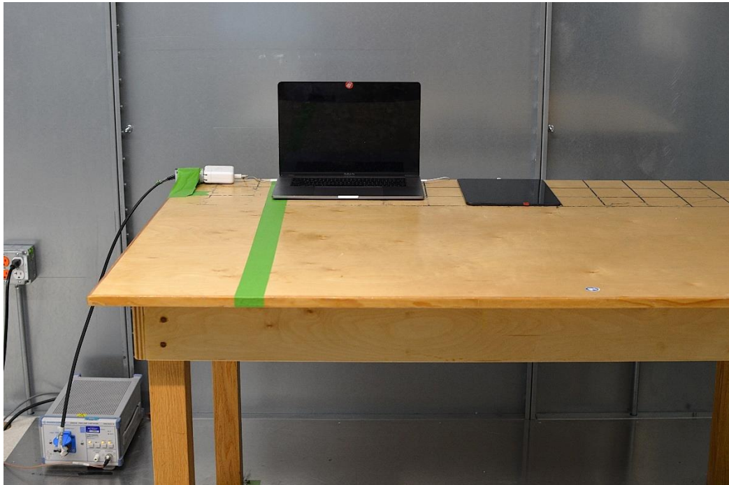
Figure 3: AC Line Conducted Emissions (Front View)
