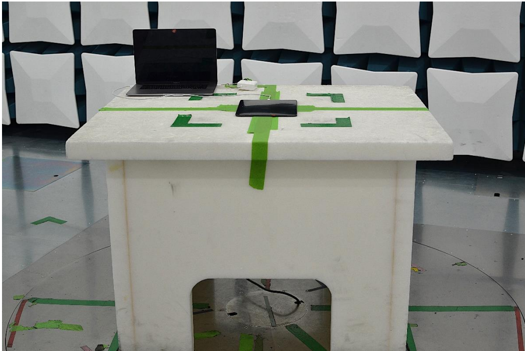
Figure 17: 30MHz-1GHz Test Setup (Front View)
