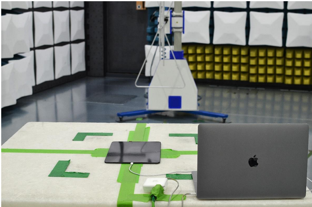
Figure 18: 30MHz-1GHz Test Setup (Rear View)
