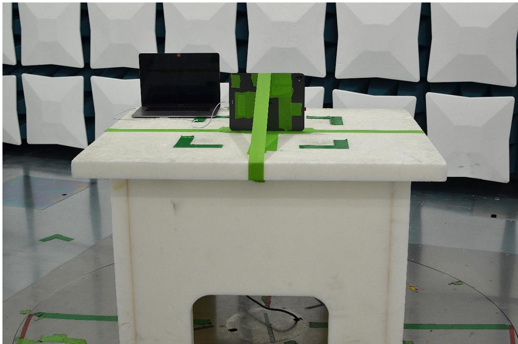
Figure 19: 30MHz-1GHz Test Setup (Front View)
