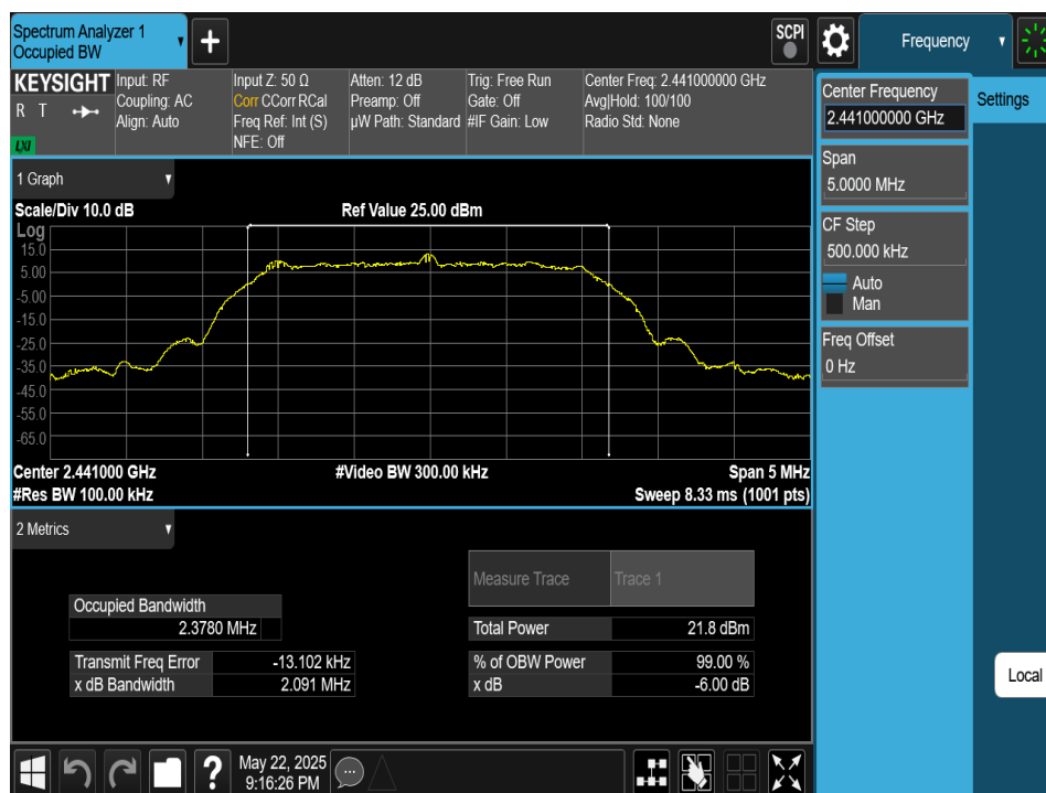
Plot 7-8. 6dB BW & 99% OBW Plot Antenna 4a (Bluetooth (HDRPS2), 2Mbps, ePA – Ch. 38)
