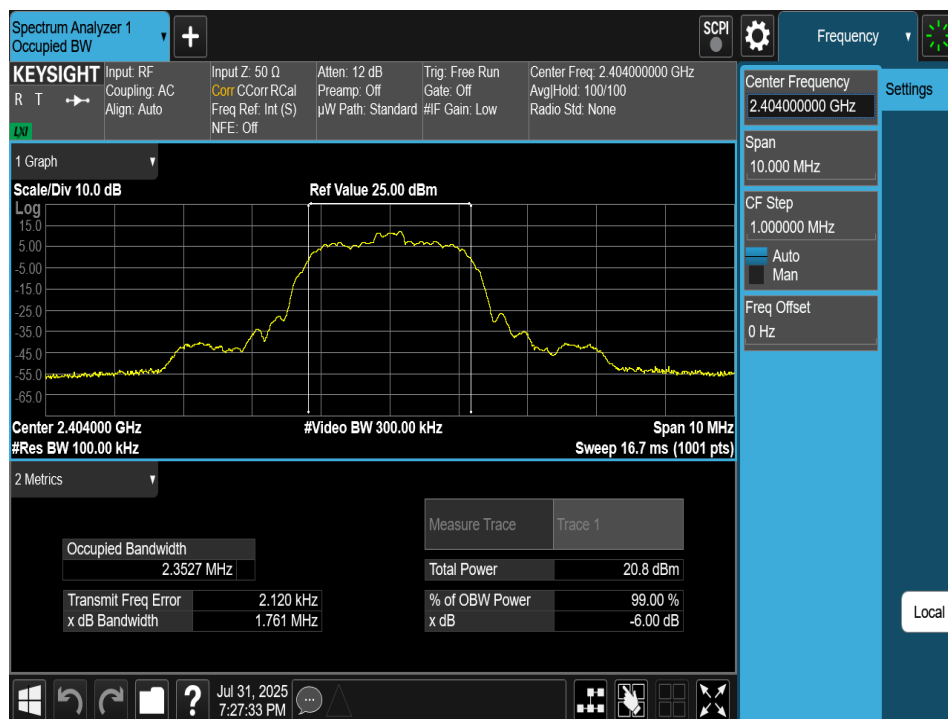
Plot 7-1. 6dB BW & 99% OBW Plot Antenna 4a (Bluetooth (HDR4), 4Mbps, ePA – Ch. 1)
