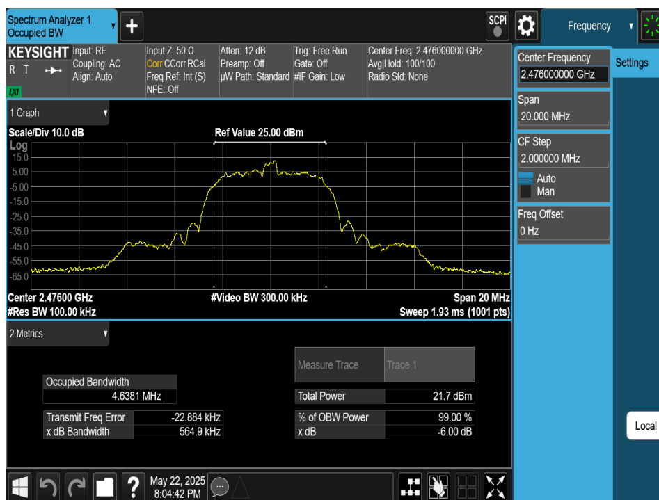
Plot 7-6. 6dB BW & 99% OBW Plot Antenna 4a (Bluetooth (HDR8), 8Mbps, ePA – Ch. 73)
