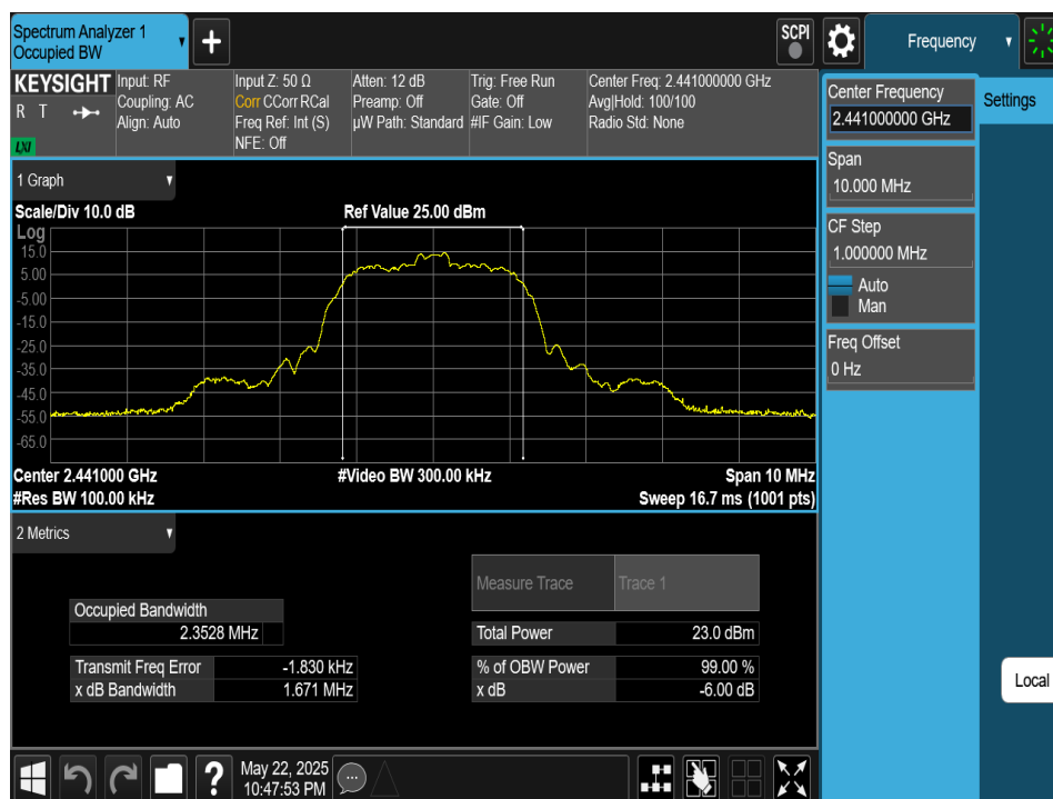
Plot 7-20. 6dB BW & 99% OBW Plot Antenna 2a (Bluetooth (HDR4), 4Mbps, ePA – Ch. 38)
