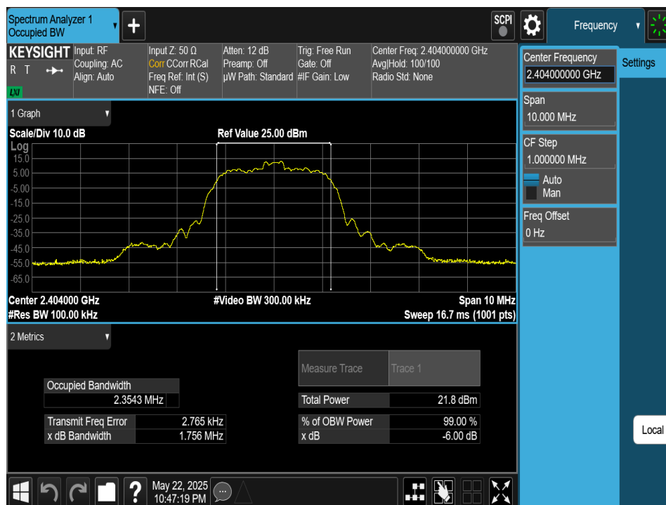
Plot 7-19. 6dB BW & 99% OBW Plot Antenna 2a (Bluetooth (HDR4), 4Mbps, ePA – Ch. 1)
