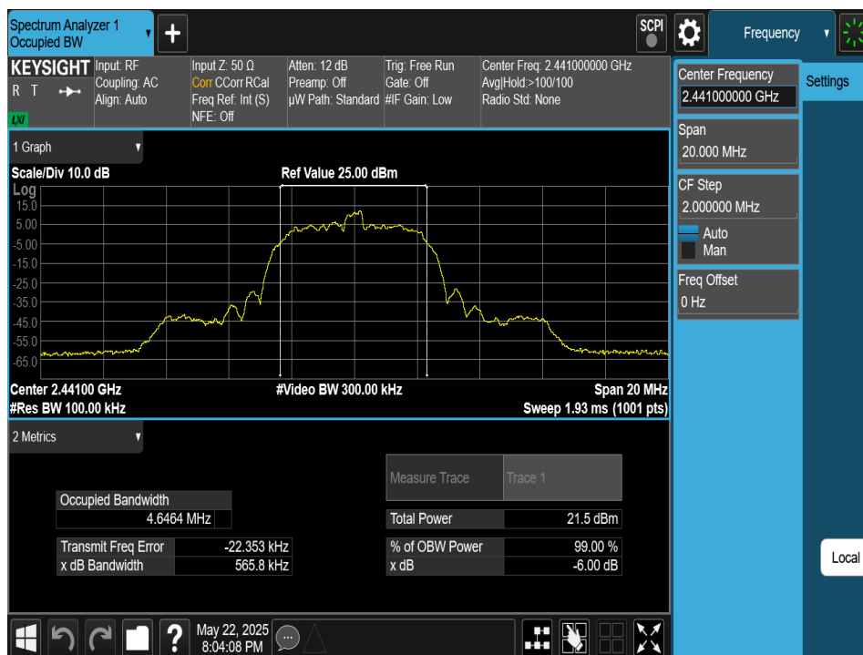
Plot 7-5. 6dB BW & 99% OBW Plot Antenna 4a (Bluetooth (HDR8), 8Mbps, ePA – Ch. 38)
