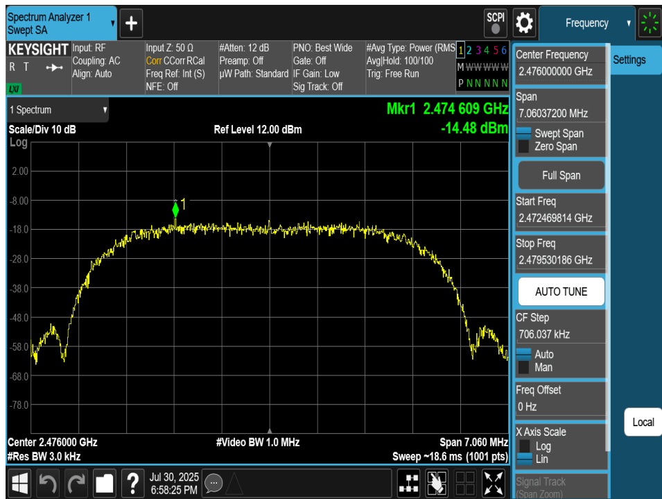
Plot 7-60. Power Spectral Density Plot Antenna 4a (Bluetooth (XHDRPM6), 6Mbps, iPA – Ch. 73)
