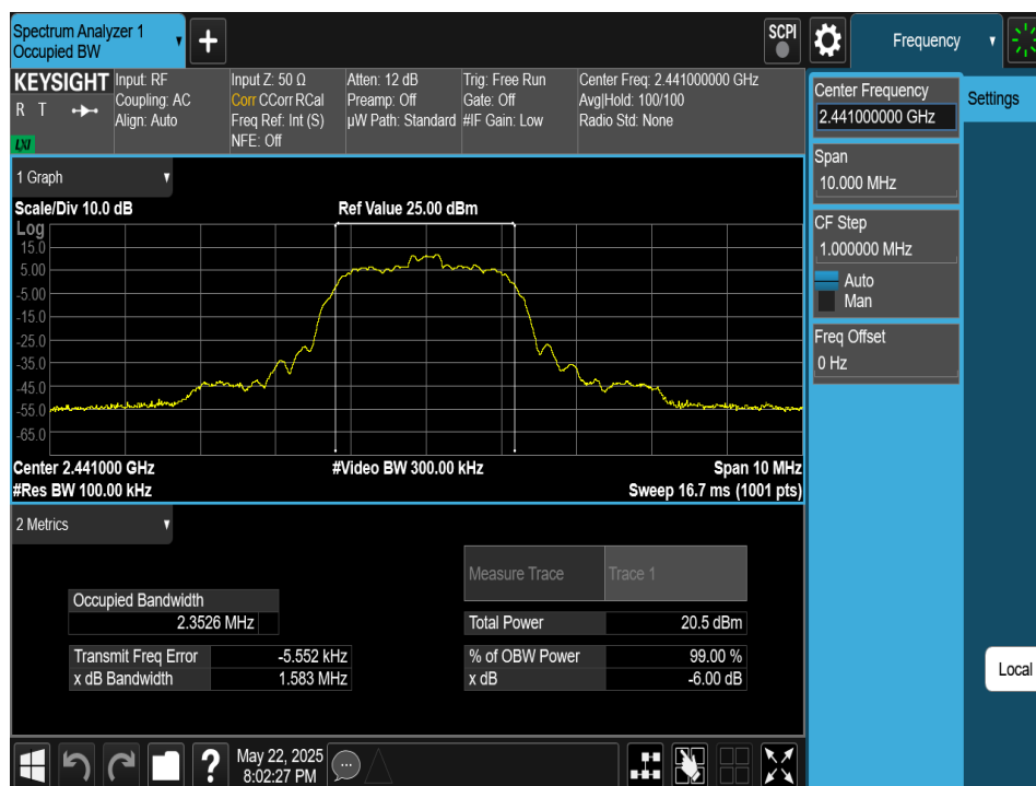
Plot 7-2. 6dB BW & 99% OBW Plot Antenna 4a (Bluetooth (HDR4), 4Mbps, ePA – Ch. 38)
