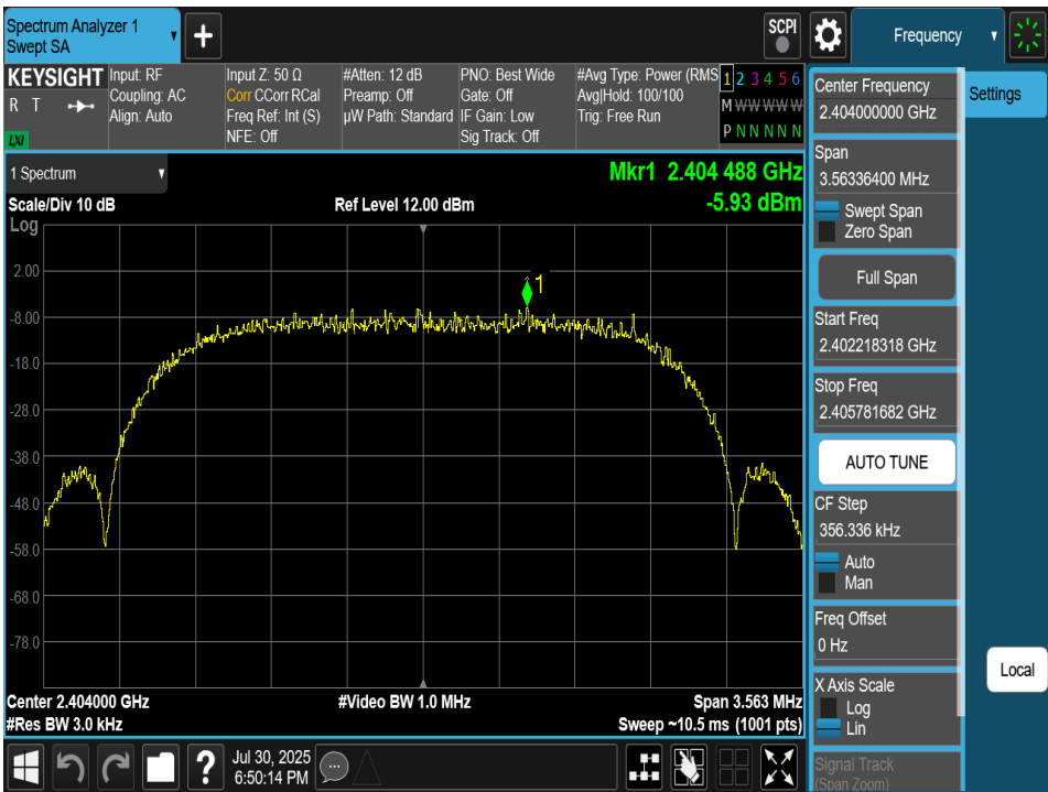
Plot 7-49. Power Spectral Density Plot Antenna 4a (Bluetooth (HDRPS2), 2Mbps, ePA – Ch. 1)
