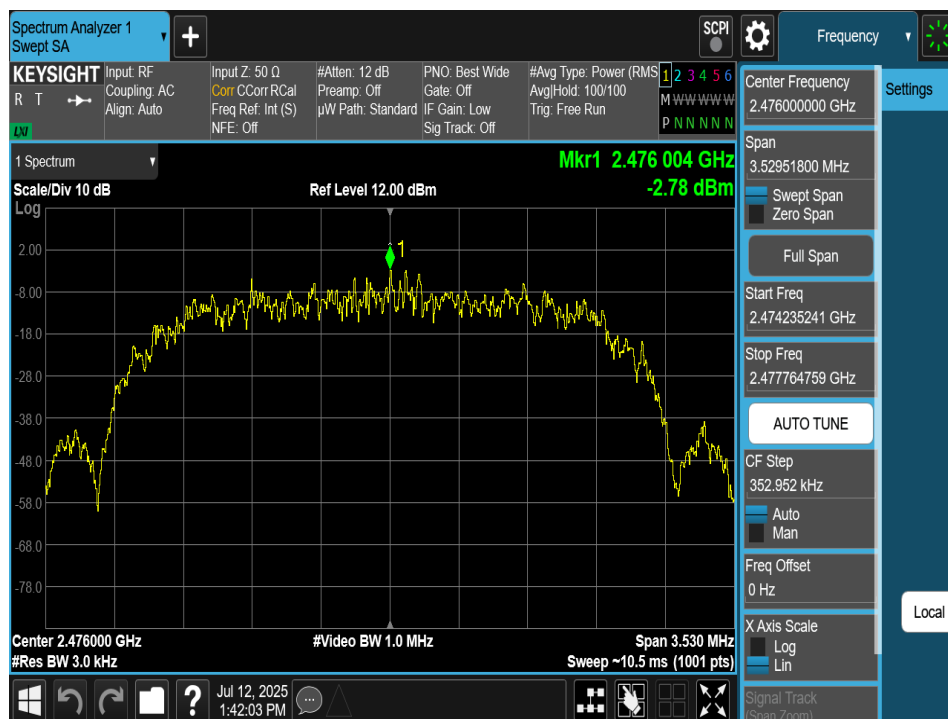
Plot 7-39. Power Spectral Density Plot Antenna 4a (Bluetooth (HDR4), 4Mbps, ePA – Ch. 73)
