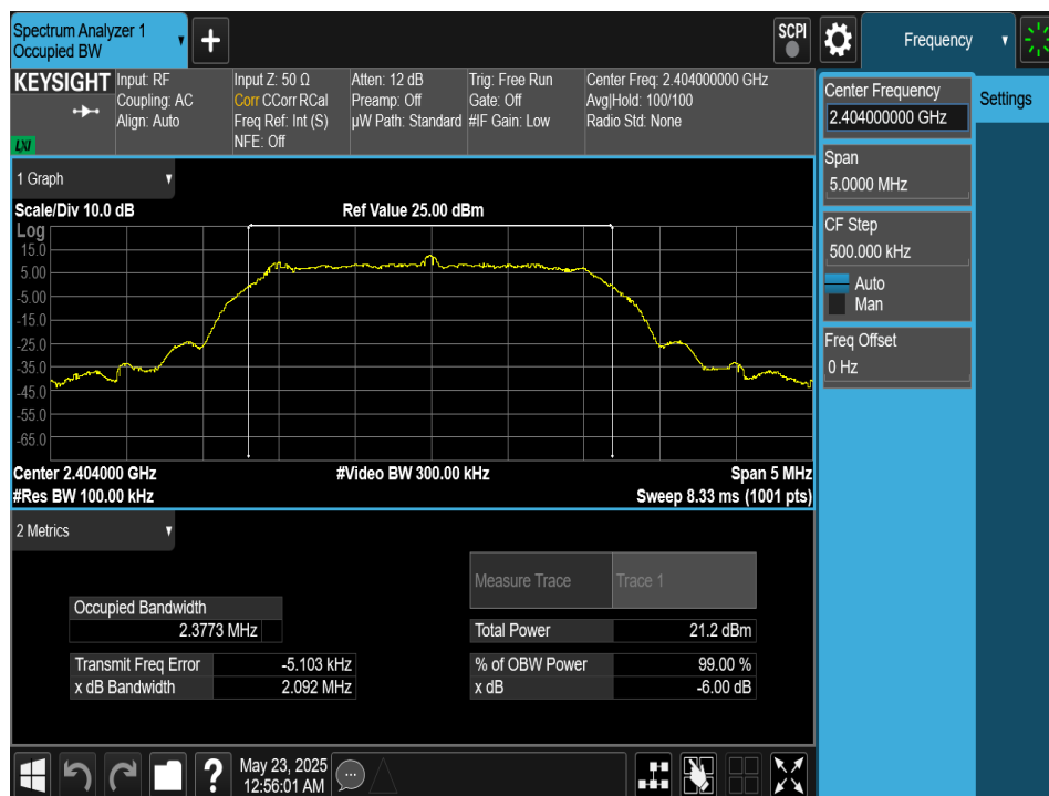
Plot 7-25. 6dB BW & 99% OBW Plot Antenna 2a (Bluetooth (HDRPS2), 2Mbps, ePA – Ch. 1)
