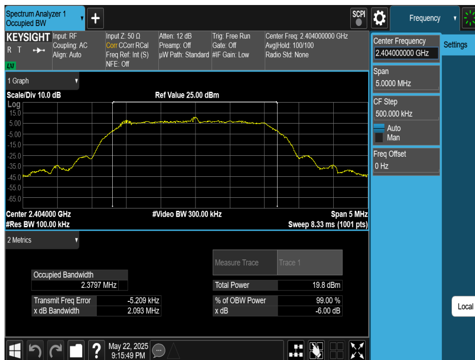
Plot 7-7. 6dB BW & 99% OBW Plot Antenna 4a (Bluetooth (HDRPS2), 2Mbps, ePA – Ch. 1)
