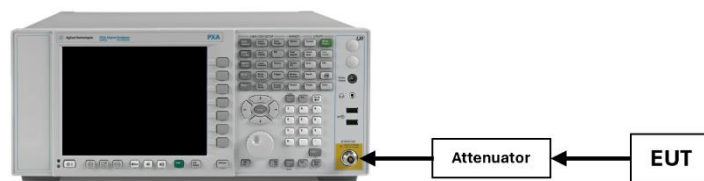
Figure 7-4. Test Instrument & Measurement Setup
