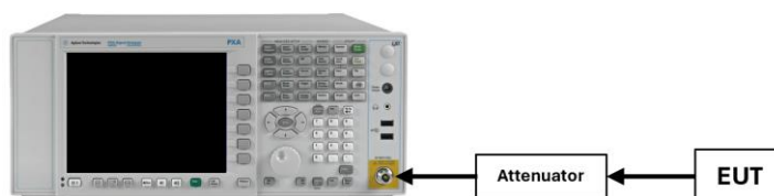
Figure 7-3. Test Instrument & Measurement Setup
