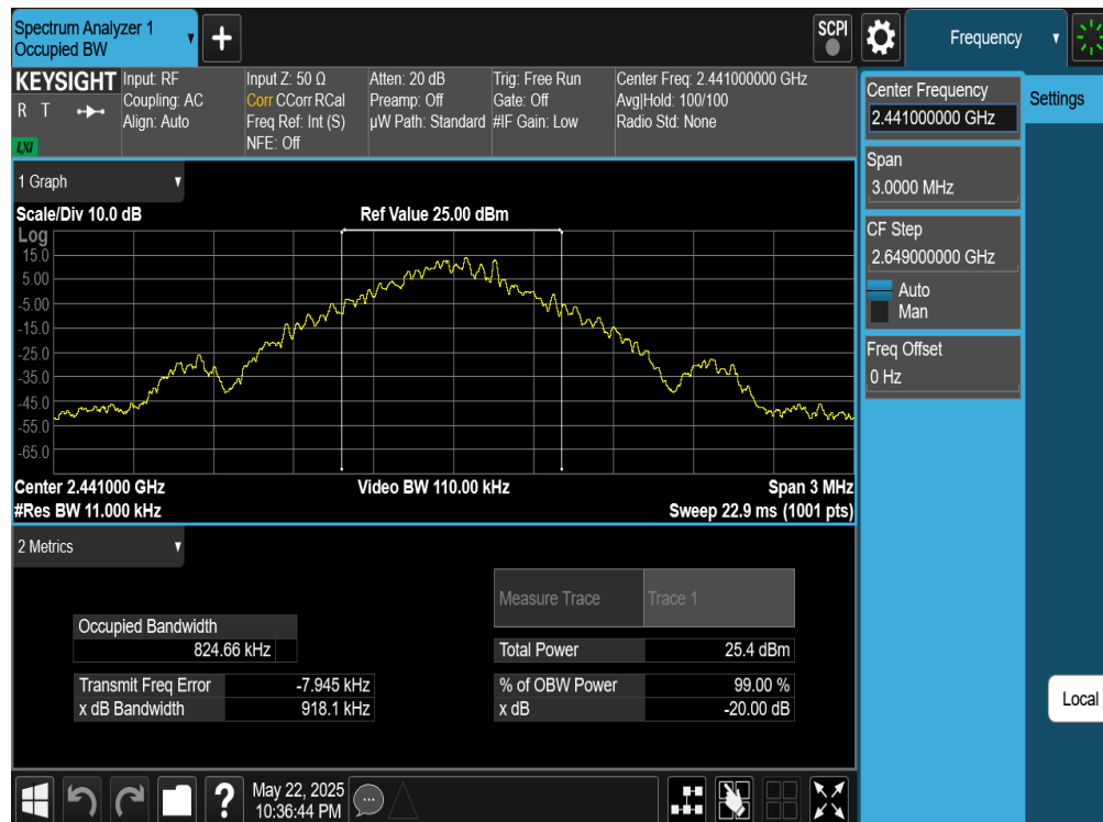
Plot 7-8. 20dB BW and 99% OBW Plot Antenna 2a (Bluetooth, GFSK, ePA – Ch. 39)
