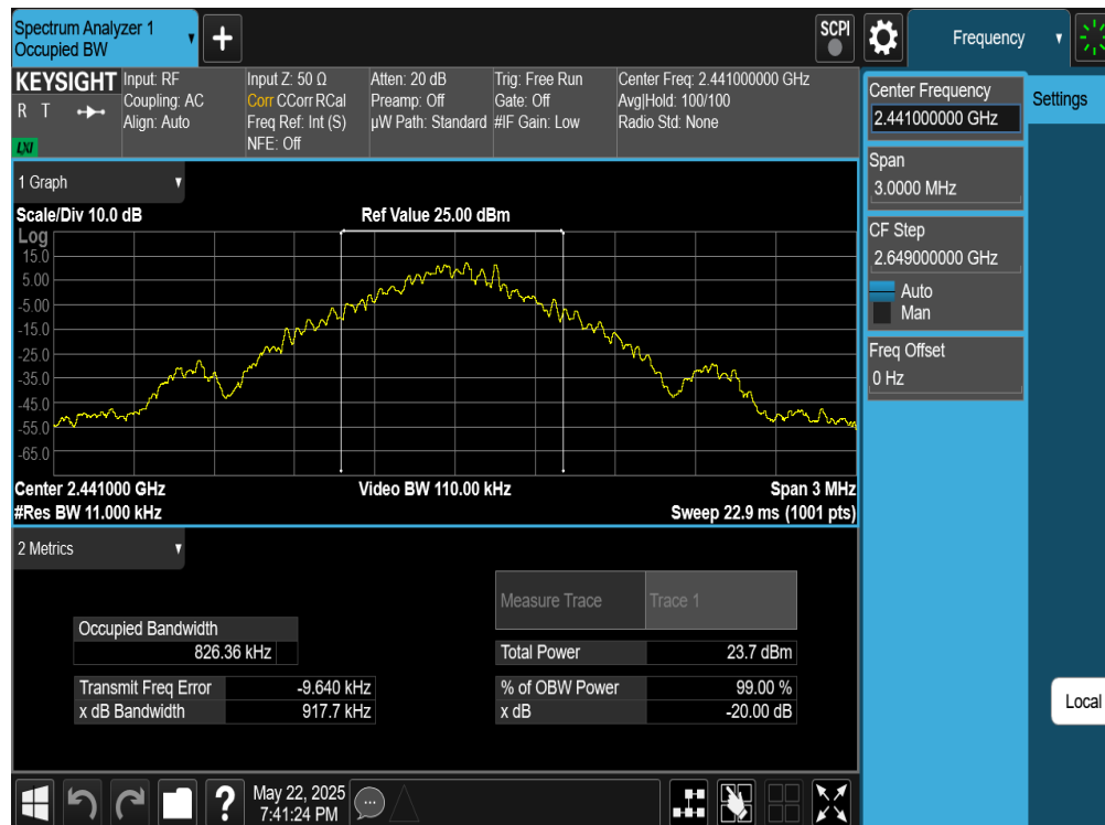
Plot 7-2. 20dB BW and 99% OBW Plot Antenna 4a (Bluetooth, GFSK, ePA – Ch. 39)
