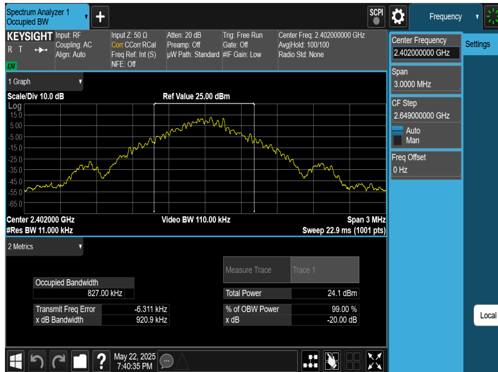
Plot 7-1. 20dB BW and 99% OBW Plot Antenna 4a (Bluetooth, GFSK, ePA – Ch. 0)
