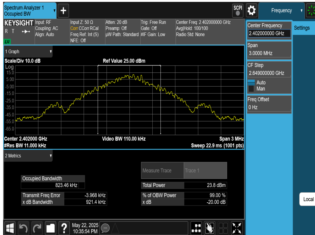
Plot 7-7. 20dB BW and 99% OBW Plot Antenna 2a (Bluetooth, GFSK, ePA – Ch. 0)
