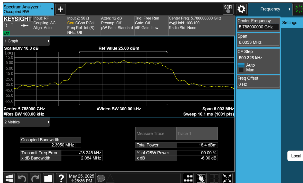
Plot 7-52. 6dB BW & 99% OBW Antenna WF5B (NB UNII HDT6, ePA– 5788MHz)
