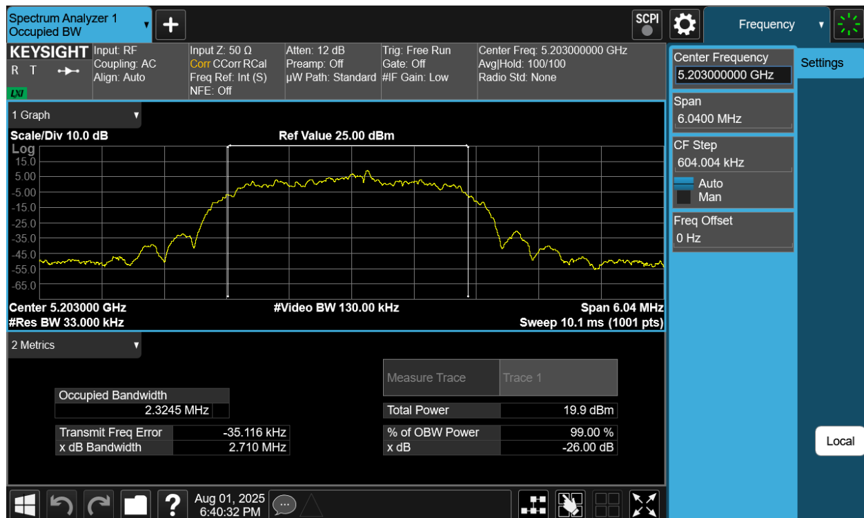
Plot 7-17. 26dB BW & 99% OBW Antenna 4a (NB UNII HDR4, ePA- 5203MHz)
