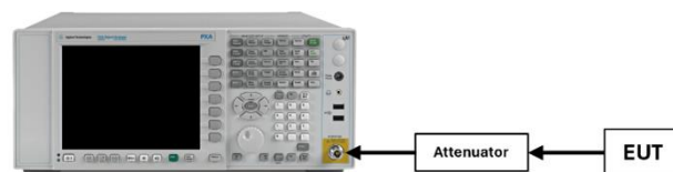
Figure 7-1. Test Instrument & Measurement Setup
