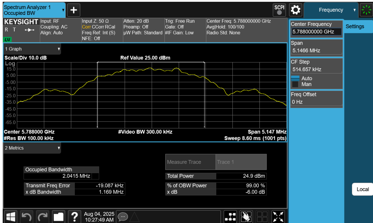
Plot 7-55. 6dB BW & 99% OBW Antenna 4a (NB UNII LE2M, ePA– 5788MHz)
