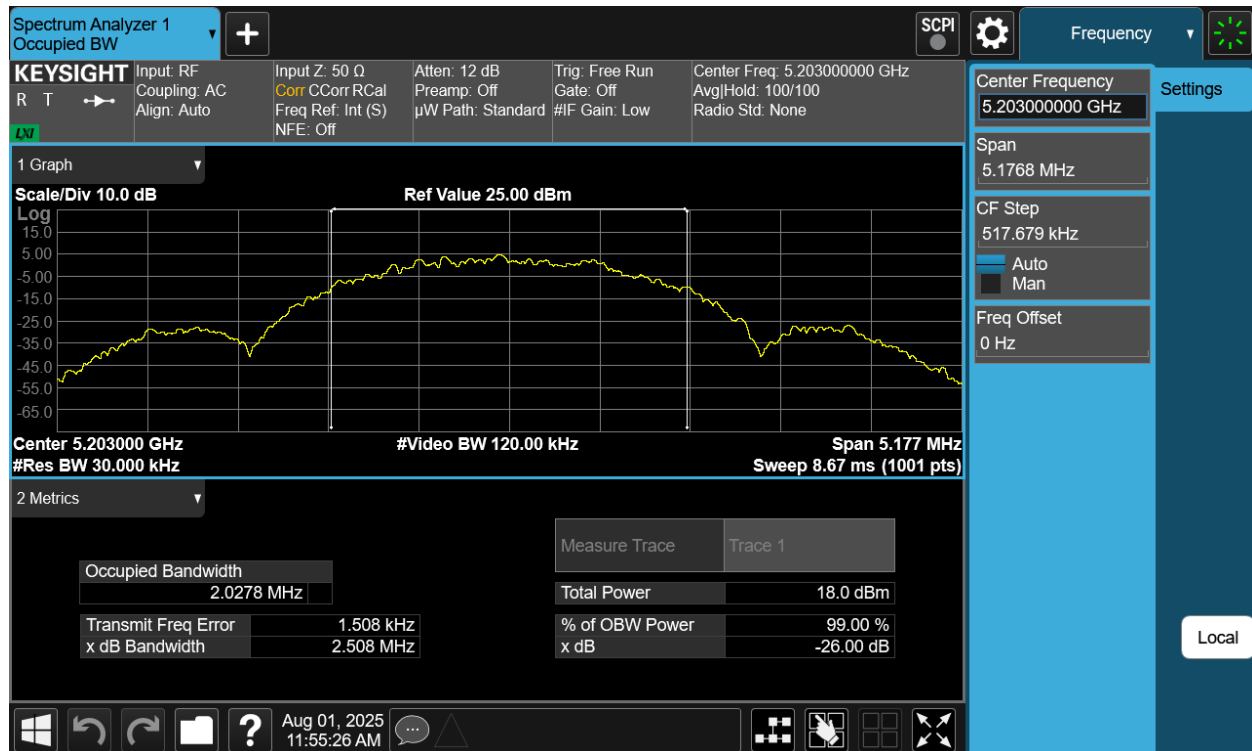
Plot 7-29. 26dB BW & 99% OBW Antenna 2a (NB UNII LE2M, ePA- 5203MHz)
