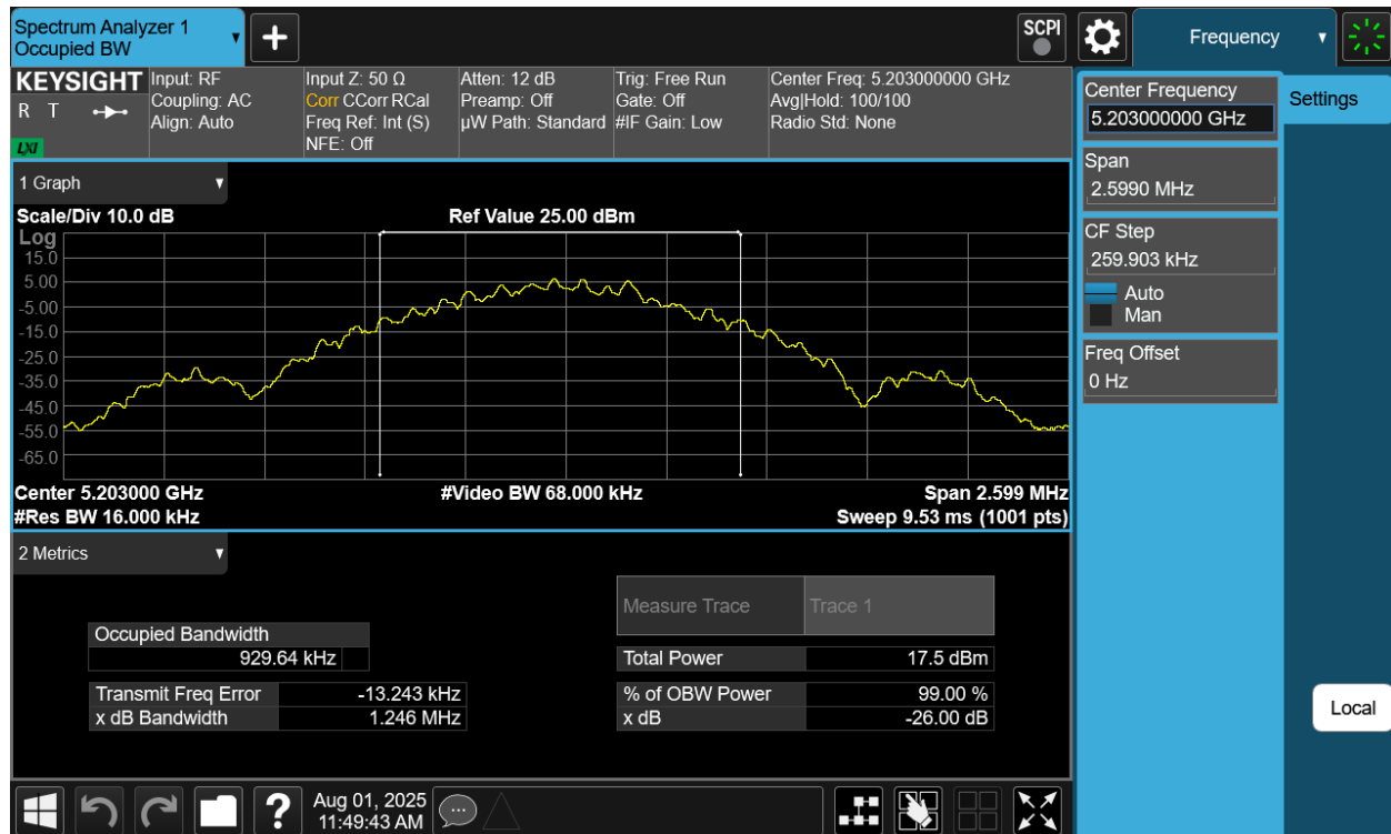
Plot 7-27. 26dB BW & 99% OBW Antenna 2a (NB UNII BDR, ePA- 5203MHz)
