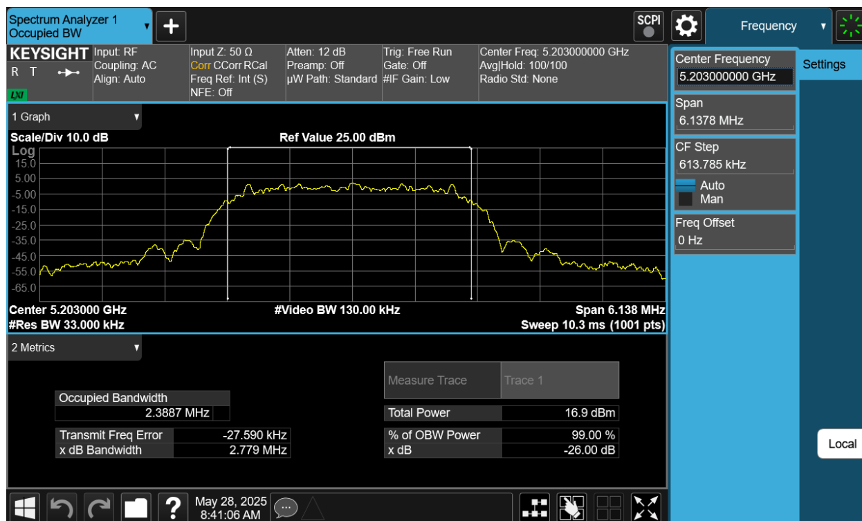
Plot 7-39. 26dB BW & 99% OBW Antenna 2a (NB UNII HDT6, ePA- 5203MHz)
