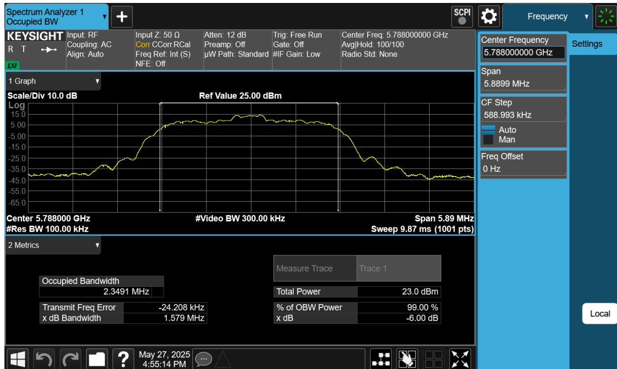
Plot 7-56. 6dB BW & 99% OBW Antenna 4a (NB UNII HDR4, ePA – 5788MHz)
