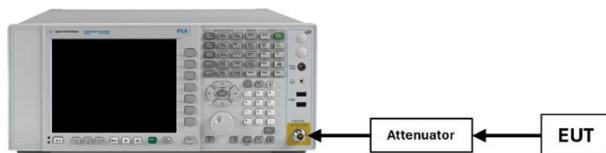
Figure 7-2. Test Instrument & Measurement Setup
