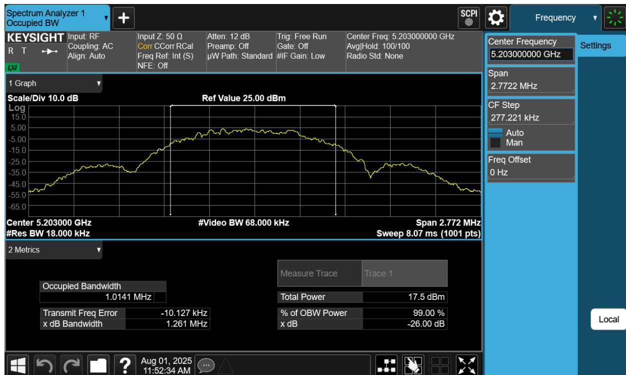
Plot 7-28. 26dB BW & 99% OBW Antenna 2a (NB UNII LE1M, ePA- 5203MHz)
