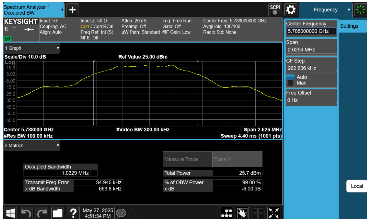
Plot 7-54. 6dB BW & 99% OBW Antenna 4a (NB UNII LE1M, ePA – 5788MHz)
