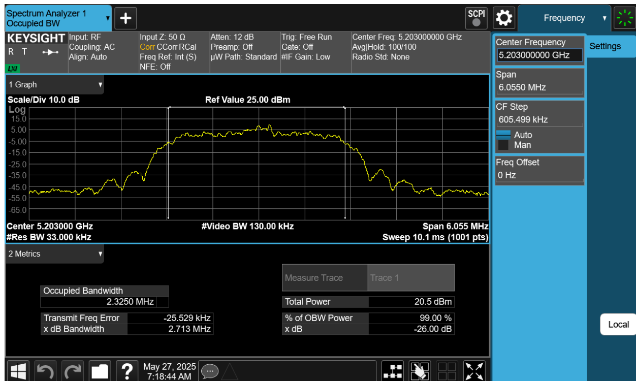
Plot 7-30. 26dB BW & 99% OBW Antenna 2a (NB UNII HDR4, ePA- 5203MHz)
