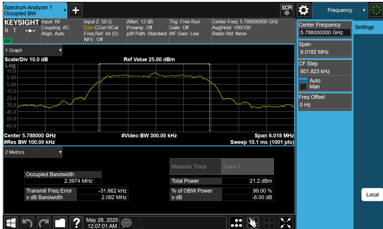
Plot 7-64. 6dB BW & 99% OBW Antenna 4a (NB UNII HDT4, ePA- 5788MHz)
