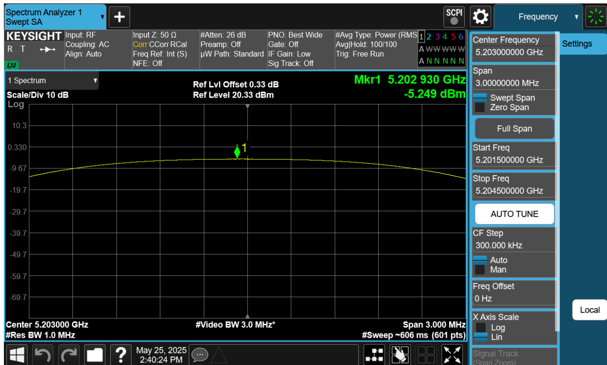
Plot 7-102. PSD Antenna WF5B (NB UNII HDT4, iPA – 5203MHz)
