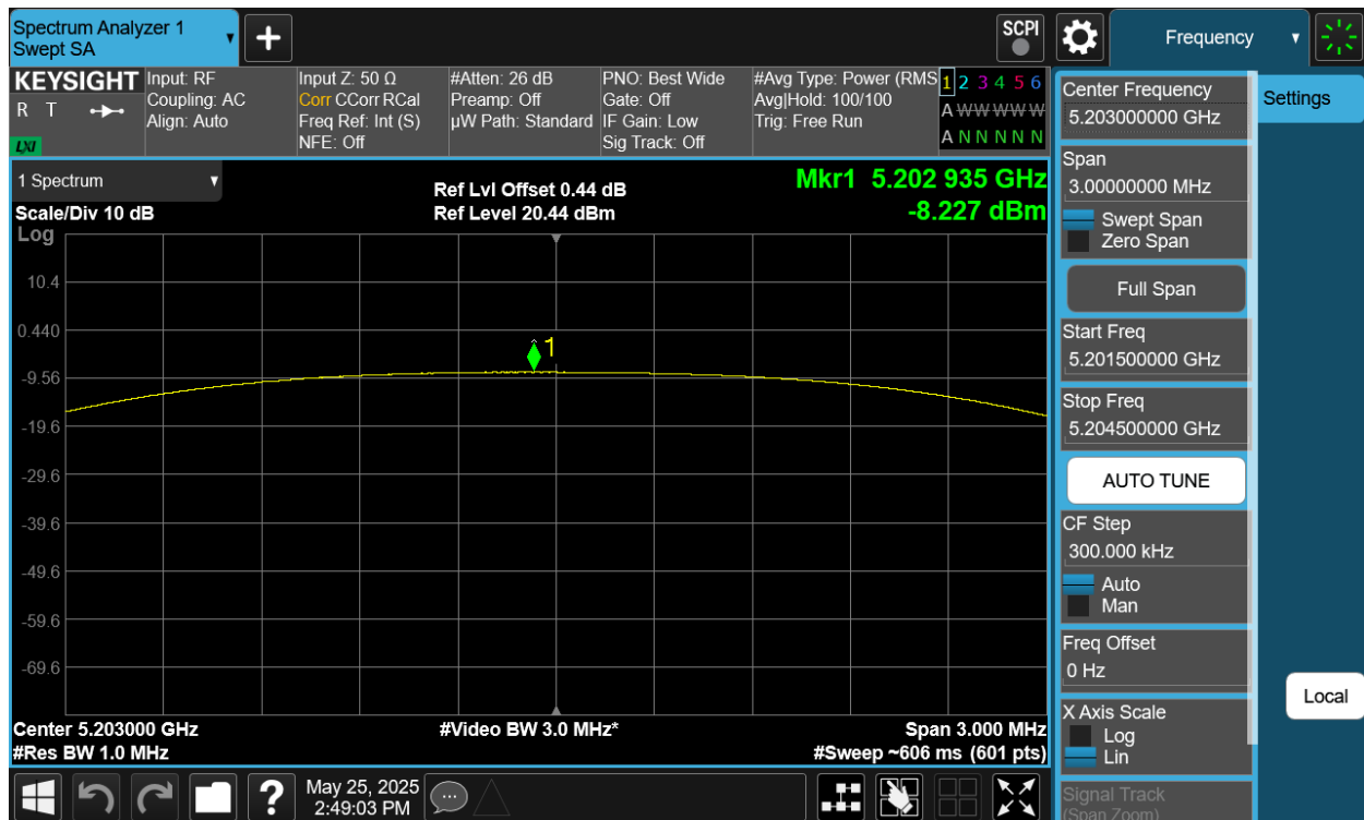
Plot 7-104. PSD Antenna WF5B (NB UNII HDT6, iPA – 5203MHz)
