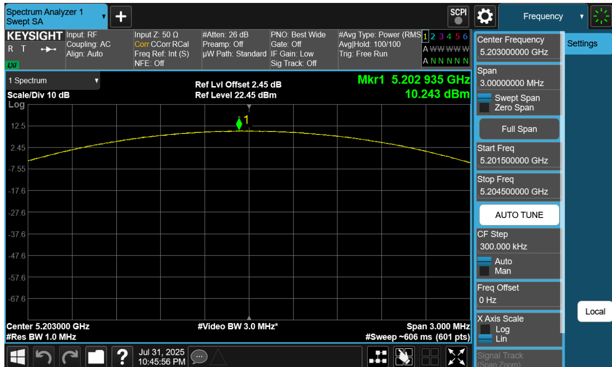
Plot 7-83. PSD Antenna WF5B (NB UNII LE2M, ePA – 5203MHz)
