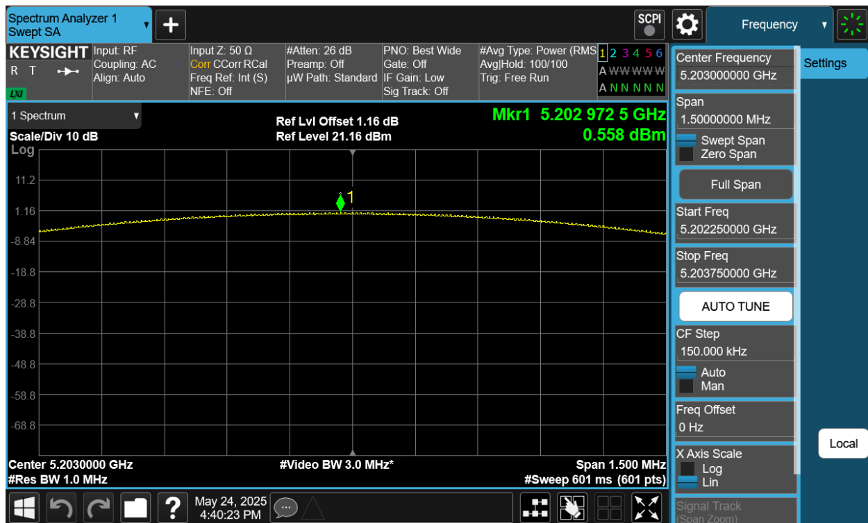
Plot 7-80. PSD Antenna WF5B (NB UNII BDR, iPA – 5203MHz)
