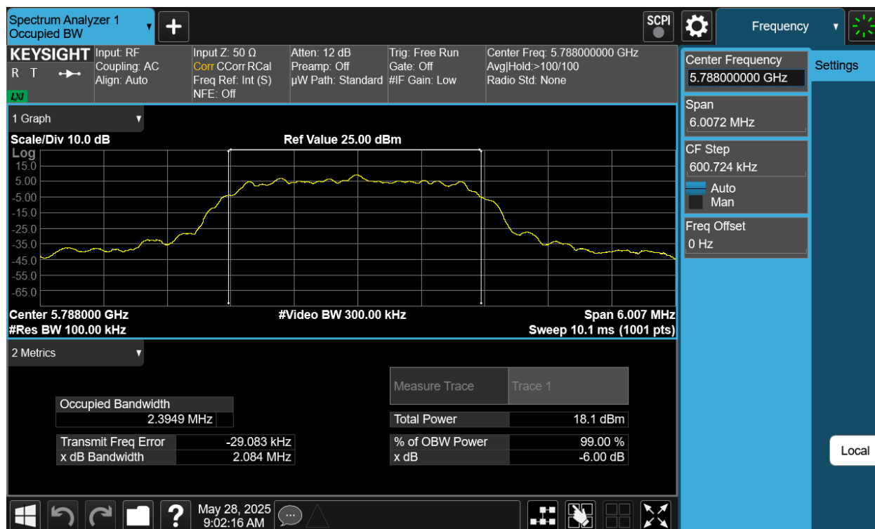
Plot 7-78. 6dB BW & 99% OBW Antenna 2a (NB UNII HDT6, ePA- 5788MHz)
