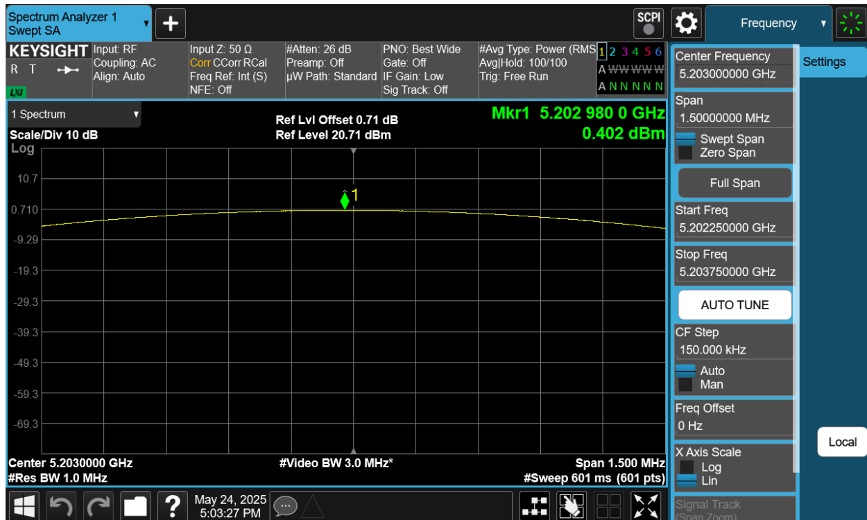
Plot 7-82. PSD Antenna WF5B (NB UNII LE1M, iPA – 5203MHz)
