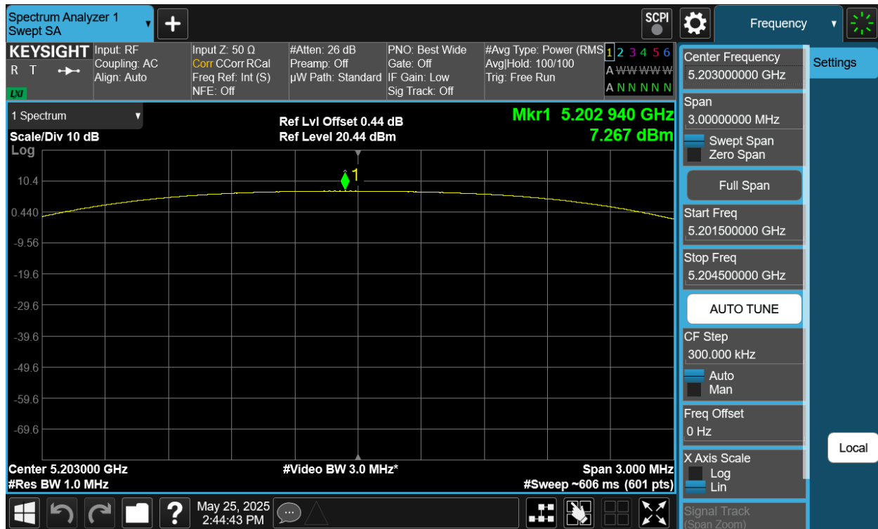
Plot 7-103. PSD Antenna WF5B (NB UNII HDT6, ePA – 5203MHz)
