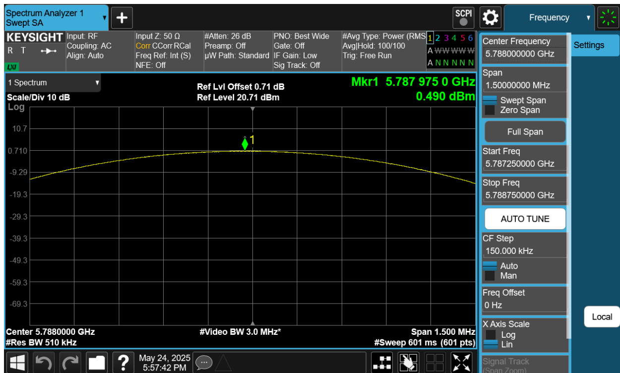
Plot 7-108. PSD Antenna WF5B (NB UNII LE1M, iPA – 5788MHz)
