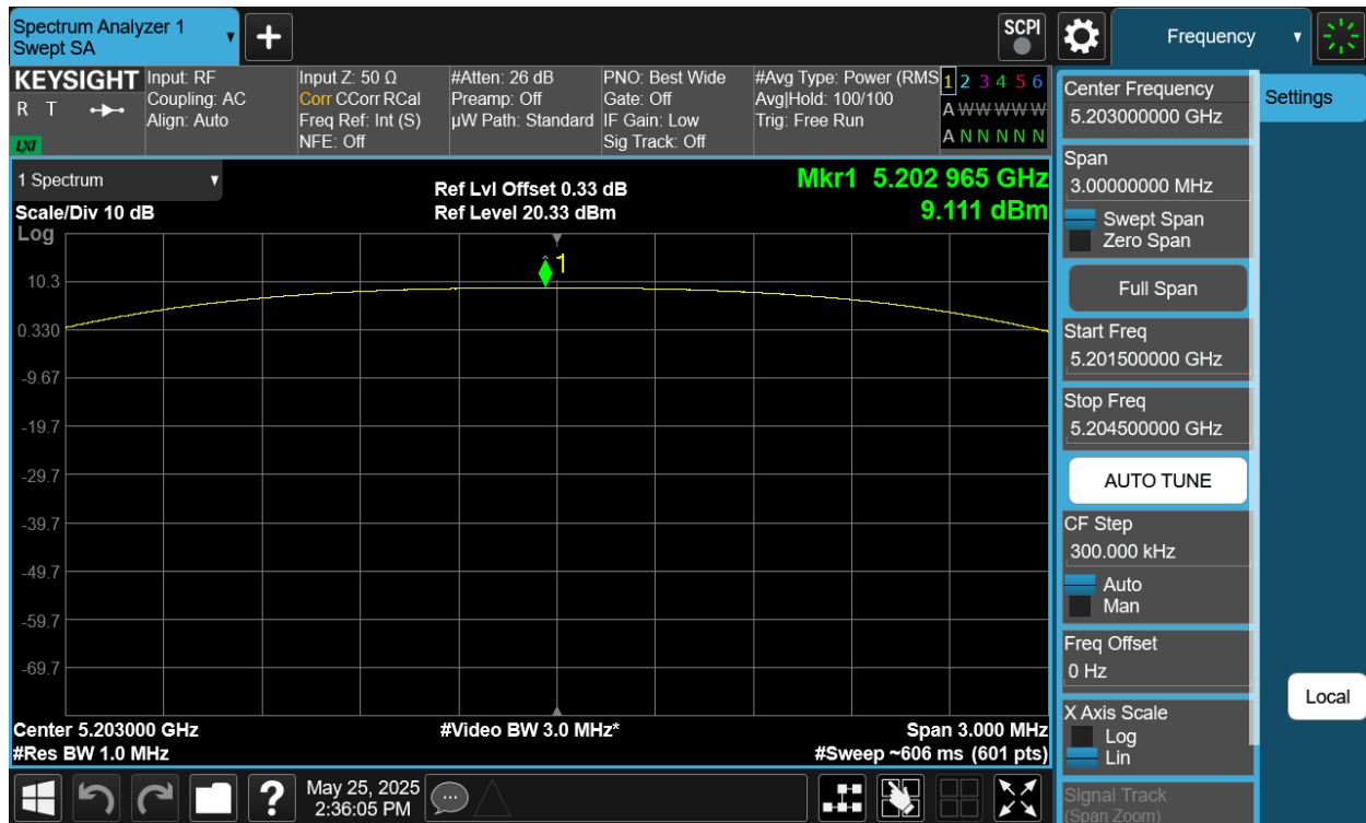
Plot 7-101. PSD Antenna WF5B (NB UNII HDT4, ePA – 5203MHz)
