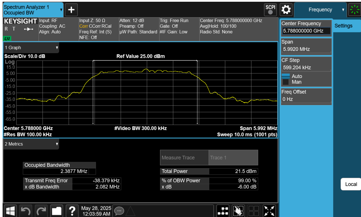
Plot 7-63. 6dB BW & 99% OBW Antenna 4a (NB UNII HDT2, ePA- 5788MHz)
