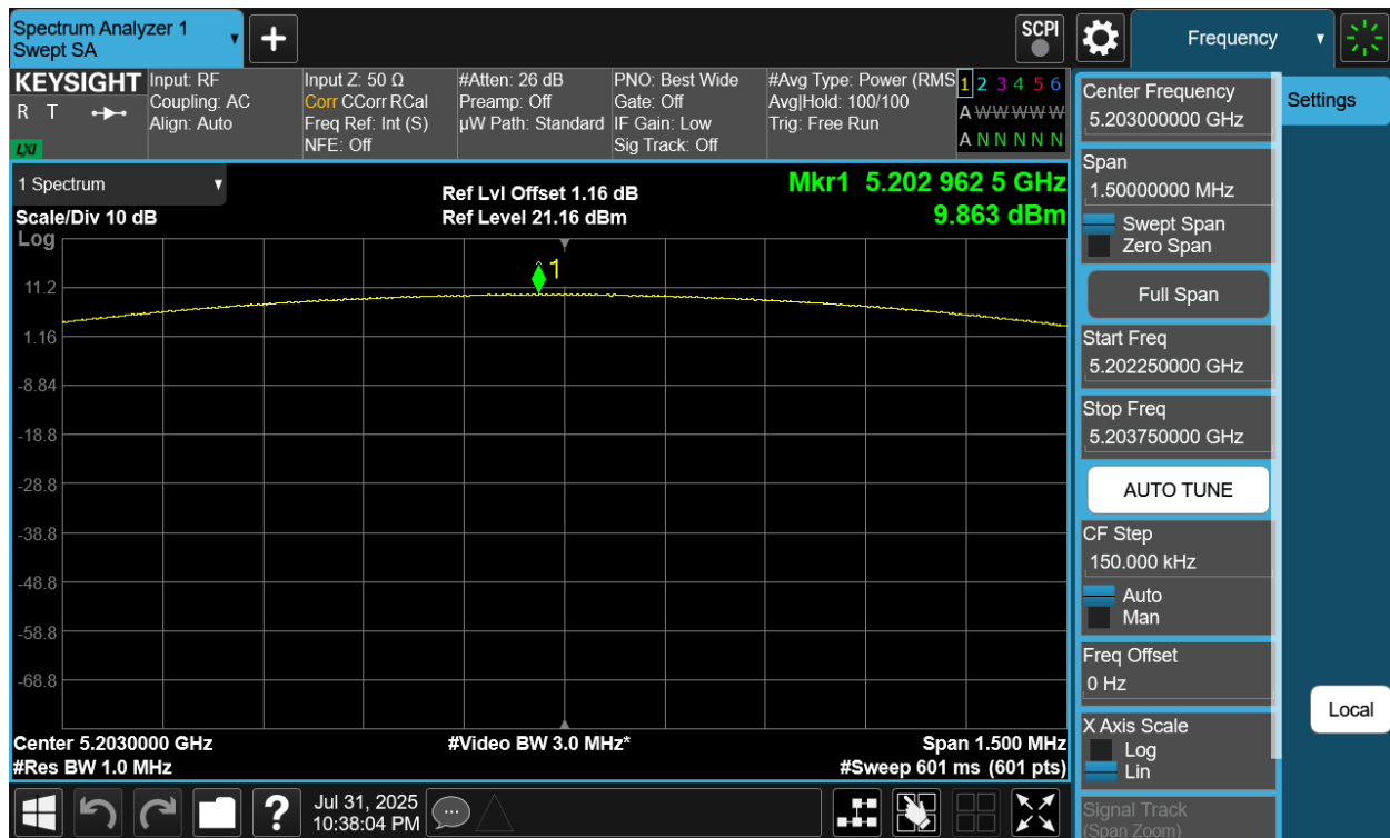
Plot 7-79. PSD Antenna WF5B (NB UNII BDR, ePA – 5203MHz)
