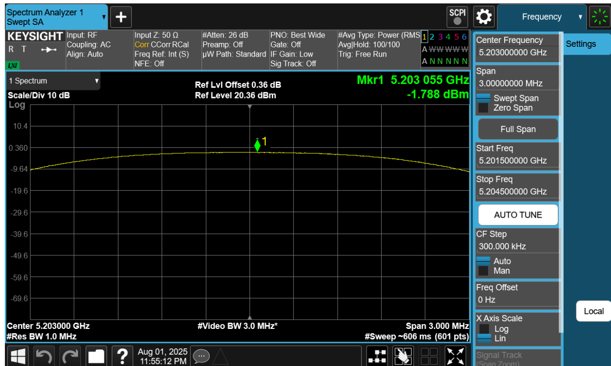
Plot 7-258. PSD TxBF Primary Antenna 4a (NB UNII HDRPS2, iPA – 5203MHz)
