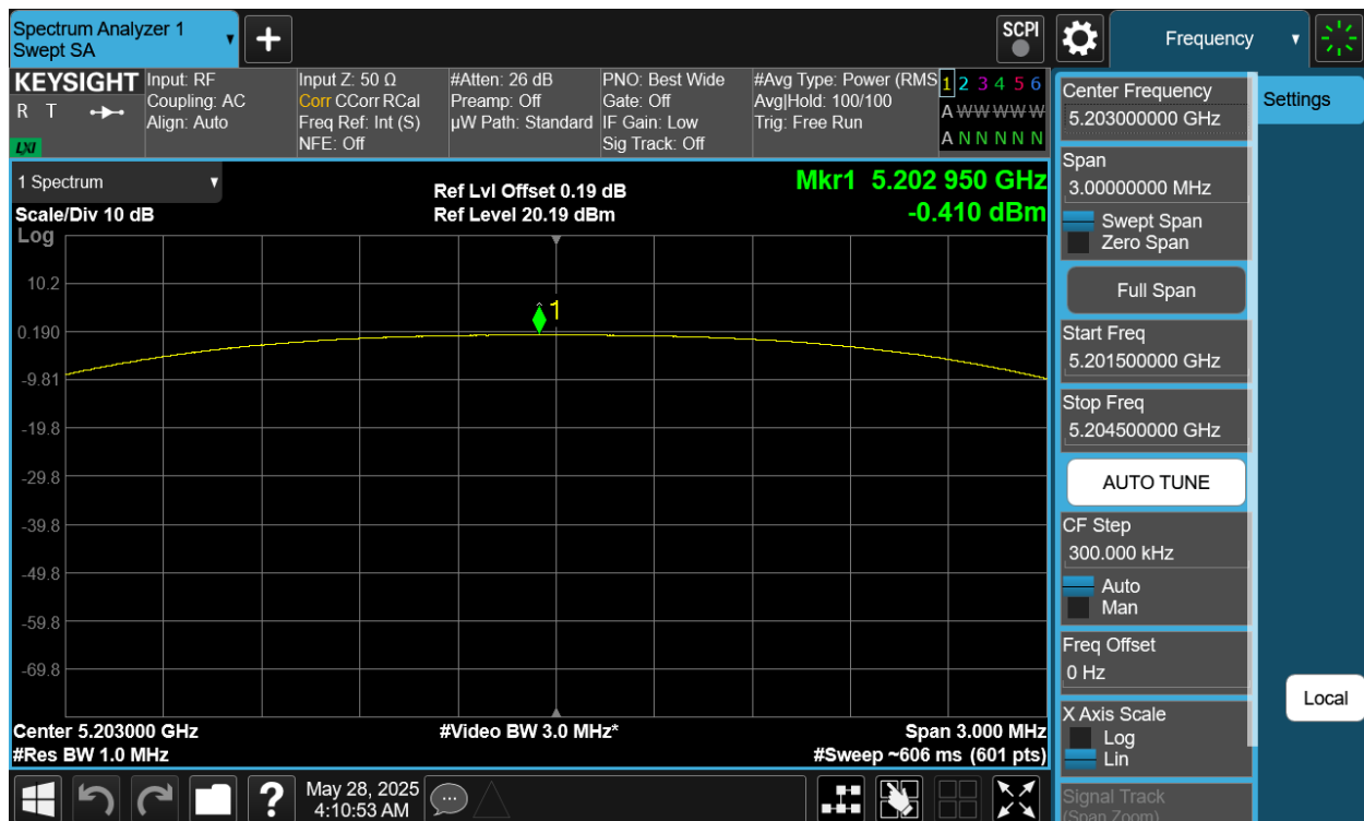
Plot 7-278. PSD TxBF Primary Antenna 4a (NB UNII HDT2, iPA – 5203MHz)
