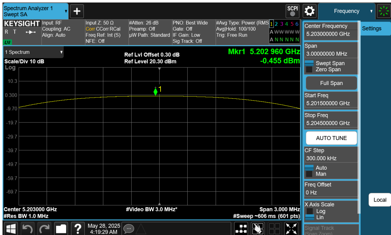
Plot 7-282. PSD TxBF Primary Antenna 4a (NB UNII HDT4, iPA – 5203MHz)
