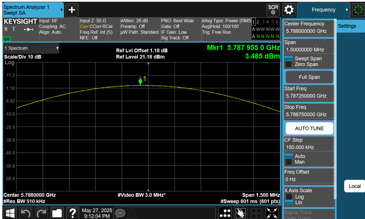
Plot 7-290. PSD TxBF Primary Antenna 4a (NB UNII BDR, iPA – 5788MHz)
