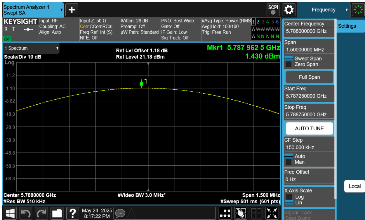
Plot 7-289. PSD TxBF Primary Antenna WF5B (NB UNII BDR, iPA – 5788MHz)
