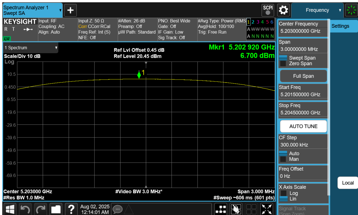
Plot 7-284. PSD TxBF Primary Antenna 4a (NB UNII HDT6, ePA – 5203MHz)
