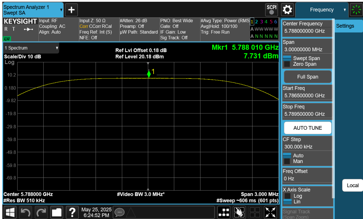
Plot 7-327. PSD Tx BF Primary Antenna WF5B (NB UNII HDT2, ePA – 5788MHz)
