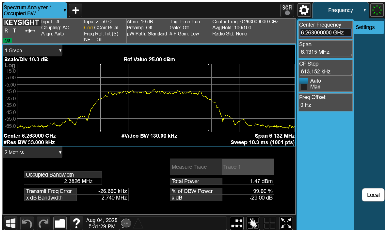
Plot 7-39. 26dB BW & 99% OBW Antenna 2a (NB UNII HDT6, ePA– 6263MHz)
