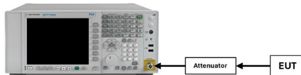
Figure 7-1. Test Instrument & Measurement Setup
