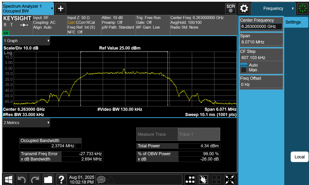
Plot 7-19. 26dB BW & 99% OBW Antenna 4a (NB UNII HDRPS2, ePA- 6263MHz)
