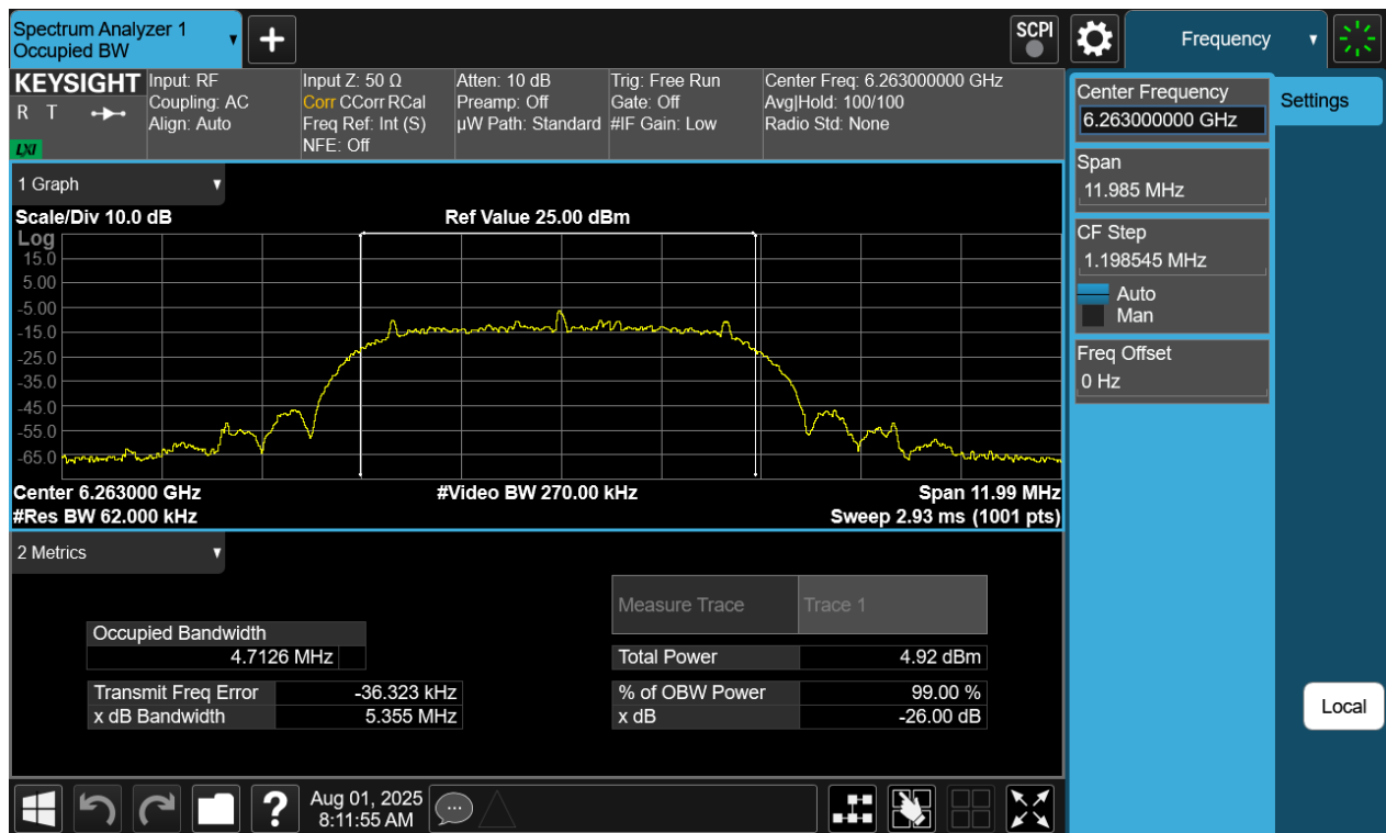
Plot 7-7. 26dB BW & 99% OBW Antenna WF5B (NB UNII XHDRPM6, ePA- 6263MHz)
