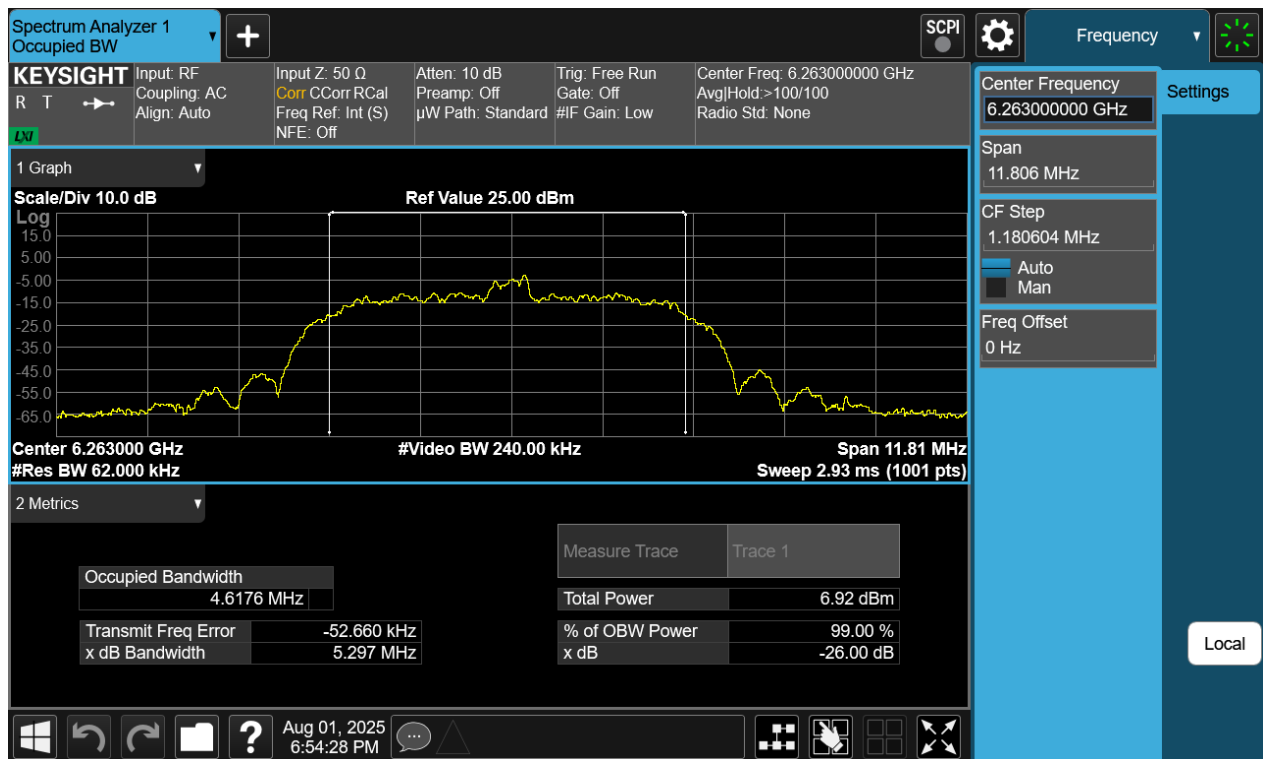
Plot 7-18. 26dB BW & 99% OBW Antenna 4a (NB UNII HDR8, ePA- 6263MHz)
