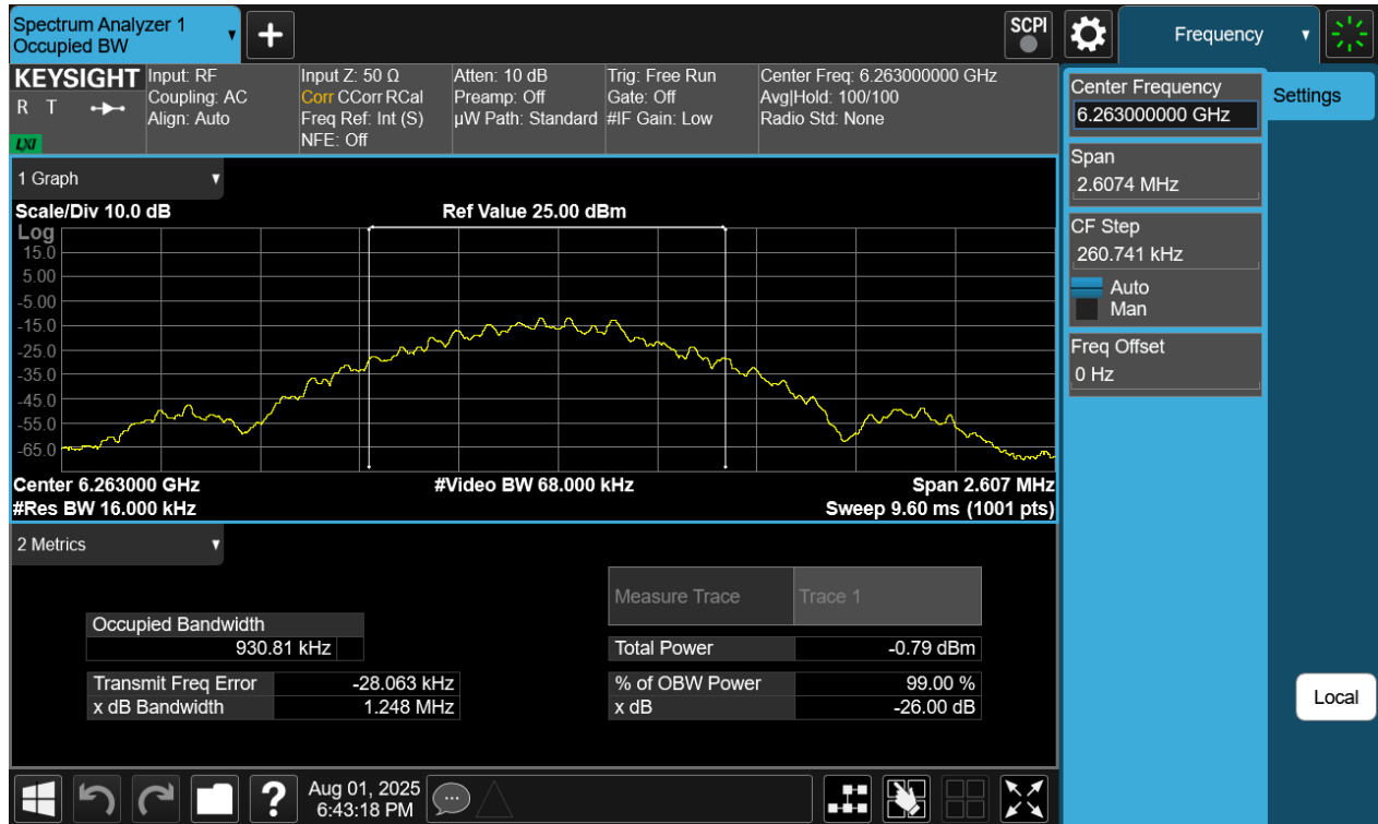
Plot 7-14. 26dB BW & 99% OBW Antenna 4a (NB UNII BDR, ePA- 6263MHz)
