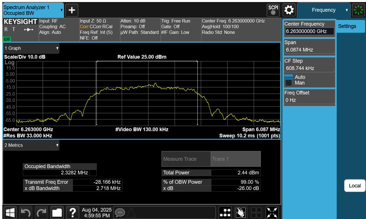
Plot 7-30. 26dB BW & 99% OBW Antenna 2a (NB UNII HDR4, ePA- 6263MHz)
