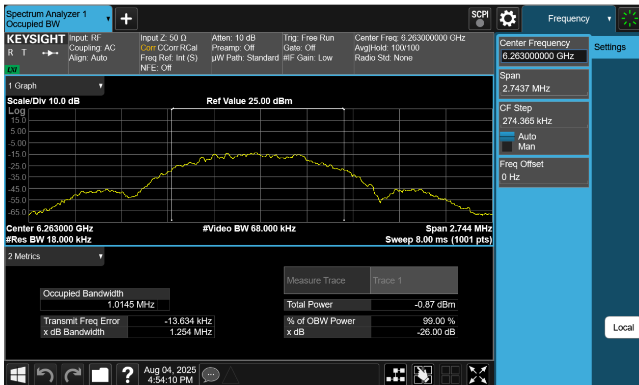
Plot 7-28. 26dB BW & 99% OBW Antenna 2a (NB UNII LE1M, ePA- 6263MHz)
