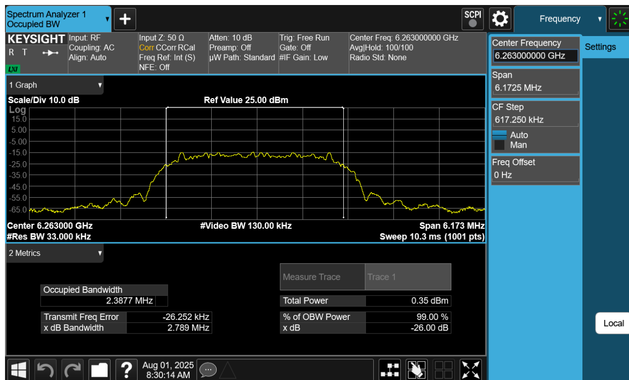
Plot 7-13. 26dB BW & 99% OBW Antenna WF5B (NB UNII HDT6, ePA- 6263MHz)
