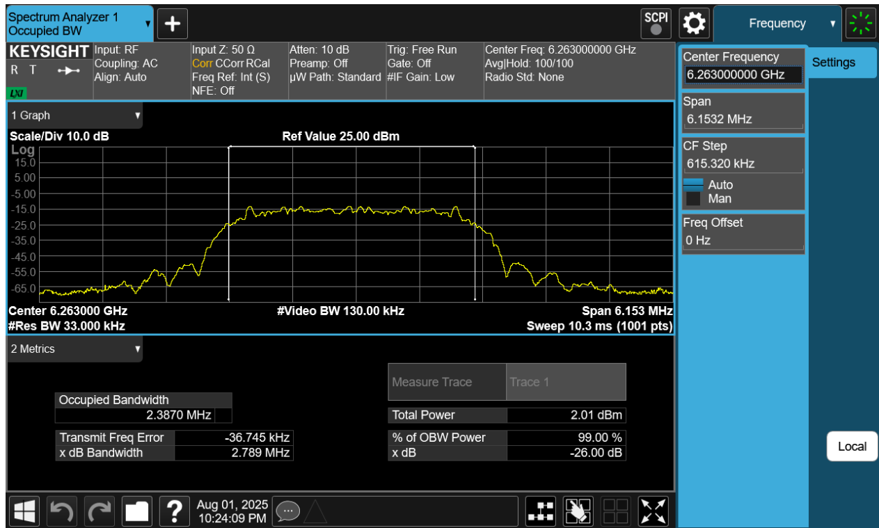
Plot 7-26. 26dB BW & 99% OBW Antenna 4a (NB UNII HDT6, ePA– 6263MHz)
