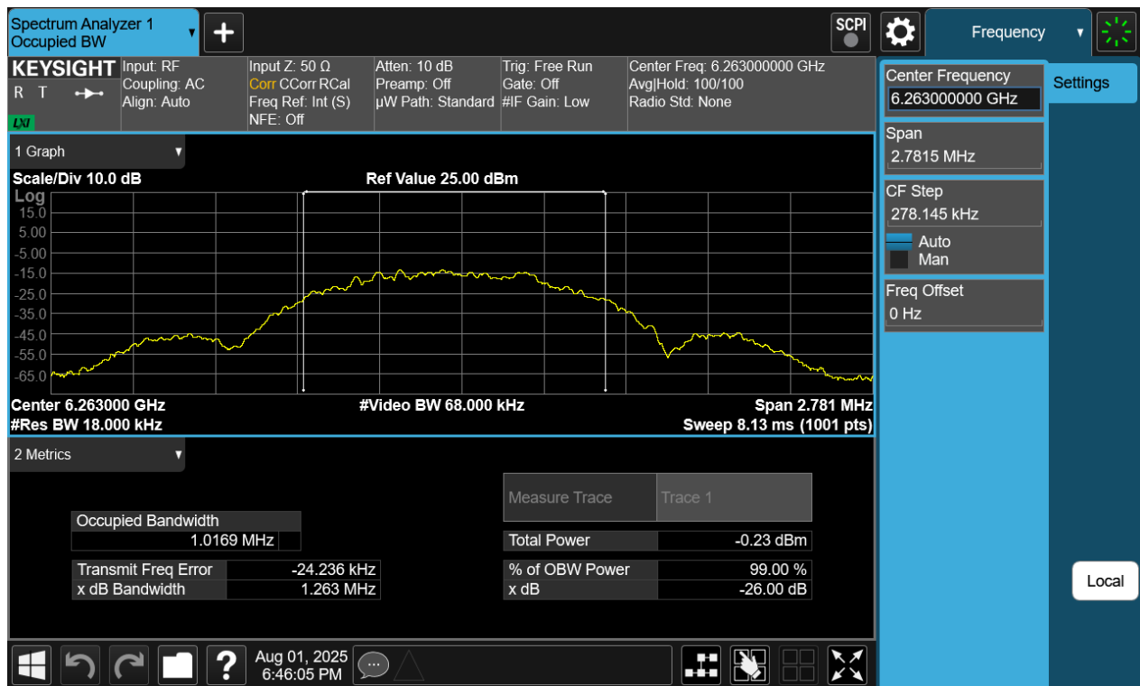
Plot 7-15. 26dB BW & 99% OBW Antenna 4a (NB UNII LE1M, ePA- 6263MHz)
