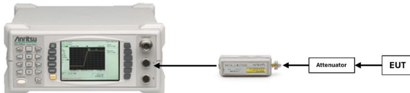
Figure 7-2. Test Instrument & Measurement Setup
