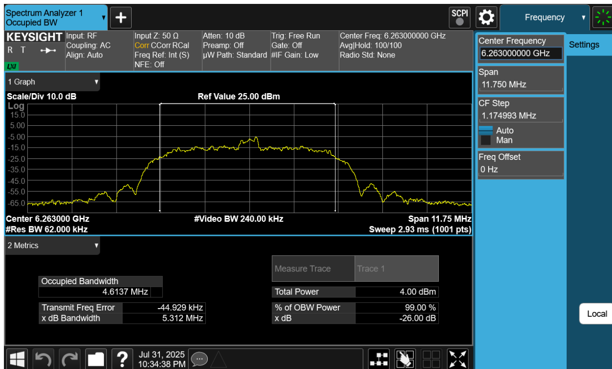
Plot 7-5. 26dB BW & 99% OBW Antenna WF5B (NB UNII HDR8, ePA- 6263MHz)
