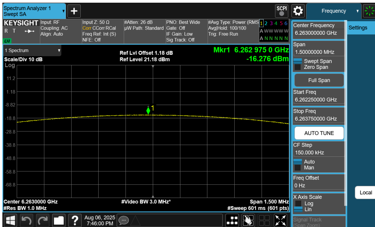
Plot 7-171. PSD TxBF Diversity Antenna 2a (NB UNII BDR, ePA – 6263MHz)
