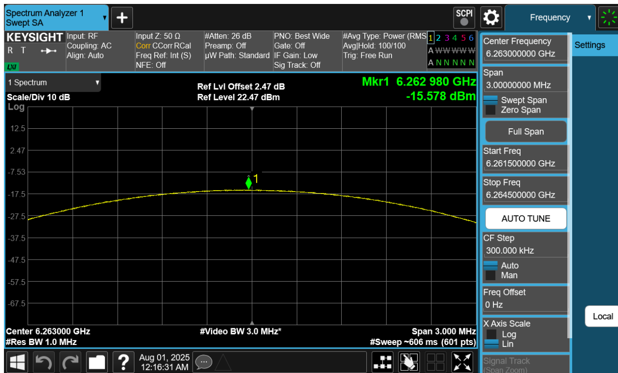
Plot 7-126. PSD TxBF Primary Antenna WF5B (NB UNII LE2M, ePA – 6263MHz)
