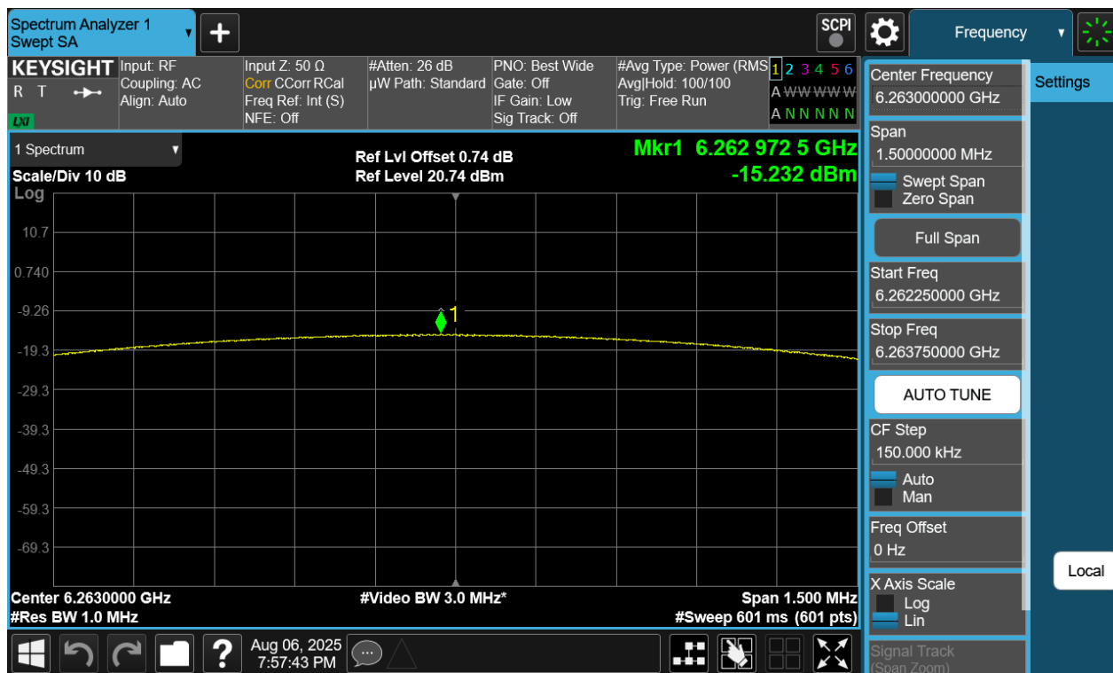
Plot 7-177. PSD Tx BF Diversity Antenna 2a (NB UNII LE1M, iPA – 6263MHz)
