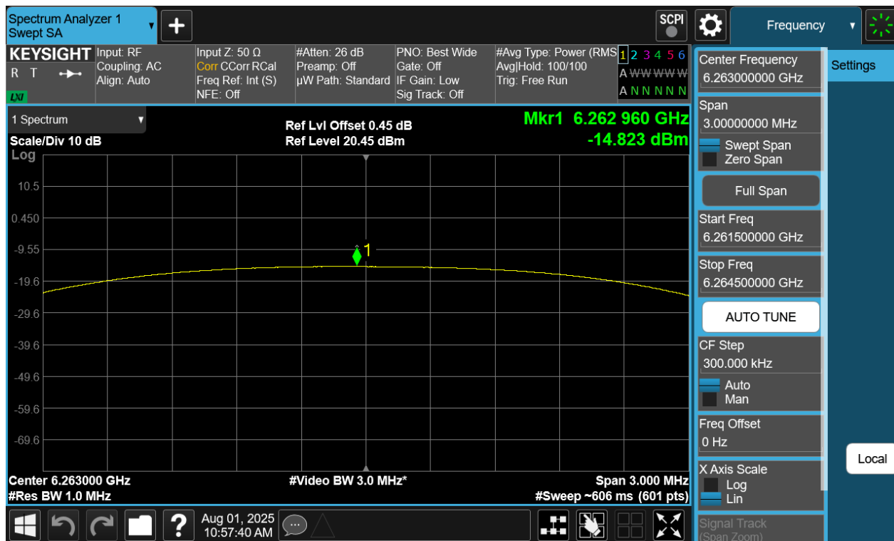
Plot 7-168. PSD TxBF Primary Antenna WF5B (NB UNII HDT6, iPA – 6263MHz)
