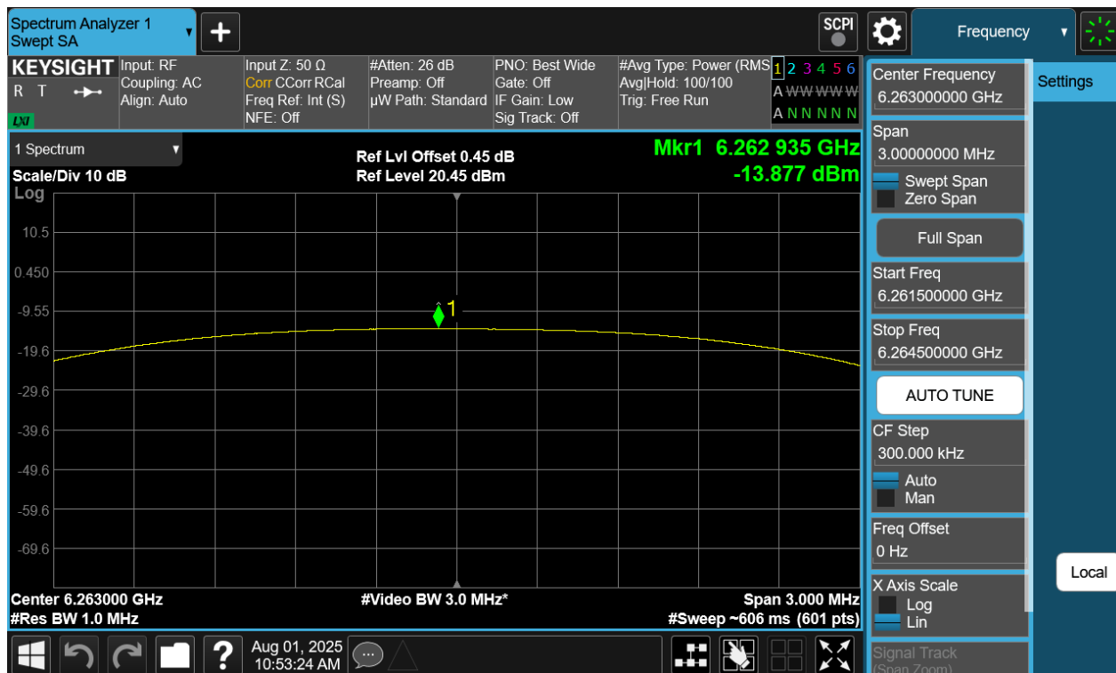
Plot 7-166. PSD TxBF Primary Antenna WF5B (NB UNII HDT6, ePA – 6263MHz)
