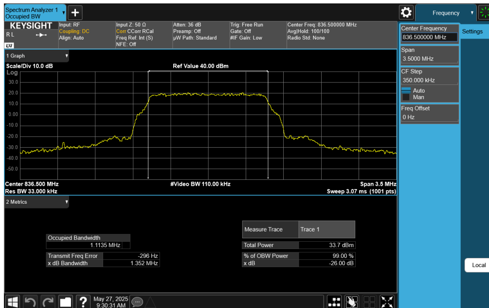
Plot 7-1. Occupied Bandwidth Plot (LTE Band 26/5 - 1.4MHz QPSK - Full RB Configuration)
