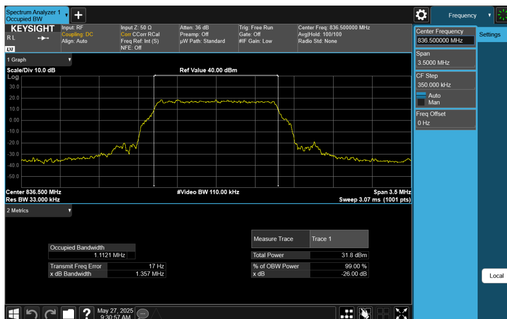
Plot 7-3. Occupied Bandwidth Plot (LTE Band 26/5 - 1.4MHz 64-QAM - Full RB Configuration)
