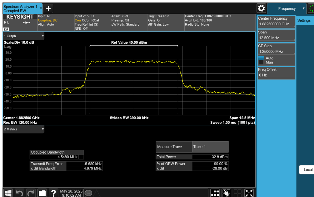
Plot 7-10. Occupied Bandwidth Plot (LTE Band 25/2 - 5MHz 16-QAM - Full RB Configuration)
