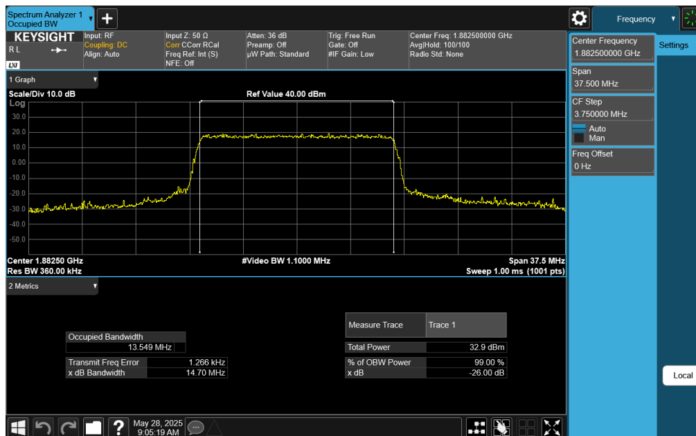
Plot 7-18. Occupied Bandwidth Plot (LTE Band 25/2 - 15MHz 16-QAM - Full RB Configuration)
