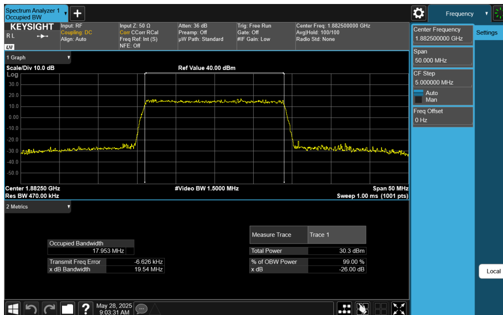
Plot 7-24. Occupied Bandwidth Plot (LTE Band 25/2 - 20MHz 256-QAM - Full RB Configuration)
