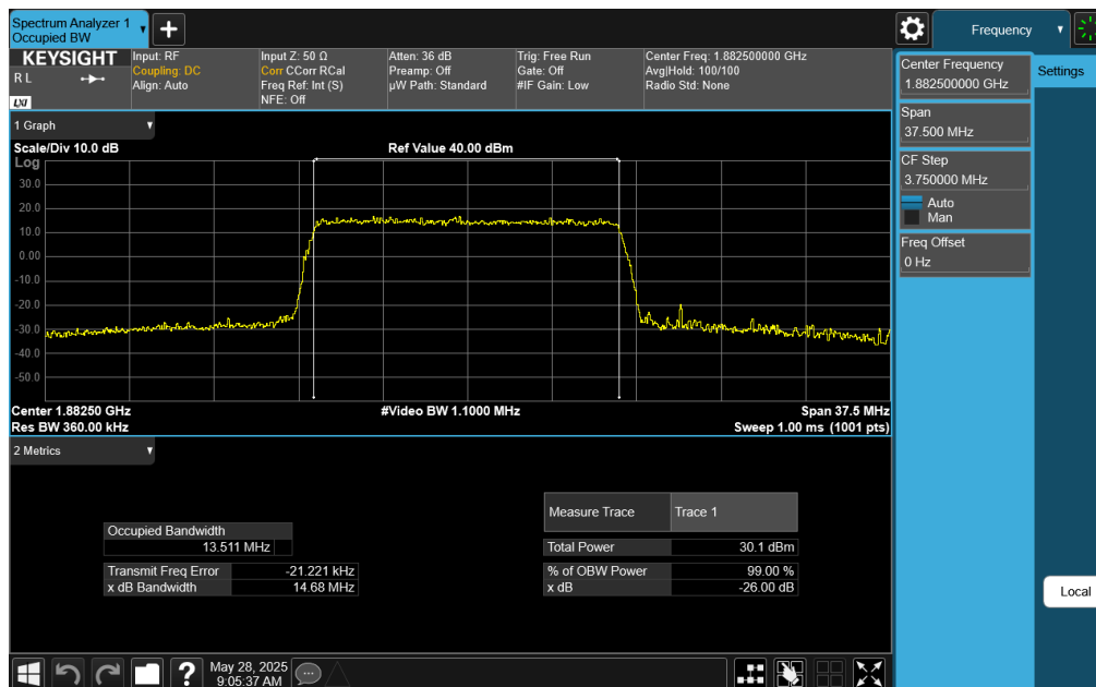
Plot 7-20. Occupied Bandwidth Plot (LTE Band 25/2 - 15MHz 256-QAM - Full RB Configuration)
