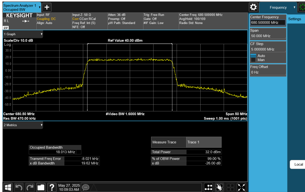
Plot 7-39. Occupied Bandwidth Plot (LTE Band 71 - 20MHz 64-QAM - Full RB)
