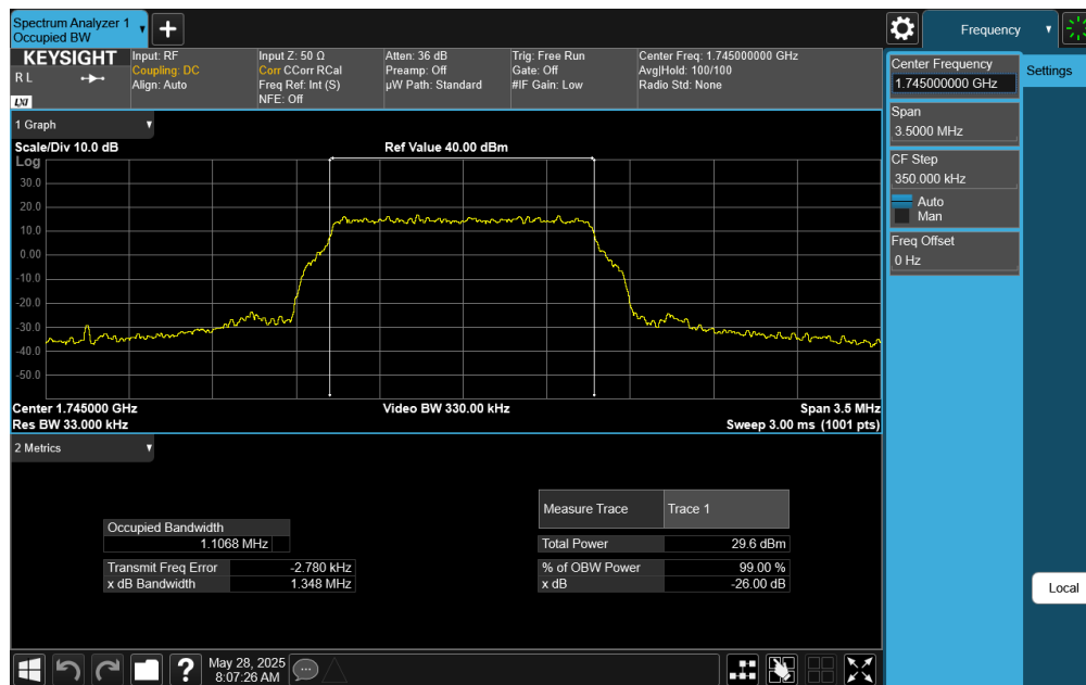
Plot 7-4. Occupied Bandwidth Plot (LTE Band 66/4 - 1.4MHz 256-QAM - Full RB)
