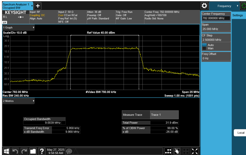
Plot 7-63. Occupied Bandwidth Plot (LTE Band 13 - 10MHz 64-QAM - Full RB)
