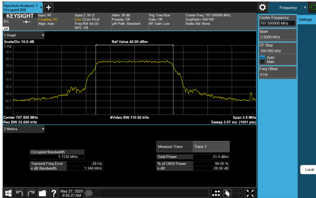
Plot 7-43. Occupied Bandwidth Plot (LTE Band 12 – 1.4MHz 64-QAM - Full RB)
