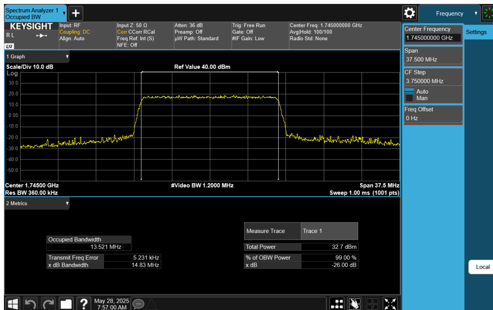
Plot 7-18. Occupied Bandwidth Plot (LTE Band 66/4 - 15MHz 16-QAM - Full RB)
