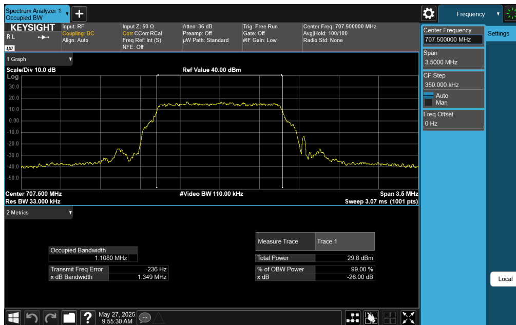
Plot 7-44. Occupied Bandwidth Plot (LTE Band 12 – 1.4MHz 256-QAM - Full RB)
