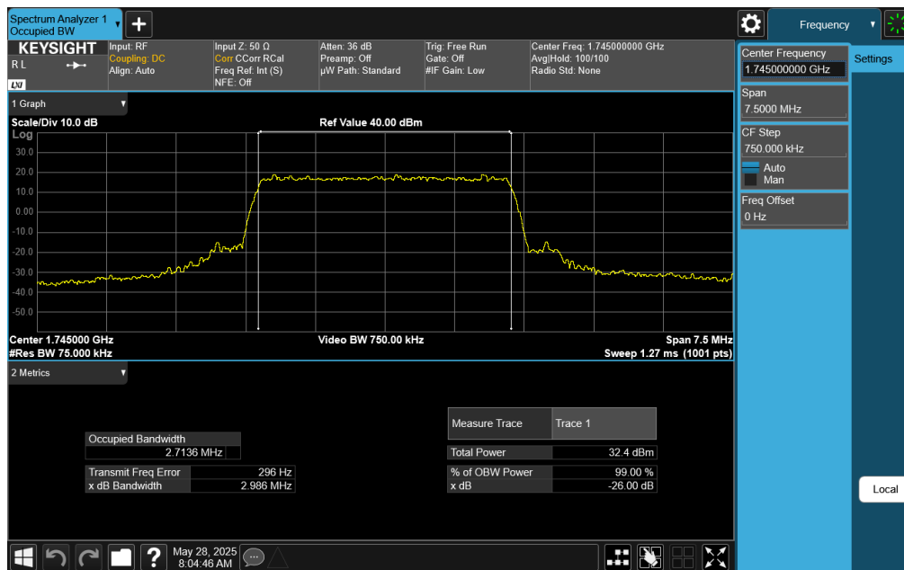
Plot 7-6. Occupied Bandwidth Plot (LTE Band 66/4 - 3MHz 16-QAM - Full RB)
