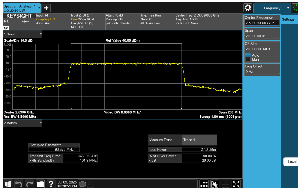
Plot 7-161. Occupied Bandwidth Plot (NR Band n41 - 100MHz DFT-s-OFDM \pi/2 BPSK - Full RB)
