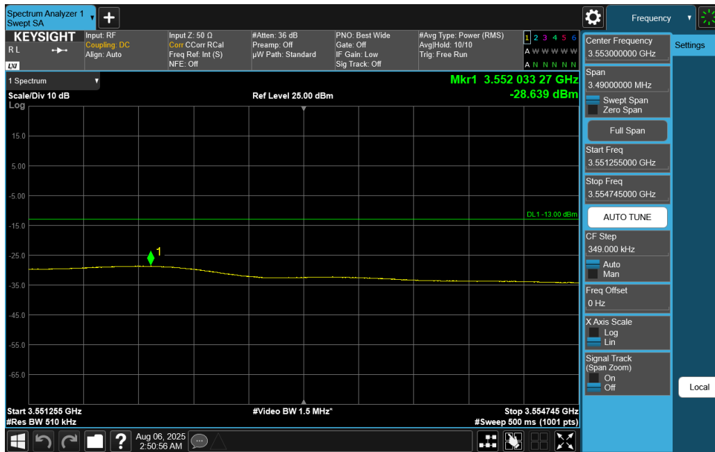
Plot 7-143. Extended Upper Band Edge Plot (NR Band n77 DoD-Band - 10MHz DFT-s-OFDM QPSK – Full RB)
