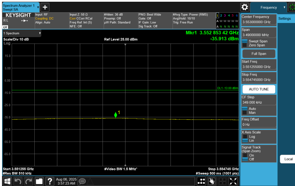
Plot 7-197. Extended Upper Band Edge Plot (NR Band n77 DoD-Band - 80MHz DFT-s-OFDM QPSK – Full RB)
