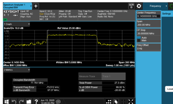
Plot 7-3 26dB BW & 99% OBW Antenna WF5B (80MHz BW 802.11be(SU) - Ch.39)
