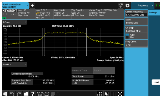
Plot 7-29 26dB BW & 99% OBW Antenna 4a (20MHz BW 802.11a - Ch.45)
