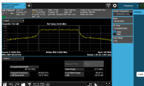
Plot 7-2 26dB BW & 99% OBW Antenna WF5B (40MHz BW 802.11be(SU) - Ch.43)
