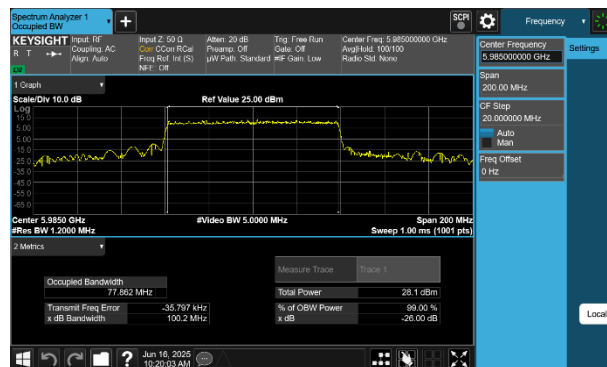
Plot 7-31 26dB BW & 99% OBW Antenna 4a (80MHz BW 802.11be(SU) - Ch.7)
