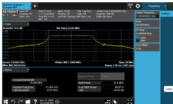
Plot 7-1 26dB BW & 99% OBW Antenna WF5B (20MHz BW 802.11a - Ch.1)
