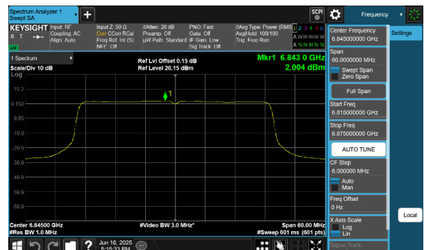
Plot 7-190 PSD CDD Primary Antenna 4a (40MHz BW 802.11be(SU) - Ch.179)
