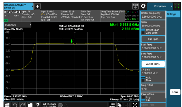
Plot 7-174 PSD CDD Primary Antenna 4a (40MHz BW 802.11be(SU) - Ch.3)
