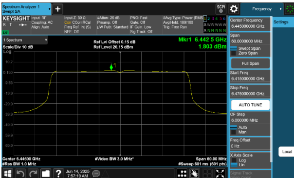
Plot 7-178 PSD CDD Primary Antenna WF5B (40MHz BW 802.11be(SU) - Ch.99)
