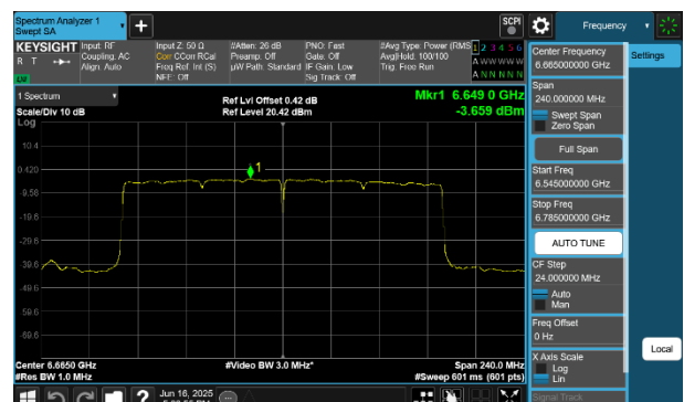
Plot 7-192 PSD CDD Primary Antenna 4a (160MHz BW 802.11be(SU) - Ch.143)
