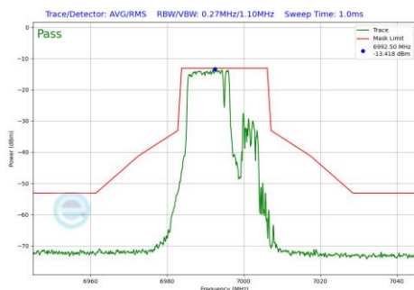
Plot 7-1108 In-Band Emission Plot SDM Primary Antenna WF5B (20MHz BW 802.11be(RU) RU106+26 Index82 (UNII Band 8) - Ch.209)
