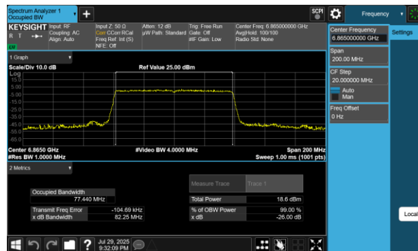
Plot 7-76 26dB BW & 99% OBW Antenna 4a (80MHz BW 802.11be(RU) RU996 Index67 - Ch.183)
