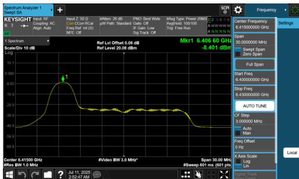
Plot 7-133 PSD Antenna WF5B (20MHz BW 802.11be(RU) RU26 Index0 - Ch.93)
