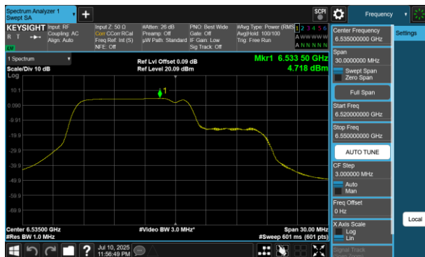
Plot 7-412 PSD Antenna 2a (20MHz BW 802.11be(RU) RU106+26 Index82 - Ch.117)
