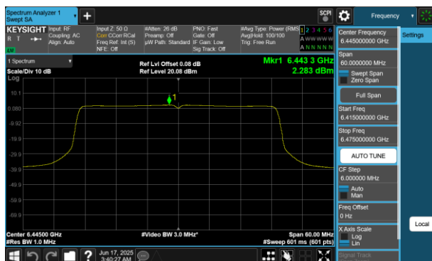
Plot 7-405 PSD Antenna 2a (40MHz BW 802.11be(RU) RU484 Index65 - Ch.99)
