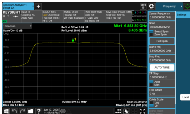
Plot 7-338 PSD Antenna 4a(20MHz BW 802.11be(RU) RU242 Index61 - Ch.181)
