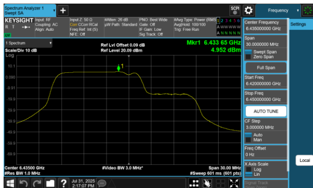
Plot 7-401 PSD Antenna 2a (20MHz BW 802.11be(RU) RU106+26 Index82 - Ch.97)
