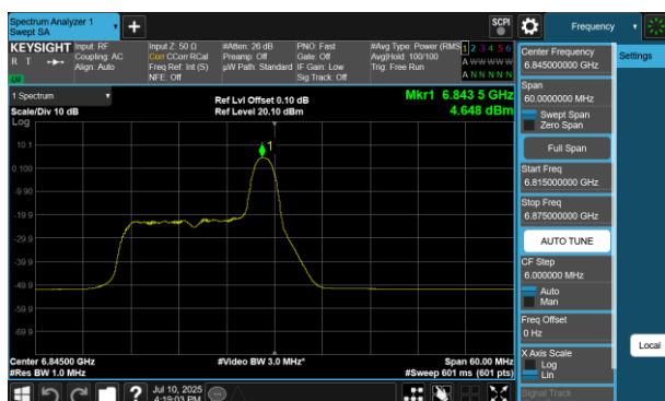
Plot 7-409 PSD Antenna 2a (40MHz BW 802.11be(RU) RU26 Index8 - Ch.179)
