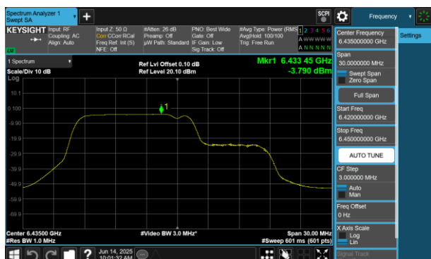
Plot 7-357 PSD Antenna 4a(20MHz BW 802.11be(RU) RU106+26 Index82 - Ch.97)
