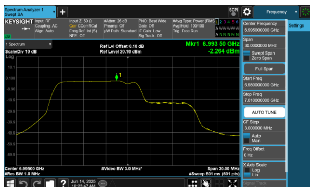
Plot 7-379 PSD Antenna 4a(20MHz BW 802.11be(RU) RU106+26 Index82 - Ch.209)
