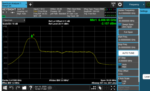
Plot 7-342 PSD Antenna 4a(20MHz BW 802.11be(RU) RU26 Index0 - Ch.93)
