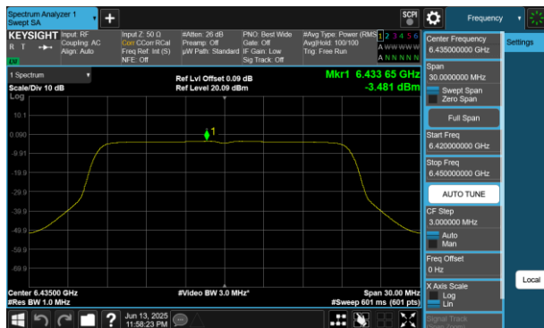
Plot 7-360 PSD Antenna 4a(20MHz BW 802.11be(RU) RU242 Index61 - Ch.97)
