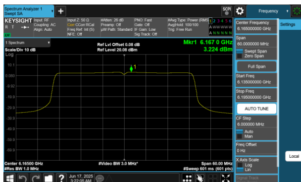
Plot 7-394 PSD Antenna 2a (40MHz BW 802.11be(RU) RU484 Index65 - Ch.43)
