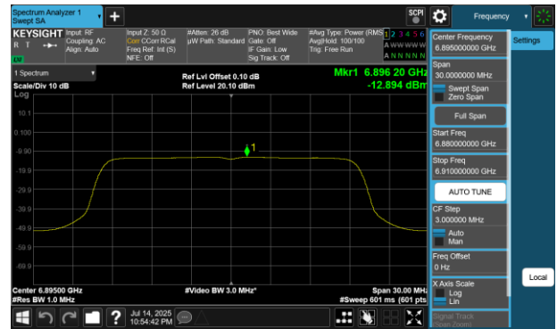
Plot 7-437 PSD SDM Diversity Antenna 2a (20MHz BW 802.11be(RU) RU242 Index61 - Ch.189)
