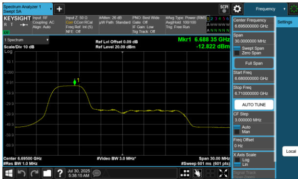
Plot 7-397 PSD SDM Diversity Antenna 4a (20MHz BW 802.11be(RU) RU52 Index37 - Ch.149)
