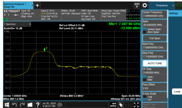
Plot 7-423 PSD SDM Diversity Antenna 2a (20MHz BW 802.11be(RU) RU52 Index37 - Ch.229)
