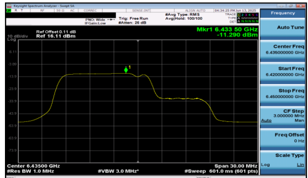
Plot 7-386 PSD SDM Diversity Antenna 2a (20MHz BW 802.11be(RU) RU106+26 Index82 - Ch.97)
