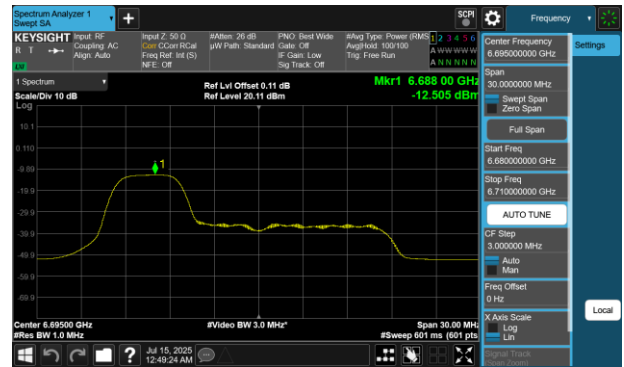
Plot 7-401 PSD SDM Diversity Antenna 2a (20MHz BW 802.11be(RU) RU52 Index37 - Ch.149)
