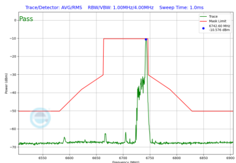
Plot 7-451 In-Band Emission Plot Antenna WF5B (80MHz BW 802.11be(RU) RU26 Index36 (UNII Band 7) - Ch.151)
