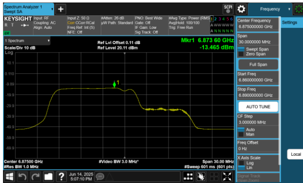
Plot 7-405 PSD SDM Diversity Antenna 4a(20MHz BW 802.11be(RU) RU106+26 Index82 - Ch.185)
