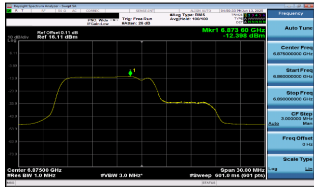
Plot 7-408 PSD SDM Diversity Antenna 2a (20MHz BW 802.11be(RU) RU106+26 Index82 - Ch.185)
