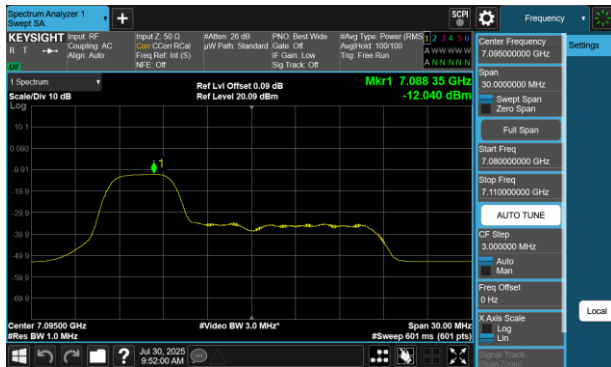
Plot 7-419 PSD SDM Diversity Antenna 4a (20MHz BW 802.11be(RU) RU52 Index37 - Ch.229)
