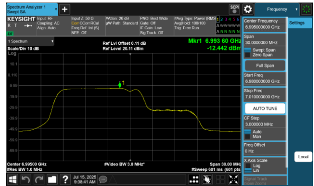
Plot 7-430 PSD SDM Diversity Antenna 2a (20MHz BW 802.11be(RU) RU106+26 Index82 - Ch.209)
