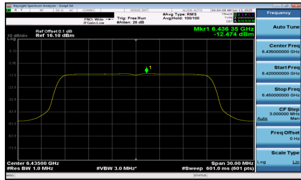
Plot 7-393 PSD SDM Diversity Antenna 2a (20MHz BW 802.11be(RU) RU242 Index61 - Ch.97)
