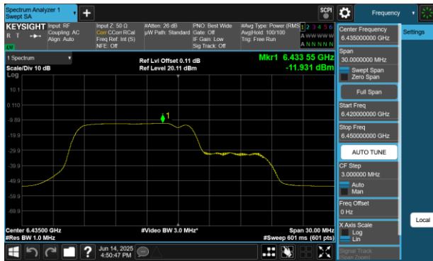
Plot 7-383 PSD SDM Diversity Antenna 4a(20MHz BW 802.11be(RU) RU106+26 Index82 - Ch.97)
