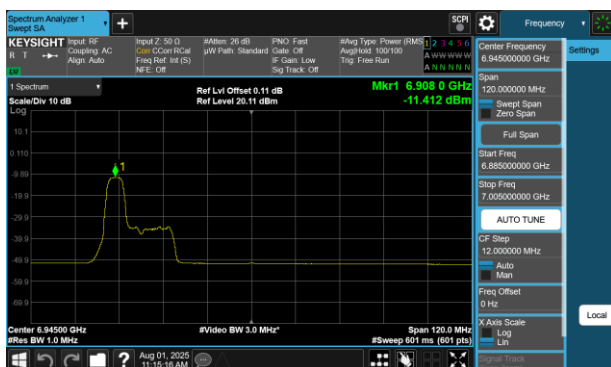
Plot 7-421 PSD SDM Diversity Antenna 4a (80MHz BW 802.11be(RU) RU52 Index37 - Ch.199)
