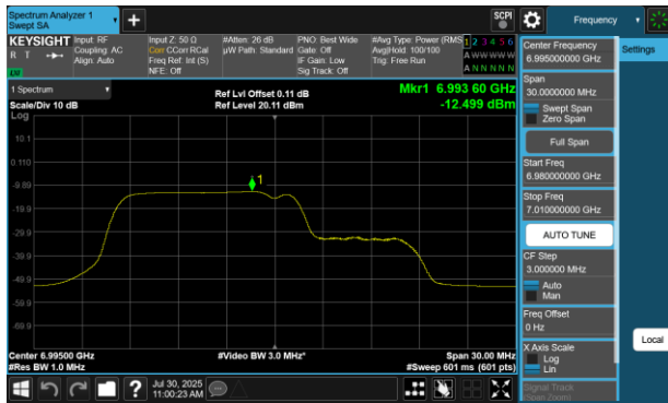
Plot 7-427 PSD SDM Diversity Antenna 4a(20MHz BW 802.11be(RU) RU106+26 Index82 - Ch.209)
