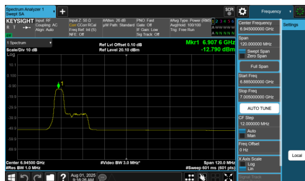
Plot 7-425 PSD SDM Diversity Antenna 2a (80MHz BW 802.11be(RU) RU52 Index37 - Ch.199)
