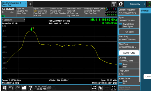
Plot 7-617 PSD CDD Diversity Antenna 4a(20MHz BW 802.11be(RU) RU26 Index0 - Ch.45)
