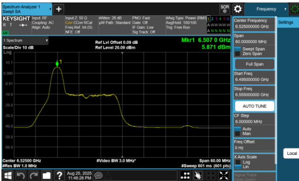
Plot 7-640 PSD CDD Diversity Antenna 4a(40MHz BW 802.11be(RU) RU26 Index0 - Ch.115)
