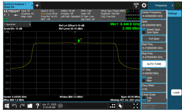
Plot 7-658 PSD CDD Diversity Antenna 2a (40MHz BW 802.11be(RU) RU484 Index65 - Ch.99)
