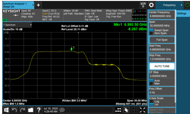
Plot 7-603 PSD SDM Primary Antenna WF5B (20MHz BW 802.11be(RU) RU106+26 Index82 - Ch.209)
