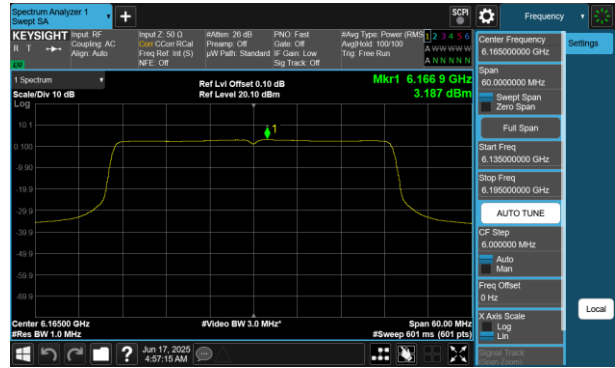
Plot 7-636 PSD CDD Diversity Antenna 2a (40MHz BW 802.11be(RU) RU484 Index65 - Ch.43)
