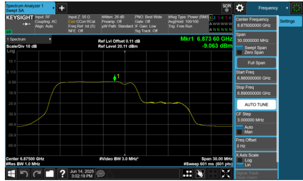
Plot 7-584 PSD SDM Primary Antenna 4a(20MHz BW 802.11be(RU) RU106+26 Index82 - Ch.185)
