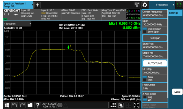
Plot 7-606 PSD SDM Primary Antenna 4a(20MHz BW 802.11be(RU) RU106+26 Index82 - Ch.209)
