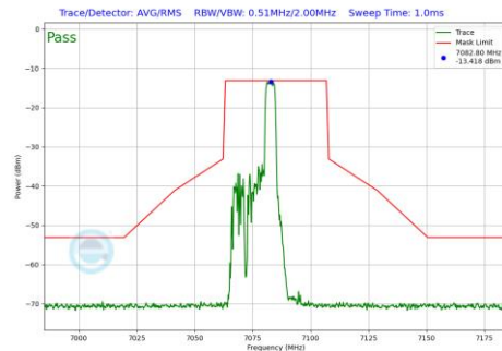
Plot 7-690 In-Band Emission Plot SDM Diversity Antenna 4a (40MHz BW 802.11be(RU) RU52 Index40 (UNII Band 8) - Ch.227)
