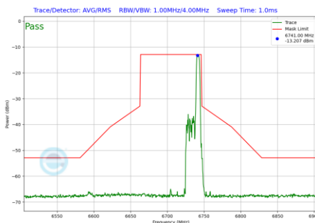
Plot 7-671 In-Band Emission Plot SDM Diversity Antenna 2a (80MHz BW 802.11be(RU) RU52 Index52 (UNII Band 7) - Ch.151)
