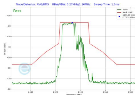
Plot 7-708 In-Band Emission Plot SDM Diversity Antenna 4a (20MHz BW 802.11be(RU) RU106+26 Index82 (UNII Band 6) - Ch.97)
