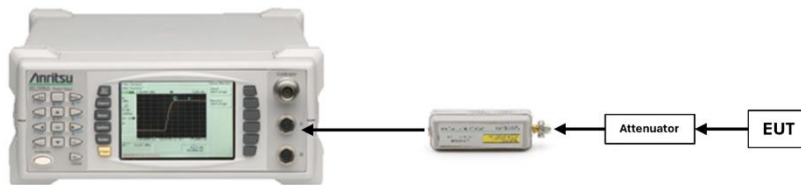
Figure 7-3. Test Instrument & Measurement Setup
