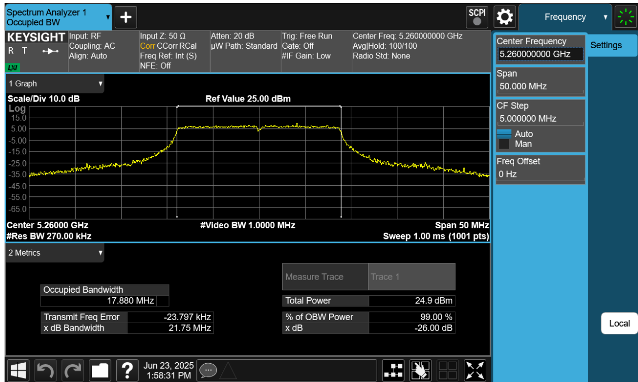
Plot 7-9 26dB BW & 99% OBW Antenna 2a (20MHz BW 802.11n - Ch.52)
